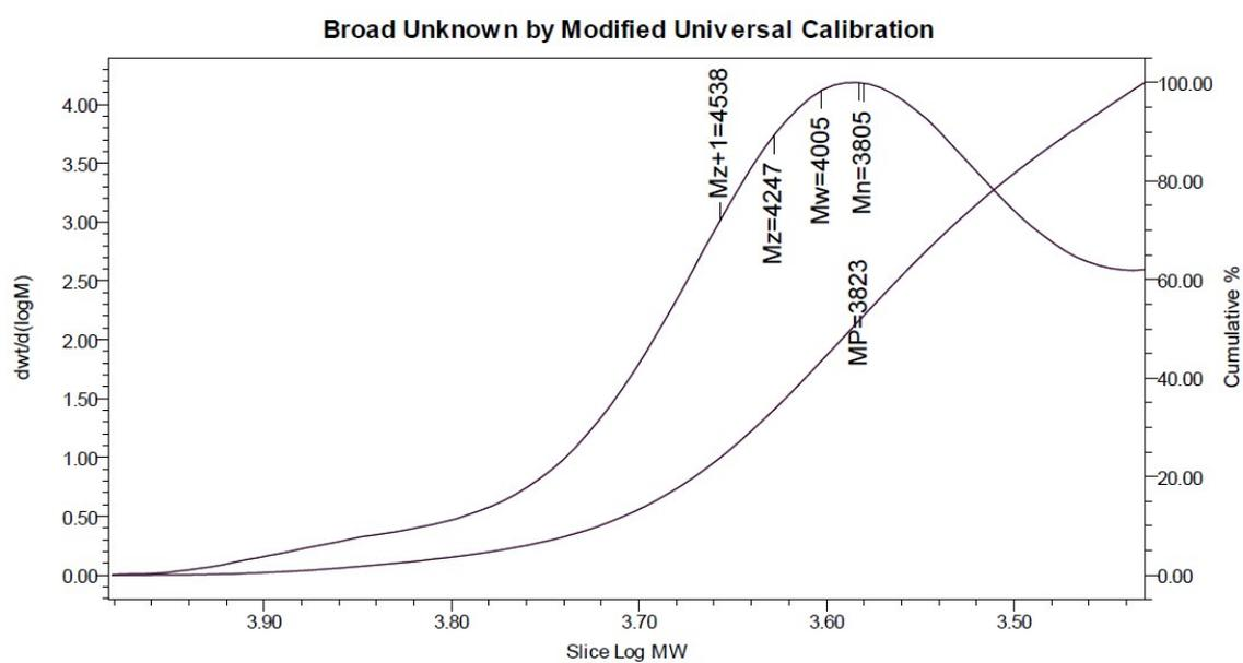
**Figure S24.** Gel permeation chromatography profile of **6**.
