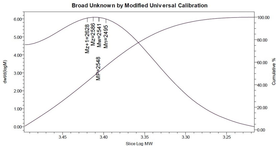
**Figure S25.** Gel permeation chromatography profile of **22**.
