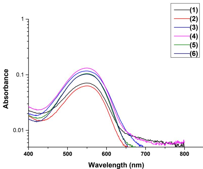
**Figure S26.** UV Absorbance spectra of Nile red in methanol.
