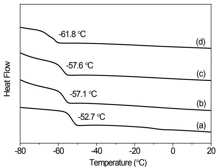
Figure S4 DSC curves of (a) the ethylene/propylene copolymer (Run 1 in Table 1) and the ethylene/propylene/FO copolymer with FO insertion ratio of (b) 2.25 mol%, (c) 4.59 mol% and (d) 9.79 mol% (Runs 2-4 in Table 1) with the feeding ratio of E/P = 1 in gas
