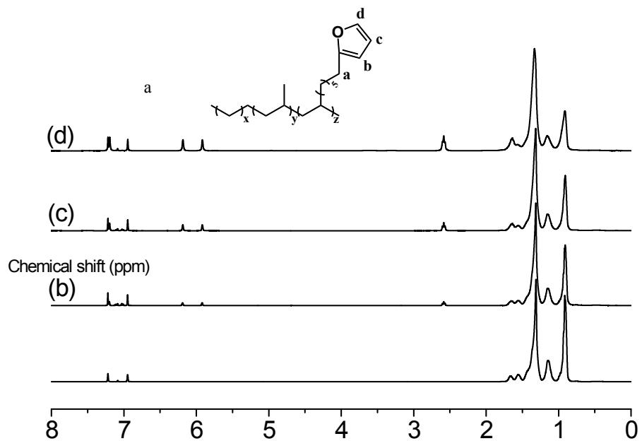
Figure S2 <sup>1</sup>H-NMR spectra of (a) the ethylene/propylene copolymer (Run 1 in Table 1) and the ethylene/propylene/FO copolymer with FO insertion ratio of (b) 2.25 mol%, (c) 4.59 mol% and (d) 9.79 mol% (Runs 2-4 in Table 1) (solvent: 1,2-dichlorobenzene-*d*<sub>4</sub>)
