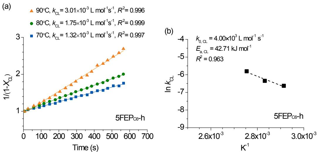
Figure S8 Specimen 5FEP<sub>c6-h</sub>: (a) fitting the initial stage (first 10 min) of the cross-linking conversion data to second order reaction kinetics to determine  $k_{\text{CL}}$  at  $70^\circ\text{C}$ ,  $80^\circ\text{C}$  and  $90^\circ\text{C}$ ; (b) Arrhenius plots to determine the  $k_{0,\text{CL}}$  and  $E_{a,\text{CL}}$  of the cross-linking reaction
