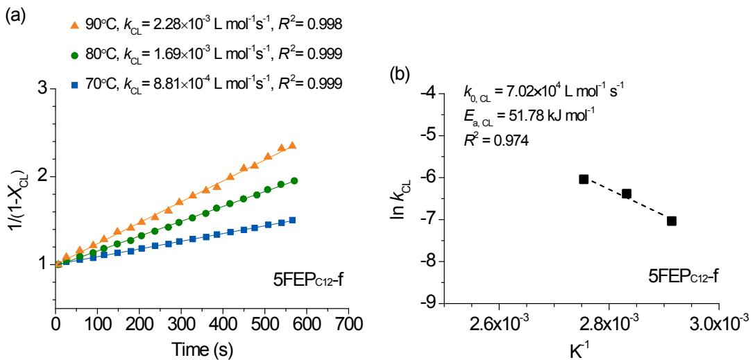
Figure S6 Specimen 5FEP<sub>C12-f</sub>: (a) fitting the initial stage (first 10 min) of the cross-linking conversion data to second order reaction kinetics to determine  $k_{\text{CL}}$  at 70°C, 80°C and 90°C; (b) Arrhenius plots to determine the  $k_{0,\text{CL}}$  and  $E_{a,\text{CL}}$  of the cross-linking reaction
