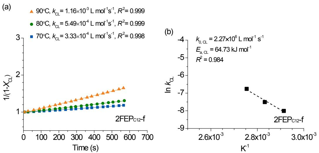
Figure S5 Specimen 2FEP<sub>C12-f</sub>: (a) fitting the initial stage (first 10 min) of the cross-linking conversion data to second order reaction kinetics to determine  $k_{\text{CL}}$  at 70°C, 80°C and 90°C; (b) Arrhenius plots to determine the  $k_{0,\text{CL}}$  and  $E_{a,\text{CL}}$  of the cross-linking reaction
