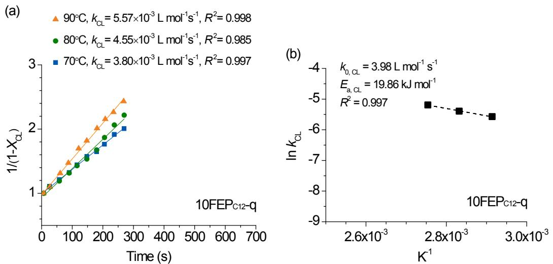
Figure S10 Specimen 10FEP<sub>C12-q</sub>: (a) fitting the initial stage (first 10 min) of the cross-linking conversion data to second order reaction kinetics to determine  $k_{\text{CL}}$  at 70°C, 80°C and 90°C; (b) Arrhenius plots to determine the  $k_{0,\text{CL}}$  and  $E_{a,\text{CL}}$  of the cross-linking reaction
