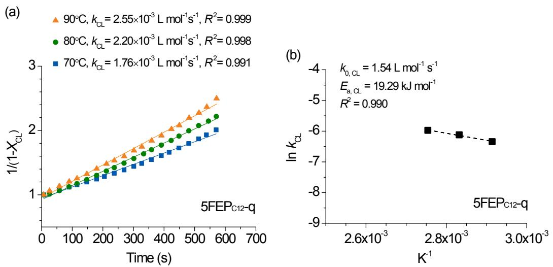
Figure S9 Specimen 5FEP<sub>C12-q</sub>: (a) fitting the initial stage (first 10 min) of the cross-linking conversion data to second order reaction kinetics to determine  $k_{\text{CL}}$  at 70°C, 80°C and 90°C; (b) Arrhenius plots to determine the  $k_{0,\text{CL}}$  and  $E_{a,\text{CL}}$  of the cross-linking reaction
