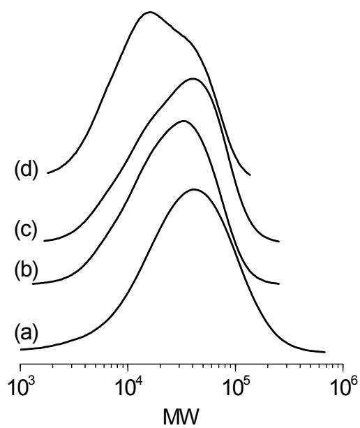
Figure S3 GPC curves of (a) the ethylene/propylene copolymer (Run 1 in Table 1) and the ethylene/propylene/FO copolymer with FO insertion ratio of (b) 2.25 mol%, (c) 4.59 mol% and (d) 9.79 mol% (Runs 2-4 in Table 1)
