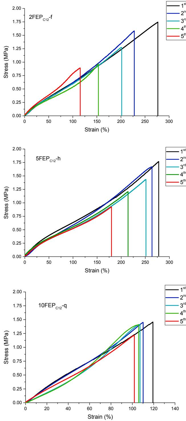
Figure S11 Stress-strain curves of the thermoreversibly cross-linked EPR under five repeated processing cycles
