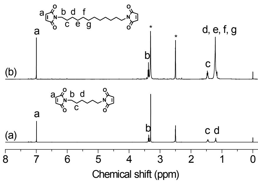
Figure S1 <sup>1</sup>H NMR spectra of (a) 1,6-dimaleimide hexane (C6) and (b) 1,12-bismaleimide dodecane (C12) (solvent: DMSO-*d*<sub>6</sub>)
