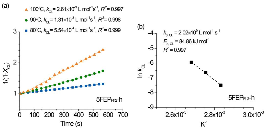
Figure S7 Specimen 5FEP<sub>Ph2-h</sub>: (a) fitting the initial stage (first 10 min) of the cross-linking conversion data to second order reaction kinetics to determine  $k_{\text{CL}}$  at  $80^\circ\text{C}$ ,  $90^\circ\text{C}$  and  $100^\circ\text{C}$ ; (b) Arrhenius plots to determine the  $k_{0,\text{CL}}$  and  $E_{a,\text{CL}}$  of the cross-linking reaction
