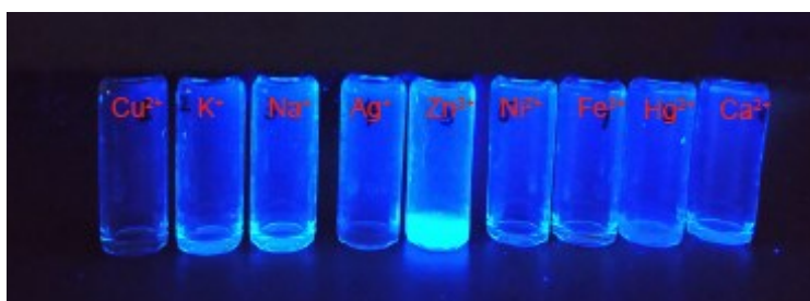
Fig. S4 Visual color change of the solution of molecule PAN-1 observed with addition of different metal ions under UV light ( \lambda = 365 nm).
