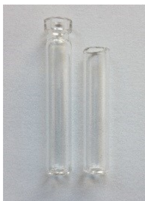
Figure S7 : Left: uncrimped vial; right: vial after removal of the headspace section.
