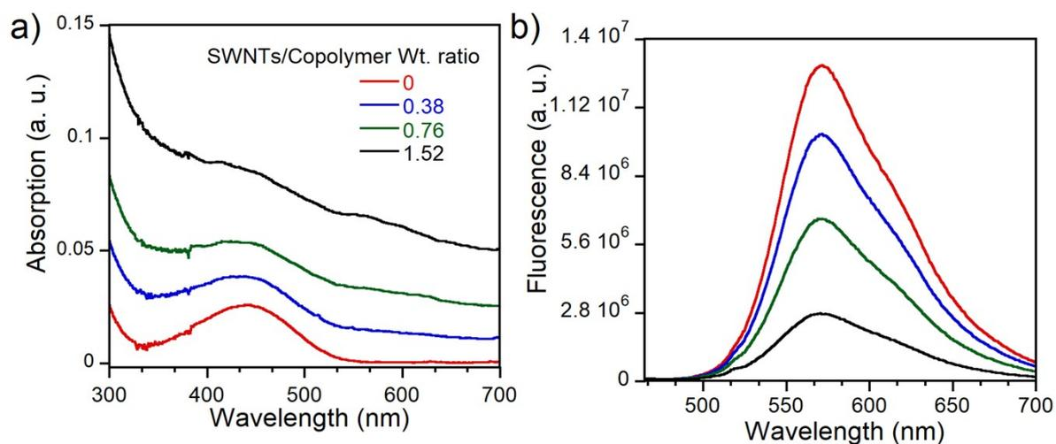
**Figure S6:** Evolution of the (a) optical absorption and (b) photoluminescence spectra of SWNT/PHTcoAHT 36000 suspensions as a function of wt. ratio for a diluted copolymer solution.
