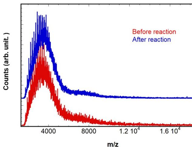
**Figure S9:** MALDI-TOF MS spectra of PHTcoAHT 5000 (red) and of the same polymer after 12 h at 60 °C with *isoamyl nitrite* in THF (blue).
