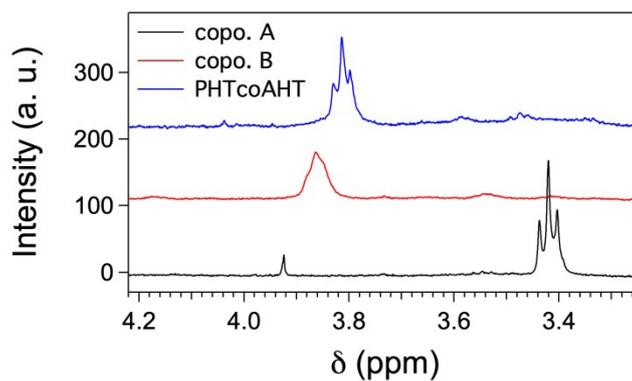
**Figure S4.** Comparison of the NMR spectra of copolymers A, B and **PHTcoAHT** ( $M_n = 36000$ ) between 3.2 and 4.3 ppm.
