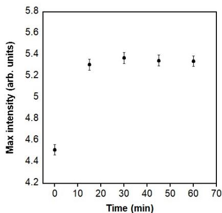
**Figure S8:** Evolution of the fluorescence intensity measured at the maximum of emission (568 nm) of SWNT/PHTcoAHT 36000 at 60°C. The first measurement corresponds to the fluorescence at room temperature.
