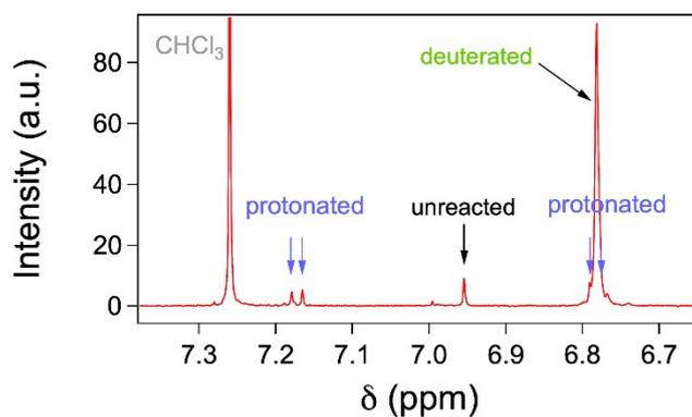
**Figure S1.** NMR analysis of the mixtures of monomers. The monomers are metallated with *i*-PrMgCl. The observed aliquot has been hydrolysed by CD<sub>3</sub>OD.
