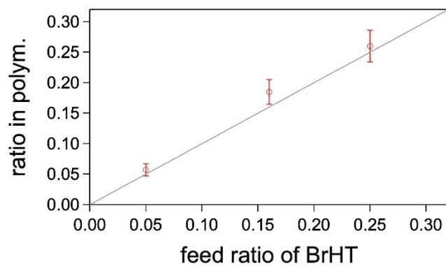
**Figure S3.** Molar fraction of monomer 2 in the polymer vs molar fraction of the monomer 2 in the feed.
