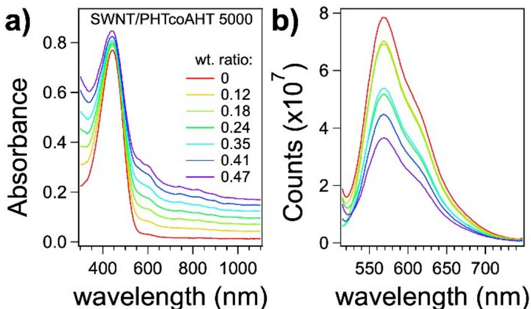
**Figure S5:** Evolution of the optical absorption (a) and fluorescence spectra (b) of SWNT/PHTcoAHT 5000 suspensions as a function of wt. ratio.
