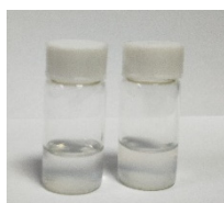
Fig. S1 SEW-2 formed precipitates in the THF/methanol mixture solvents with methanol contents of 50 vol % (left) and 90 vol % (right) at the bottom of the vials.
