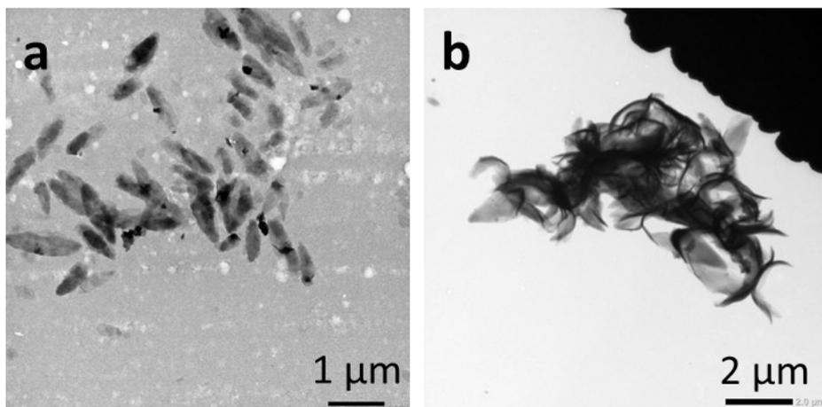
**Figure S13.** TEM images of self-assembled 2D lenticular morphologies prepared from (a) PNIPAM<sub>35</sub>-*b*-PVDF<sub>150</sub> and (b) PNIPAM<sub>35</sub>-*b*-PVDF<sub>450</sub> via micellization in acetone : water mixture after acetone removal by rotary evaporation at room temperature.
