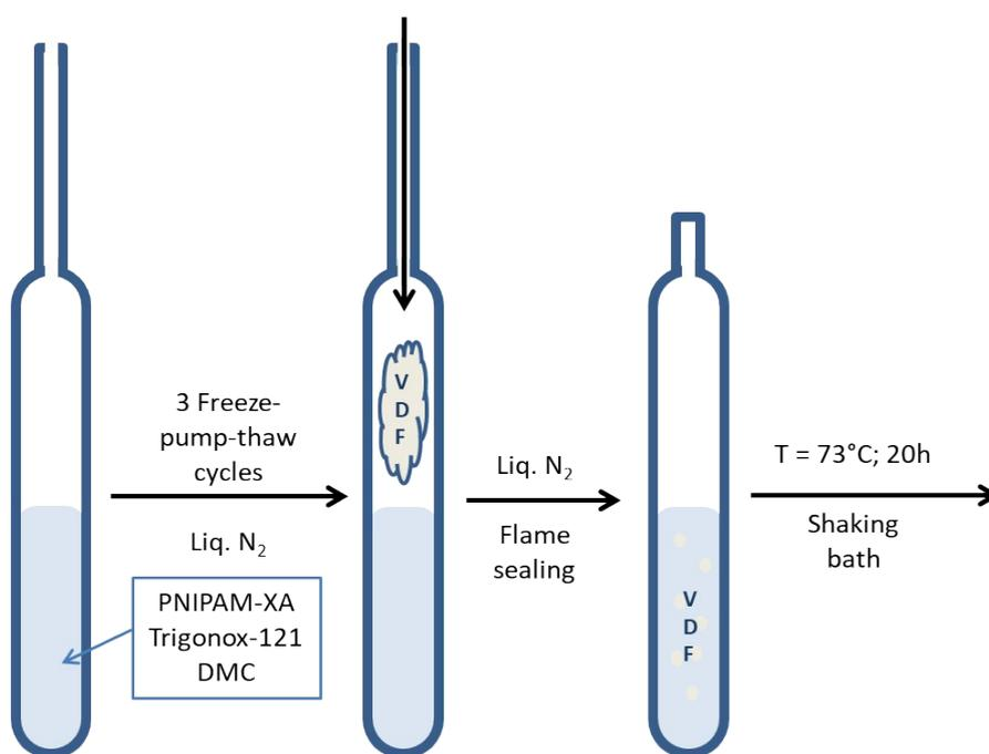
**Scheme S1.** Schematic representation of the synthesis protocol of PVDF BCPs in carius tubes using PNIPAM macroCTAs.
