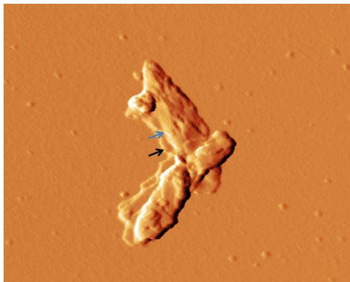
Figure S11. AFM amplitude image of PNIPAM<sub>35</sub>-*b*-PVDF<sub>100</sub> lenticular aggregates. Arrows indicate two stacked lenticular aggregates.
