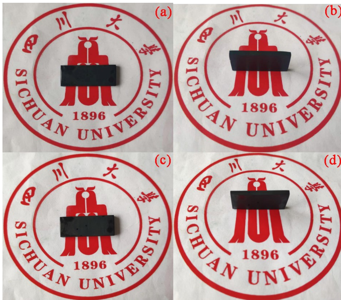
Fig. S5. (a) and (b) were the 375 °C cured resin before DMA test; (c) and (d) were the 375 °C cured resin after DMA test
