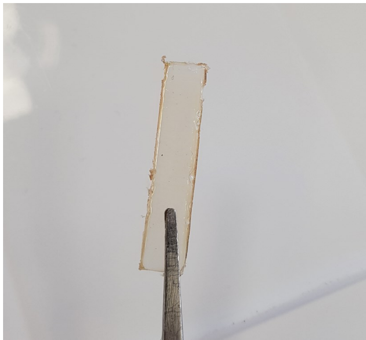
Figure S19. Polymer film of P(N-HBO-MA) prepared by solvent casting
