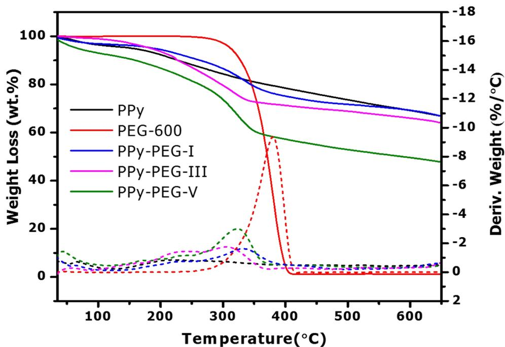
Fig. S7 TGA and DTG curves of the PPy, PEG-600, PPy-PEG-I, PPy-PEG-III and PPy-
