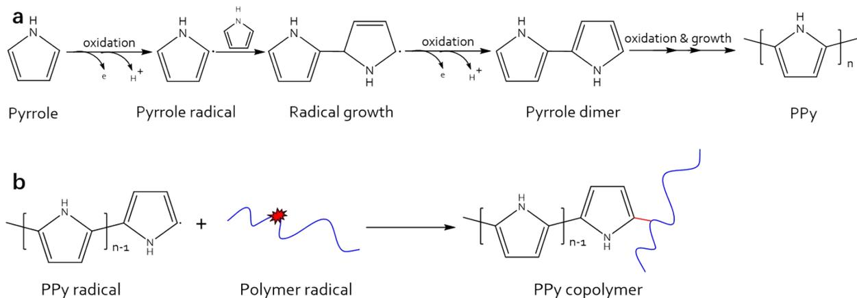
**Fig. S1** (a) Schematic illustration of the synthesis mechanism of PPy by redox polymerization, and (b) the proposed synthesis strategy of PPy copolymer by coupling PPy radicals with additional polymeric radicals.
