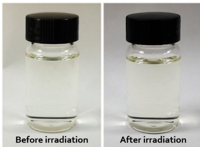
Fig. S5 The PEG-600/pyrrole aqueous solution without  $\text{Fe}^{2+}$  or  $\text{Fe}^{3+}$  before and after gamma-ray irradiation.
