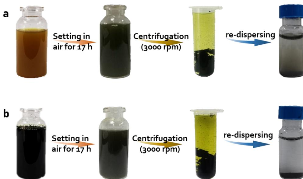
Fig. S4 Schematic illustration of control experiments processes: (a) PEG-600/pyrrole/  $Fe^{2+}$ , and (b) PEG-600/pyrrole/  $Fe^{3+}$ .
