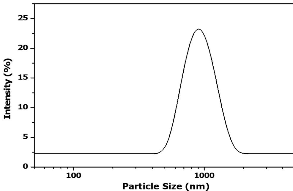
**Fig. S2** The particle size distribution of PEG-PPy-I.
