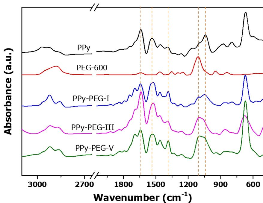
Fig. S6 FT-IR spectra of the PPy, PEG-600, PPy-PEG-I, PPy-PEG-III and PPy-PEG-V.
