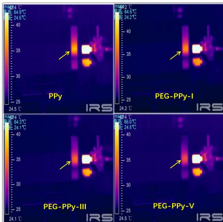
Fig. S10 Photothermal images of various samples dispersed in water ( $1 \text{ mg mL}^{-1}$ ) after 5 min laser irradiation ( $808 \text{ nm}$ ,  $1 \text{ W cm}^{-2}$ ).
