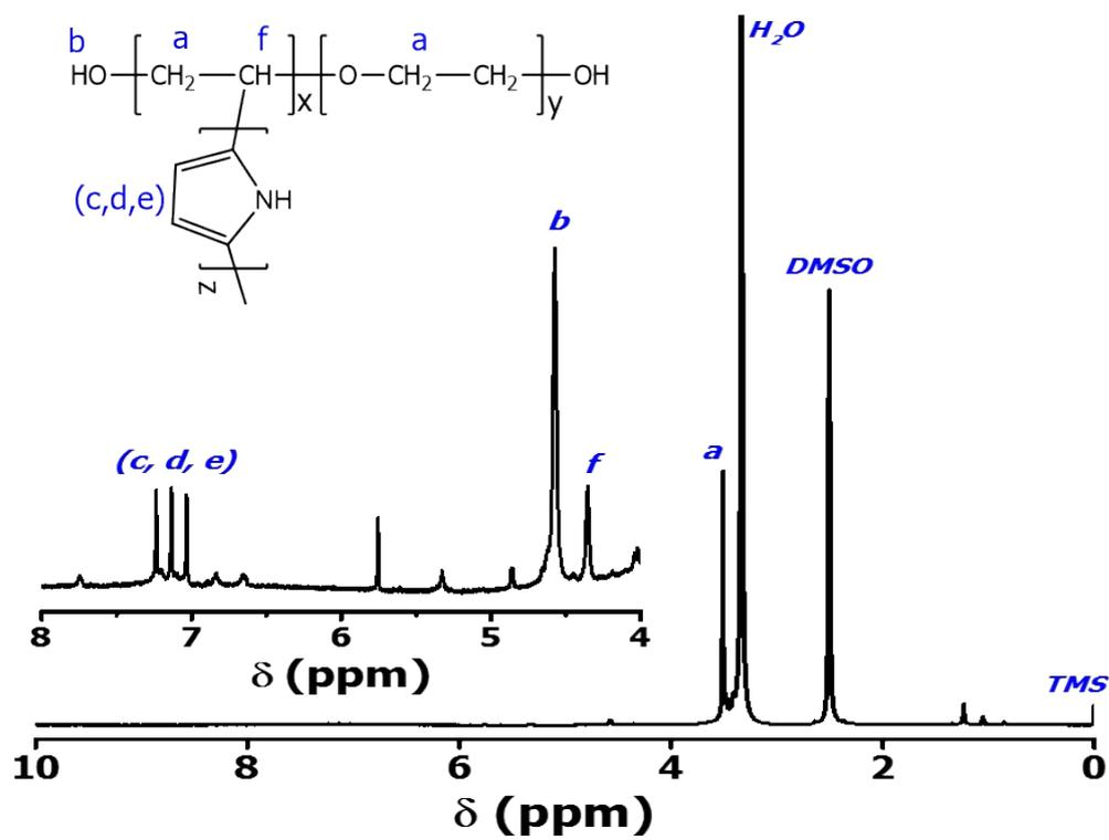
Fig. S9 <sup>1</sup>H-NMR spectrum of PPy-PEG-V.
