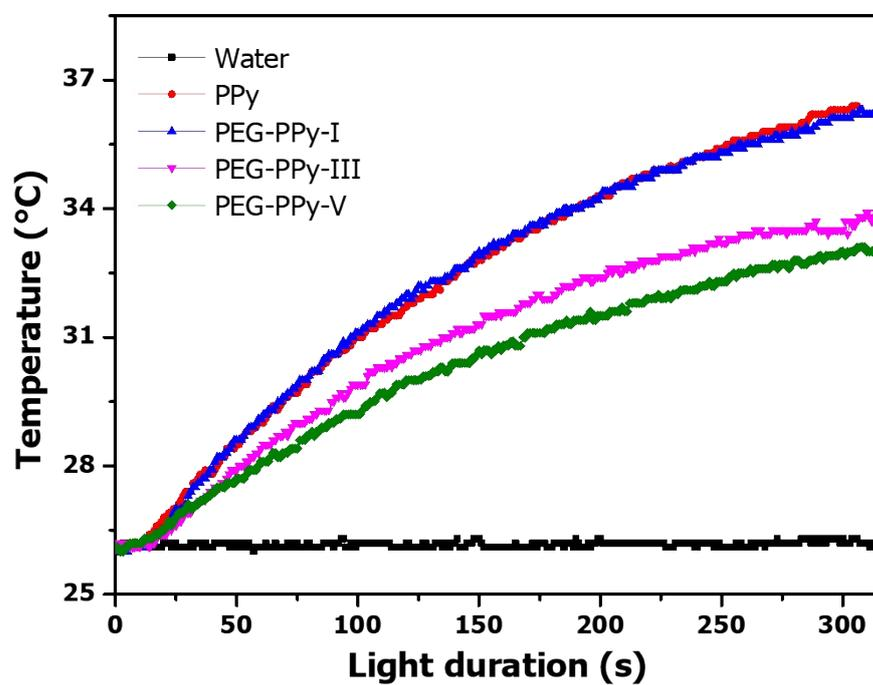
Fig. S11 Temperature change in various samples solutions ( $1 \text{ mg mL}^{-1}$ ) after 5 min laser irradiation ( $808 \text{ nm}$ ,  $1 \text{ W cm}^{-2}$ ).
