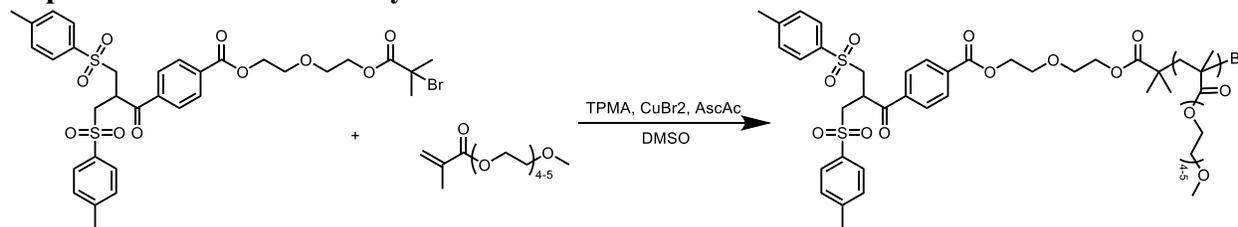
Stock solutions of  $CuBr_2$  (16 mg/mL), tris (2-pyridylmethyl) amine (TPMA, 43 mg/mL), and bis-sulfone initiator (54 mg/mL) were prepared in DMSO in individual dram vials. To a scintillation vial containing PEGMA monomer (0.4 mL, 1.5 mmol, 200 equivalents), 100  $\mu$ L of the  $CuBr_2$  (1.6 mg, 7.4  $\mu$ mol, 1 equivalent), 100  $\mu$ L of the TPMA stock (4.3 mg, 15  $\mu$ mol, 2 equivalents), and
