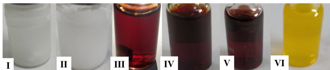
Fig. S1 The different solubility of catalysts at room temperature (I: ZnGA; II: ZnGA at 60 °C after 0.5 hour; III: SalenCo II ; IV: SalenCo II ; V: SalenFe; VI: SalenAl).
