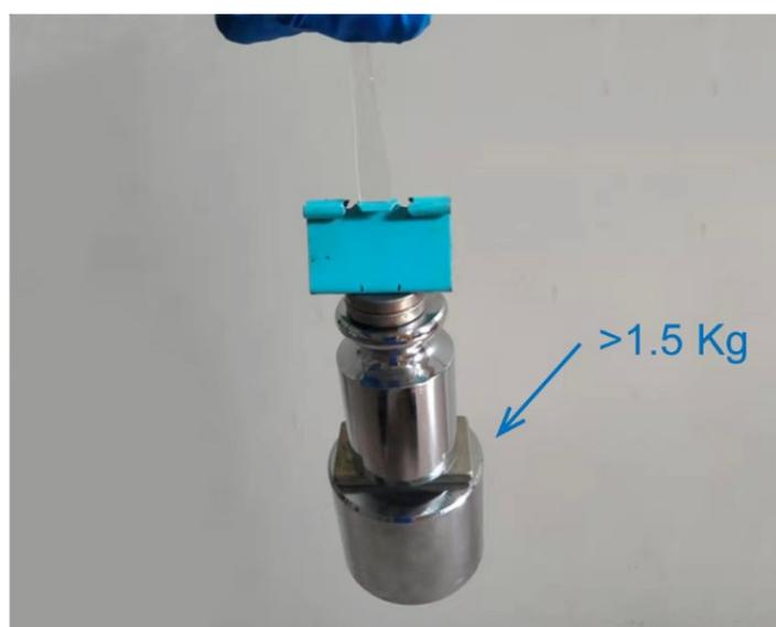
**Figure S10.** A TSHTCE film can lift a 1500 g load without significant elongation, which is 1000 times greater than its own weight.
