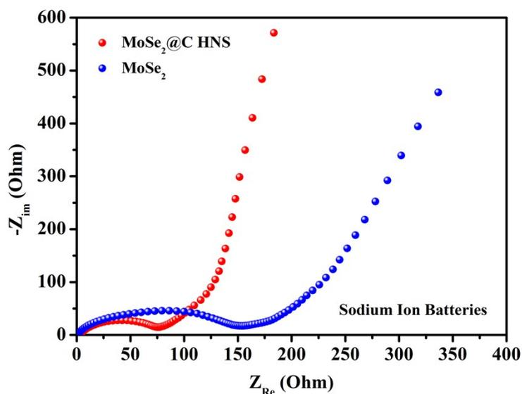
**Figure S10.** Electrochemical impedance spectroscopy of  $\text{MoSe}_2@C$  HNS and bare  $\text{MoSe}_2$  for SIBs.
