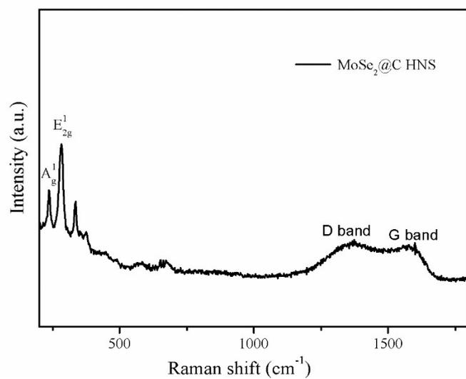
**Figure S7.** Raman scattering spectrum of MoSe<sub>2</sub>@C HNS.
