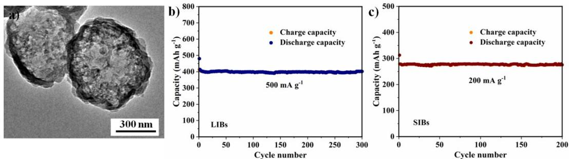
**Figure S9.** a) TEM image of CHNS, b) cycle performance of CHNS in LIBs at a current density of  $500 \text{ mA g}^{-1}$ , c) cycle performance of CHNS in SIBs at a current density of  $200 \text{ mA g}^{-1}$ .
