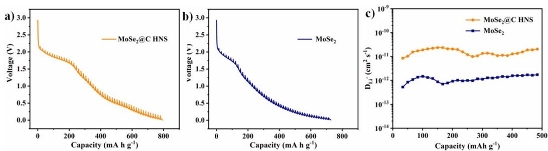
**Figure S11.** GITT curves of  $\text{MoSe}_2@C$  HNS (a) and bare  $\text{MoSe}_2$  (b),  $D_{Li^+}$  value calculated from GITT data (c).
