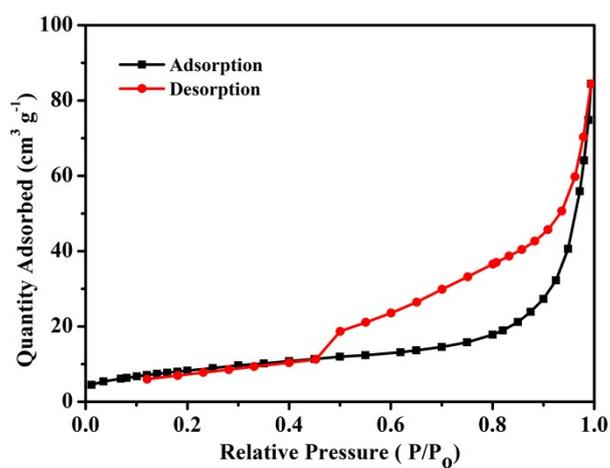
**Figure S4.** a) The nitrogen adsorption/desorption curve of the MoSe<sub>2</sub>@C HNS composite.
