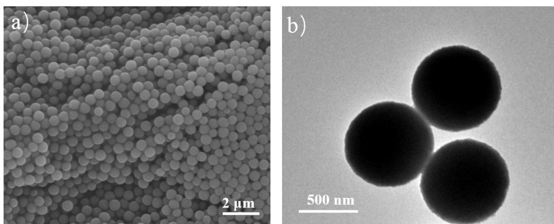
**Figure S1.** SEM and TEM images of MoG solid nanospheres precursors.
