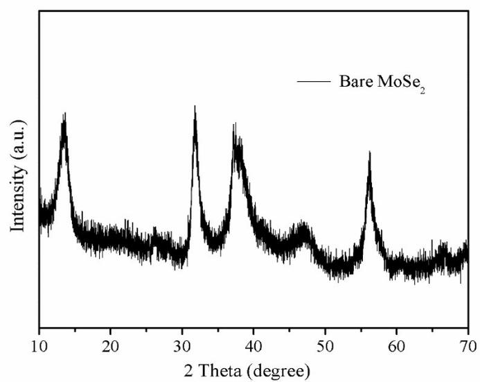
**Figure S6.** XRD pattern of bare MoSe<sub>2</sub>.
