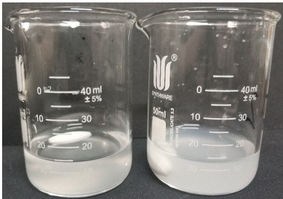
Figure S5. The photographs of SiO 2 -0 (left) and SiO 2 -2 (right) aqueous solution with adsorption of Pb 2+ for 20 min.
