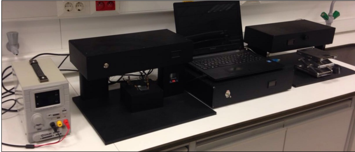
Figure S51. Photoconductivity measurement system used in the Study
