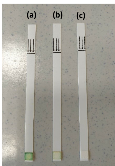
Figure SI35. a) Detection of \text{H}_2\text{O}_2 using Quantifix® peroxide sticks (range 0-25 mg/L \text{H}_2\text{O}_2 , Sigma-Aldrich) for semiquantitative determination of peroxide. The stick was introduced in the crude mixture of a photocatalytic experiment (photooxidation of benzylamine, 1a , in the presence of [\text{Ru3}]\text{Cl}_2 (1 mol %)) after 30 min of reaction and turned blue as a symptom of \text{H}_2\text{O}_2 presence, b) Control experiment, c) Non used stick.
