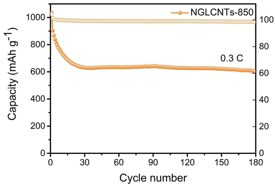
**Figure S10.** Cycling performance of NGLSCNTs-850/S with the sulfur loading of 80% and the areal sulfur mass loading of 2 mg cm<sup>-2</sup> at the rate of 0.3 C.
