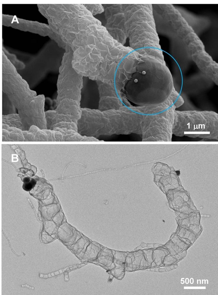
**Figure S4.** FESEM and TEM images of Co/NGLCNTs obtained at the calcination temperature of 950 °C.
