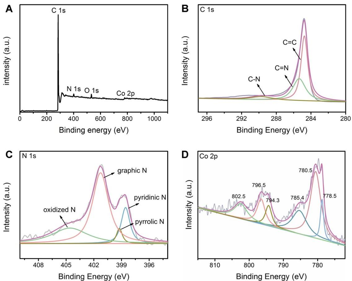
**Figure S7.** XPS spectra of NGLCNTs-850: (A) survey, (B–D) high-resolution spectra of C 1s, N 1s, and Co 2p.
