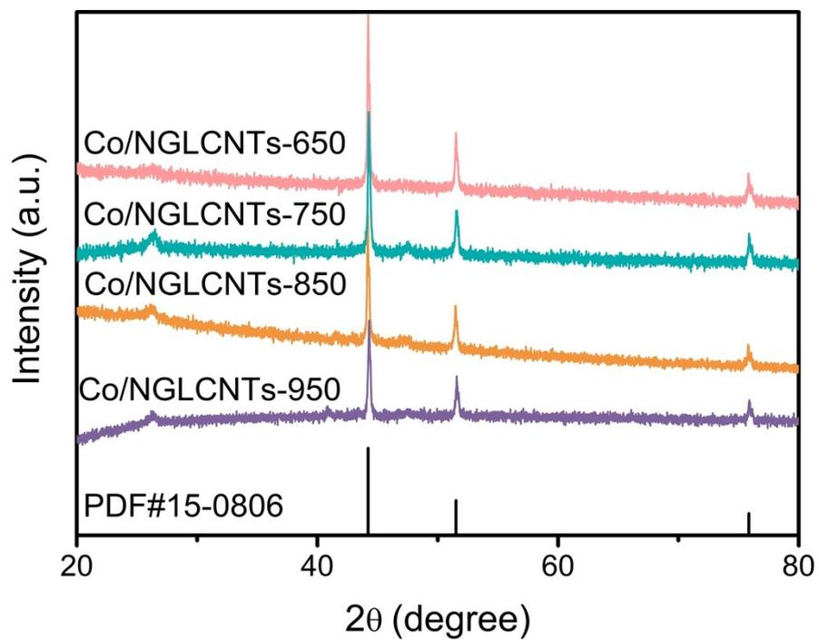
**Figure S6.** XRD patterns of NGLCNTs obtained at different calcination temperatures.
