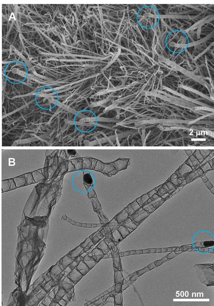
**Figure S1.** FESEM and TEM images of Co/NGLCNTs obtained at the calcination temperature of 850 °C.
