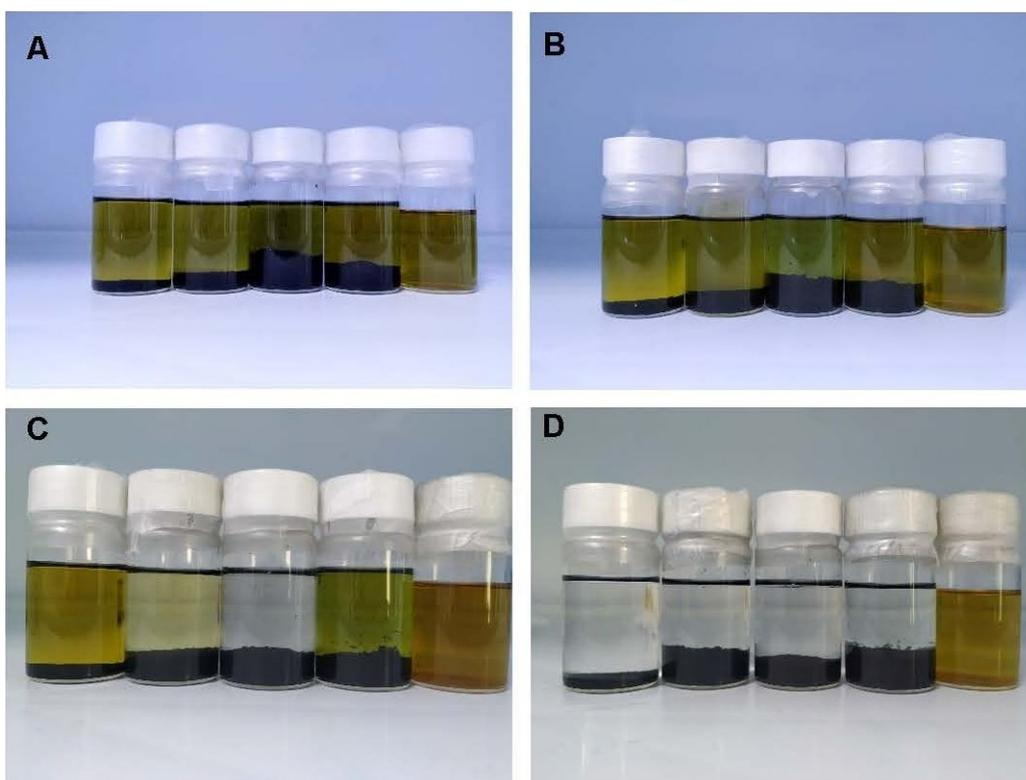
**Figure S9.** Digital pictures of adsorption test of NGLSCNTs-650, -750, -850, -950 and blank solution (from left to right) in  $\text{Li}_2\text{S}_6/\text{DME}$  solution after (A) 5 min and (B) 2 h and (C) 4 h and (D) 48 h.
