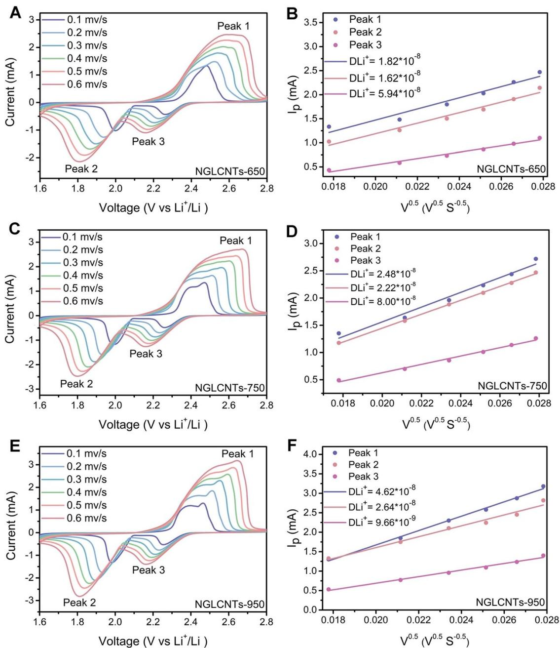
**Figure S8.** CV curves at different sweep rates and  $Li^+$  diffusion coefficients (A, B) NGLSCNTs-650, (C, D) NGLSCNTs-750, (E, F) NGLSCNTs-950.
