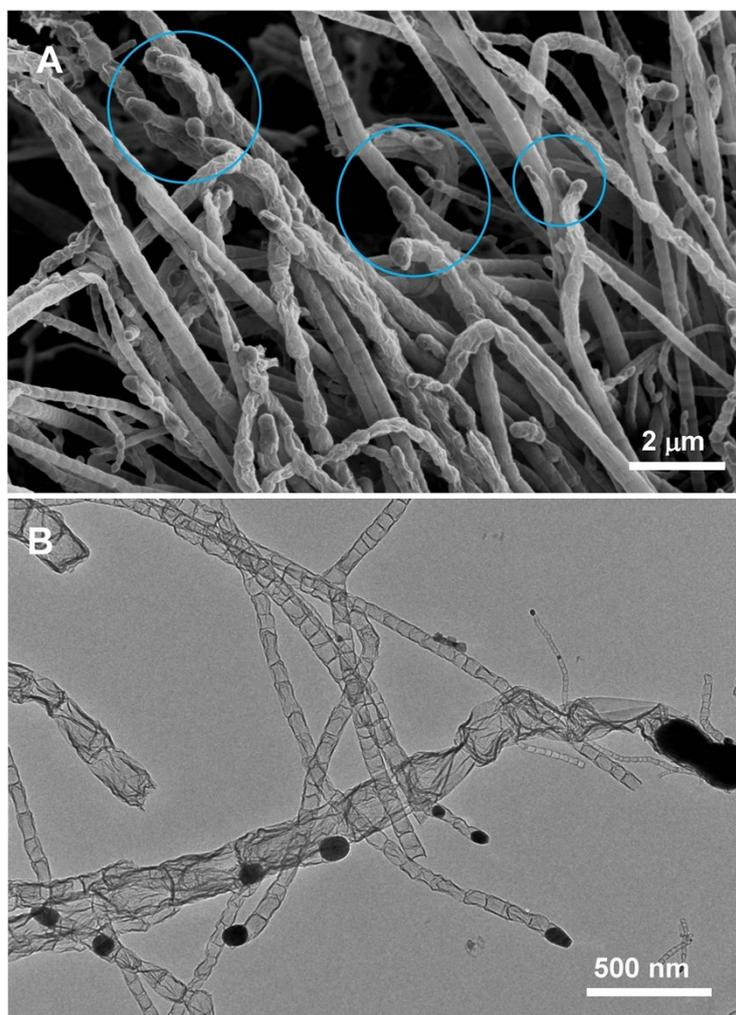
**Figure S2.** FESEM and TEM images of Co/NGLCNTs obtained at the calcination temperature of 650 °C.
