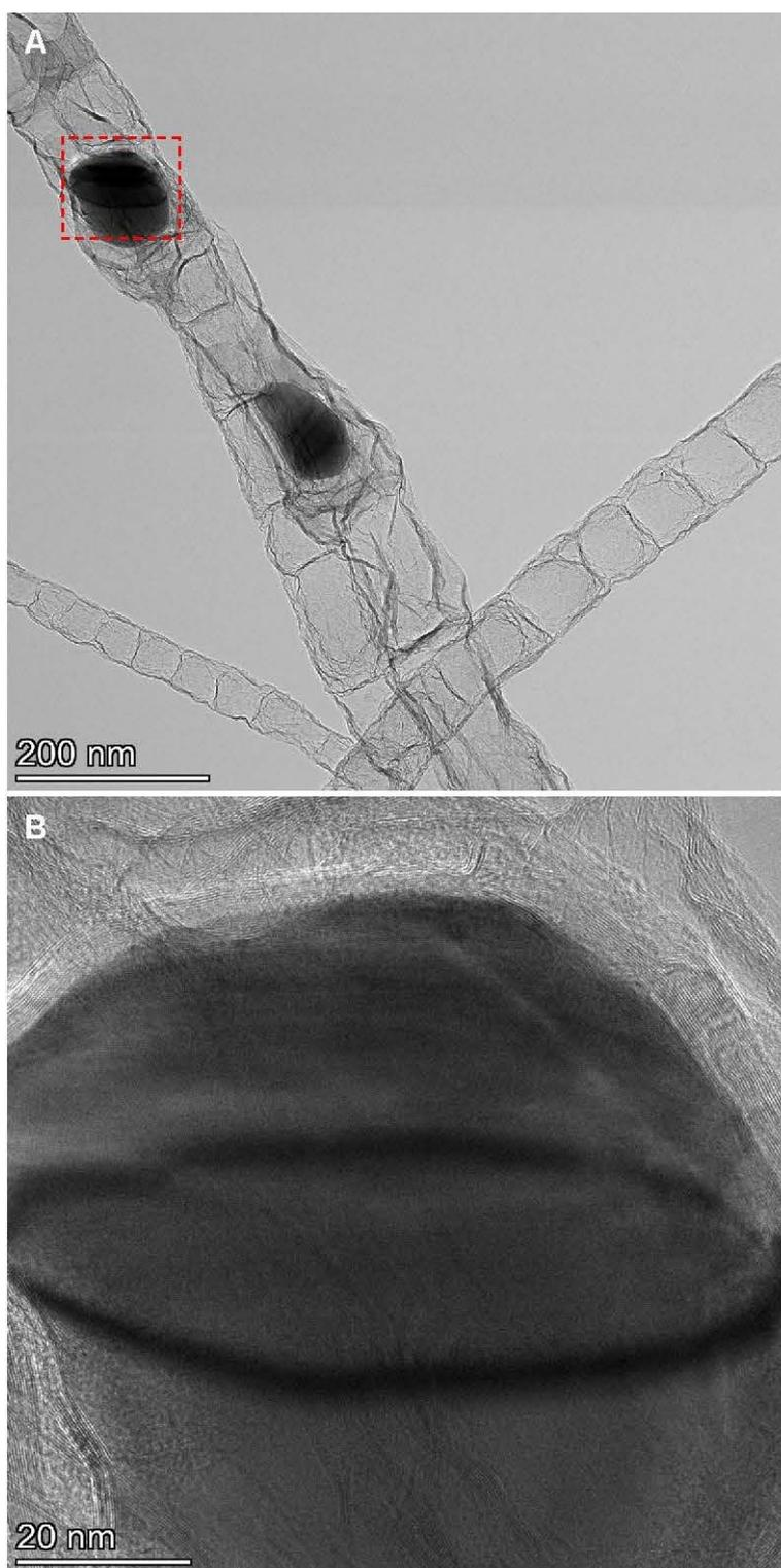
**Figure S5.** (A) Low-magnification TEM image of of the NGLCNTs. (A) HRTEM image of few-layer graphene coated Co nanoparticle recorded from a marked with red boxes in (A).
