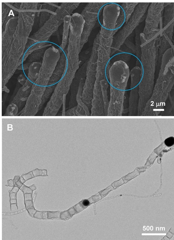
**Figure S3.** FESEM and TEM images of Co/NGLCNTs obtained at the calcination temperature of 750 °C.
