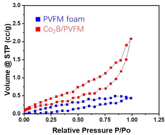
Figure S4 The BET curves of pristine PVFM and  $\text{Co}_2\text{B}/\text{PVFM}$
