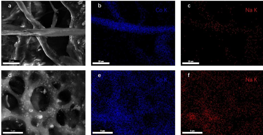
Figure S3 SEM images and EDS mapping of the  $\text{Co}_2\text{B}/\text{PVFM}$  sponge after catalyzing the hydrolysis of 10 wt% (a, b, c) and 30 wt% (d, e, f)  $\text{NaBH}_4$  solution.
