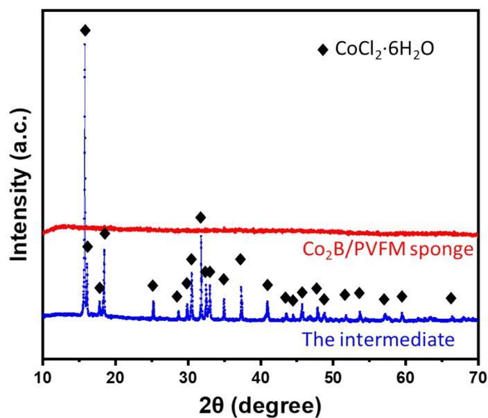
Figure S1 XRD pattern of  $\text{Co}_2\text{B}/\text{PVFM}$  sponge and the intermediate.
