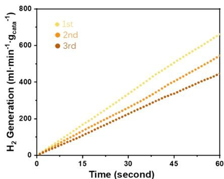
Figure S6 The hydrolysis kinetics of 20 wt%  $NaBH_4$  solution at 298 K catalysed by the  $Co_2B/PVDMF$  sponge catalyst in 3 consecutive test.
