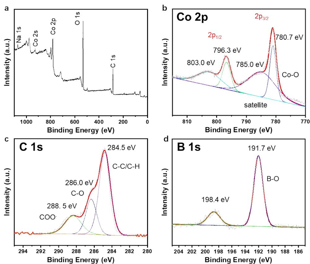
Figure S2 XPS spectra and curve fitting profiles of  $\text{Co}_2\text{B}/\text{PVFM}$  sponge: (a) survey, (b) Co 2p, (c) C 1s and (d) B 1s.
