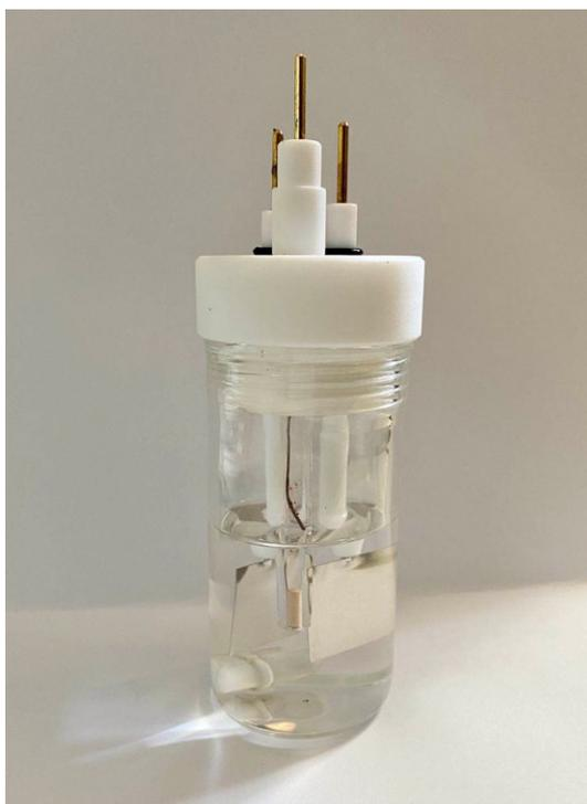
**Figure S1.** Optical graph of an electrolytic cell with a three-electrode system.
