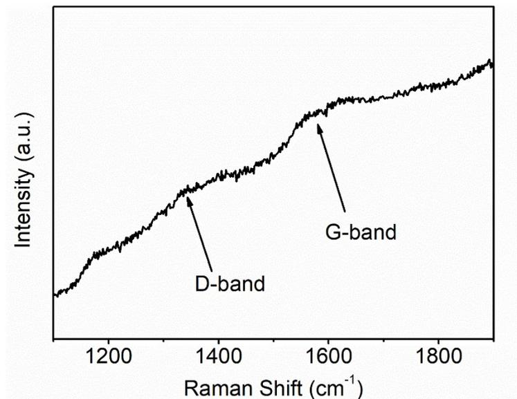
Fig. S3 Raman spectrum of the prepared CDs.
