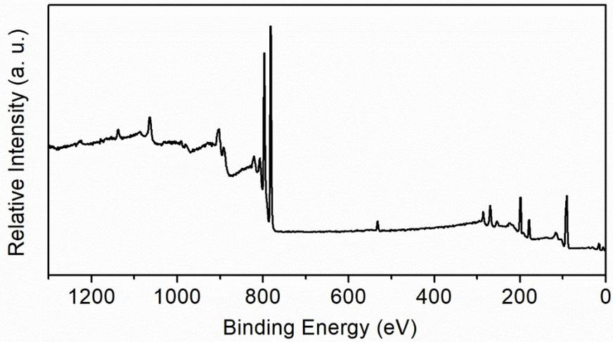
Fig. S4 XPS survey spectrum of CDs@BaCl<sub>2</sub>.
