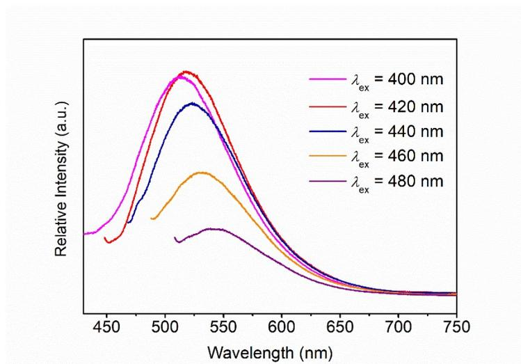
Fig. S5 PL spectra of CDs@BaCl<sub>2</sub> under different excitation wavelengths.
