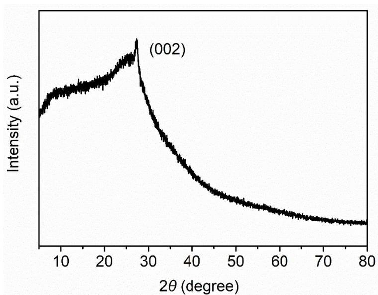
Fig. S2 XRD patterns of the prepared CDs.
