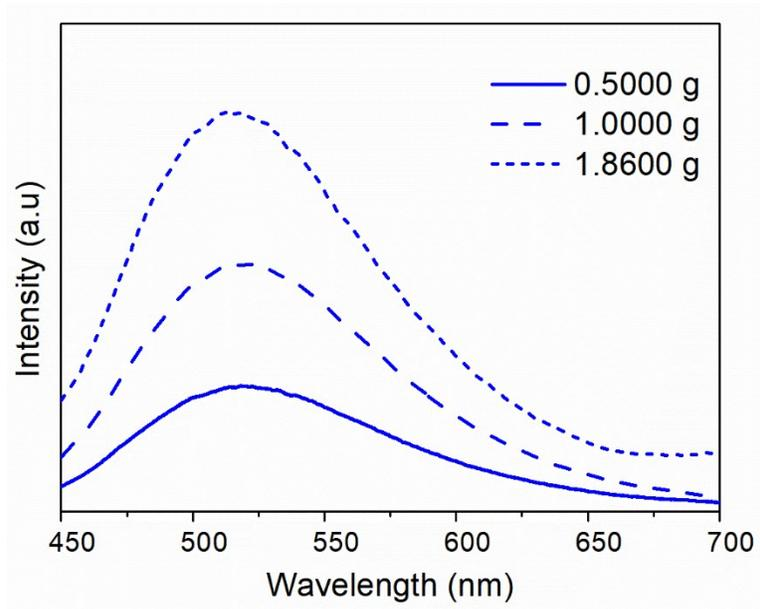
Fig. S6 PL spectra of the CDs@BaCl<sub>2</sub> phosphors made with different weights of BaCl<sub>2</sub>.
