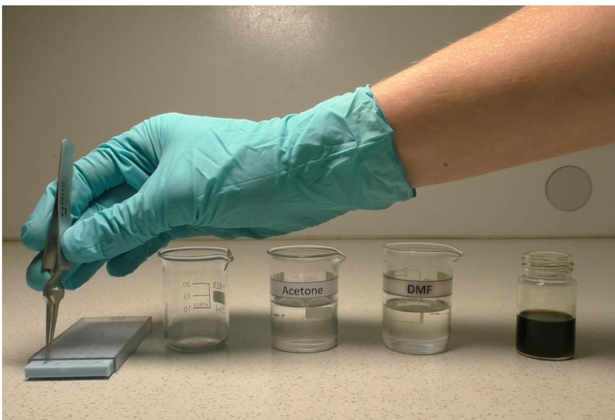
**Figure S7.** Pick the grid with reverse tweezers.
