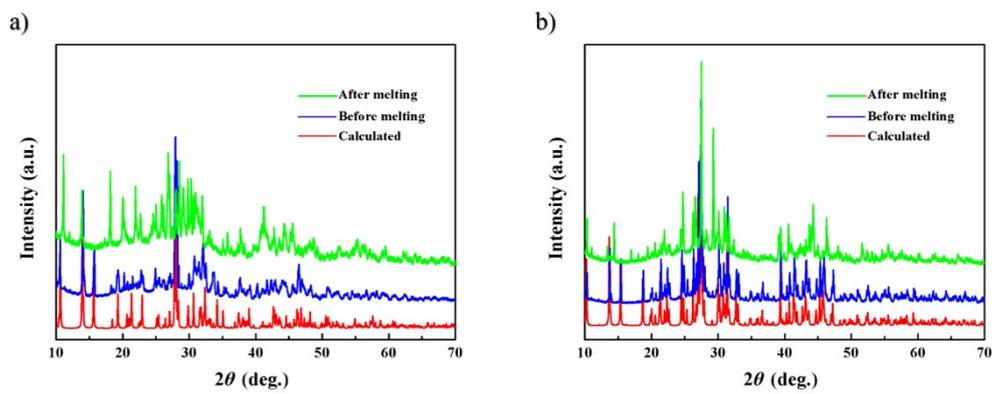
**Figure S1.** PXRD patterns of a)  $K_3SrBi(P_2O_7)_2$  and b)  $Rb_3SrBi(P_2O_7)_2$ .
