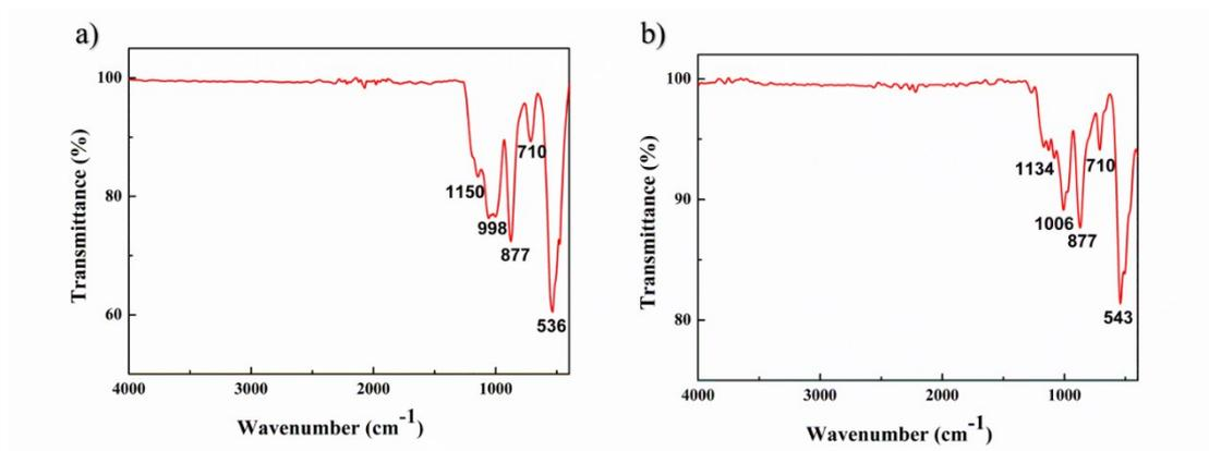
**Figure S4.** IR spectra of a) K<sub>3</sub>SrBi(P<sub>2</sub>O<sub>7</sub>)<sub>2</sub> and b) Rb<sub>3</sub>SrBi(P<sub>2</sub>O<sub>7</sub>)<sub>2</sub>.
