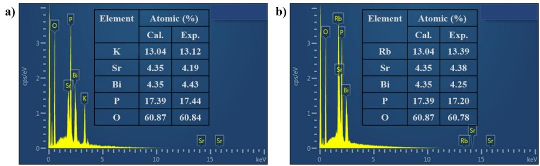
**Figure S6.** EDS spectra of a)  $K_3SrBi(P_2O_7)_2$  and b)  $Rb_3SrBi(P_2O_7)_2$ .
