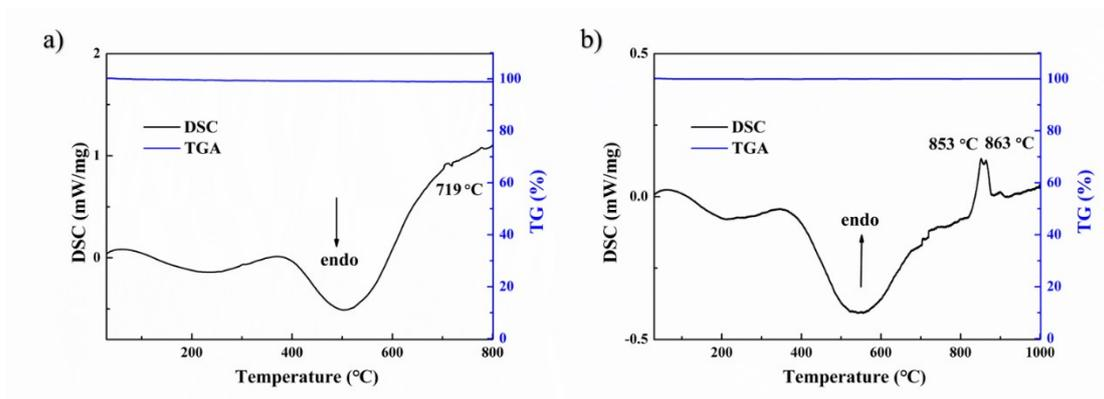
Figure S5. TG and DSC curves of a)  $K_3SrBi(P_2O_7)_2$  and b)  $Rb_3SrBi(P_2O_7)_2$ .
