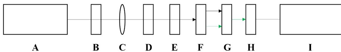
**Figure S7.** Experimental optical path diagram of SHG measurement (A: Nd<sup>3+</sup> laser, B: filter, C: lens, D: attenuator, E: 1064 nm filter, F: sample, G: 532 nm filter, H: photomultiplier tube, I: oscilloscope).
