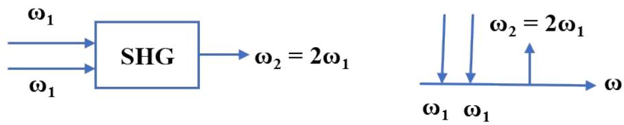
**Figure S8.** The schematic diagram of the second harmonic generation (SHG).
