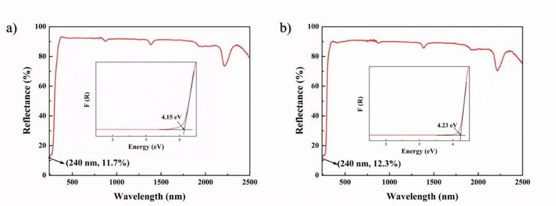
**Figure S3.** UV-Vis-NIR diffuse reflectance and absorption spectra of a)  $K_3SrBi(P_2O_7)_2$  and b)  $Rb_3SrBi(P_2O_7)_2$ .
