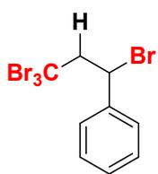
**(1,3,3,3-tetrabromopropyl) benzene.** Purified using column chromatography over silica (60-120 mesh) as colourless oil in 68% yield.  $^1\text{H}$  NMR (400 MHz,  $\text{CDCl}_3$ )  $\delta$  7.49 (d,  $J = 7.3$  Hz, 2H), 7.40 – 7.31 (m, 3H), 5.38 – 5.27 (m, 1H), 4.16 – 4.02 (m, 2H).  $^{13}\text{C}$  NMR (101 MHz,  $\text{CDCl}_3$ )  $\delta$  140.78, 128.99, 128.91, 128.18, 66.44, 50.09, 35.04.
