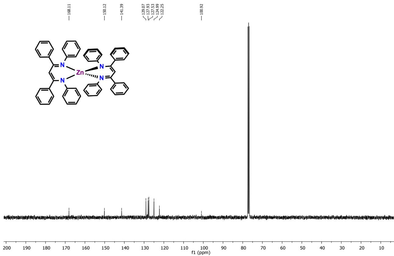
**Fig S6:**  $^{13}\text{C}$  NMR spectrum of **2a** recorded in CDCl<sub>3</sub>, solvent residual peak is at 77.4 ppm.
