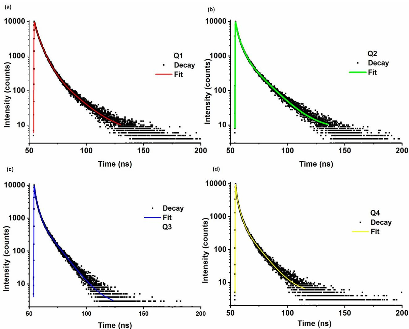
**Fig S11:** Tri-exponential fit of TCSPC data for **2a** when excitation was done with 374 nm laser and emitted photon was collected at 415 nm.
