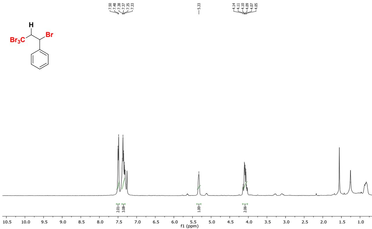
Fig S20: <sup>1</sup>H NMR spectrum recorded in CDCl<sub>3</sub>, solvent residual peak is at 7.26 ppm.
