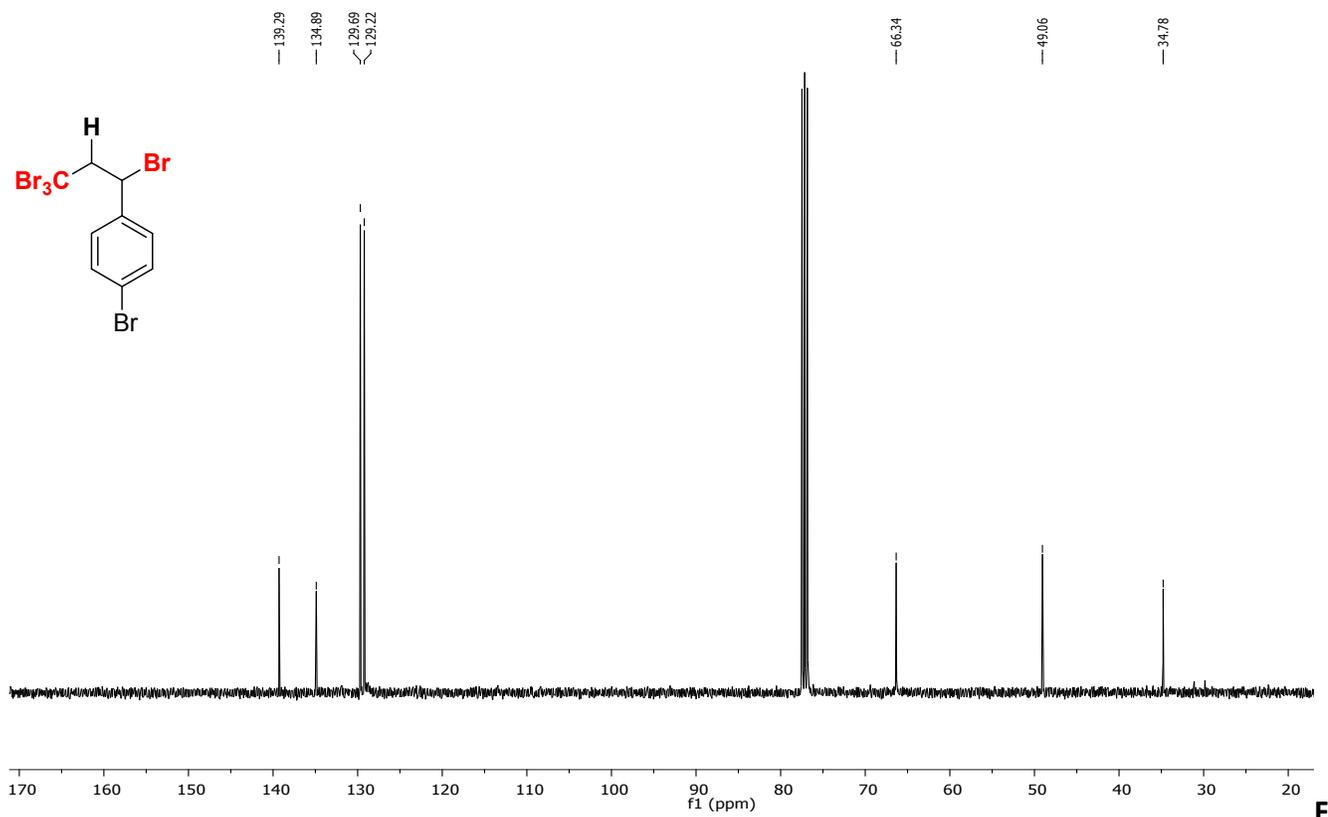
ig S27: The <sup>13</sup>C NMR spectrum recorded in CDCl<sub>3</sub>, solvent residual peak is at 77.4 ppm.
