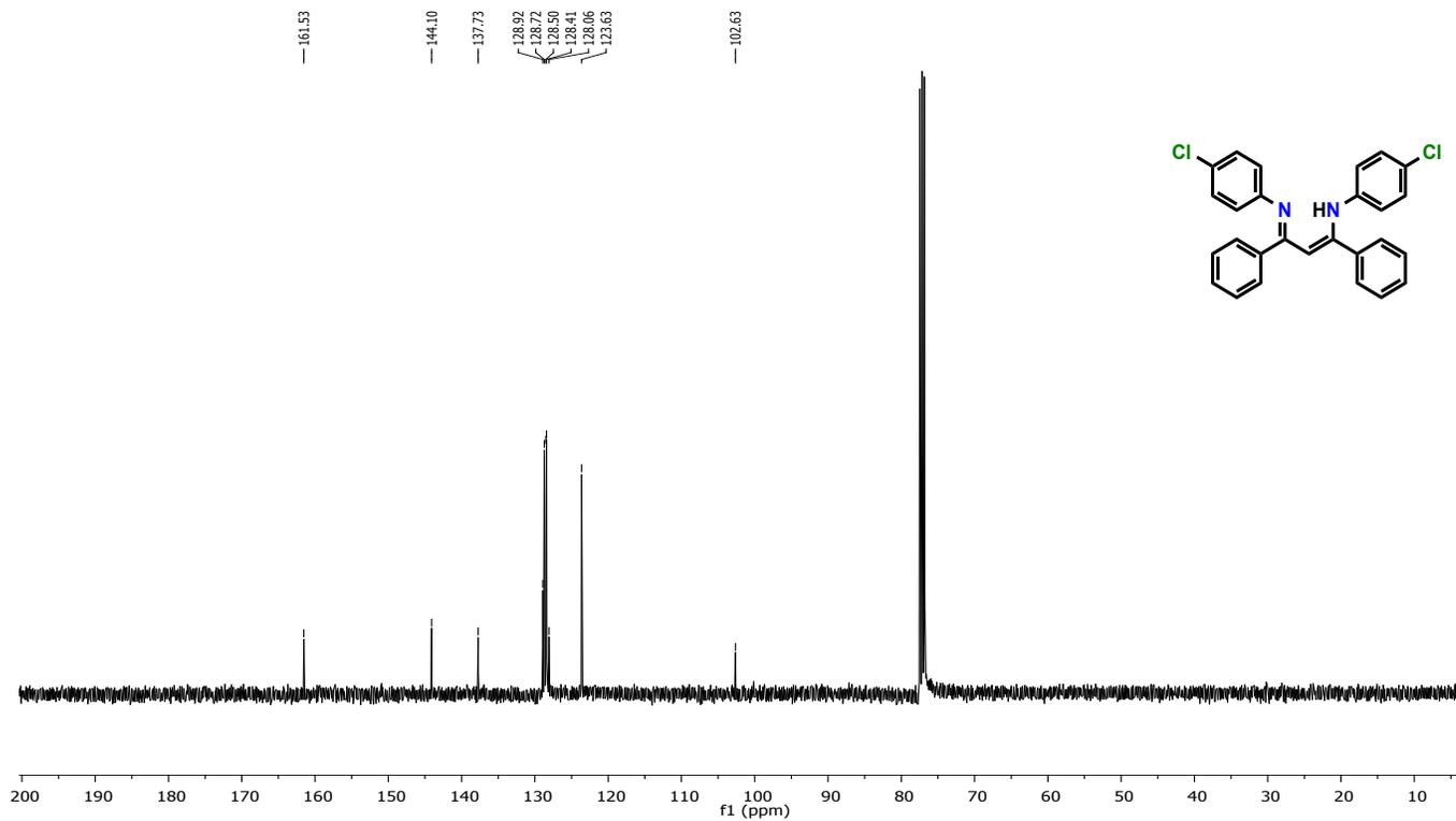
**Fig S4:** <sup>13</sup>C NMR spectrum of **1b** recorded in CDCl<sub>3</sub>, solvent residual peak is at 77.4 ppm.
