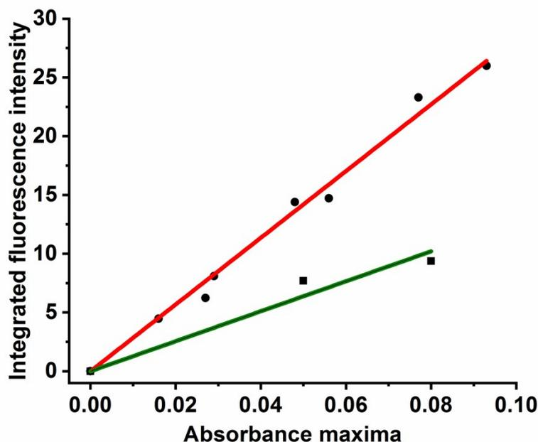
**Fig S10:** Linear fitted plots of integrated fluorescence intensity at absorbance maxima vs corresponding absorbance maxima, for emission quantum yield measurements of **1a** (sample) with **2a** (reference).
