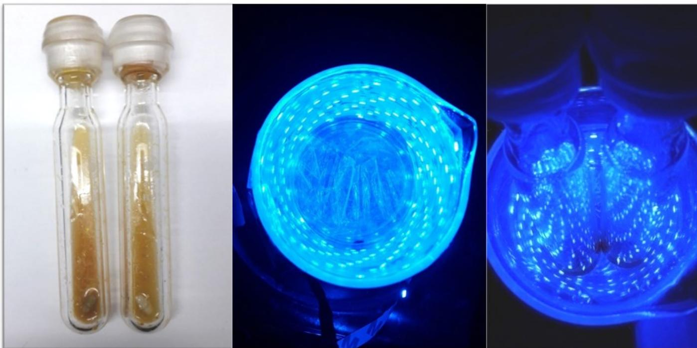
**Fig S15:** Sealed tubes packed under anaerobic atmosphere and kept for stirring in blue light setup.
