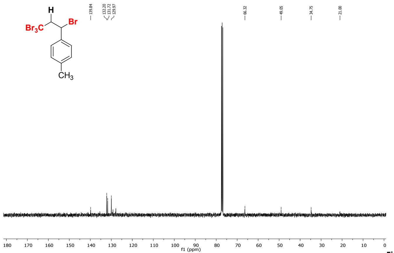
**g S29:** The  $^{13}\text{C}$  NMR spectrum recorded in  $\text{CDCl}_3$ , solvent residual peak is at 77.4 ppm.
