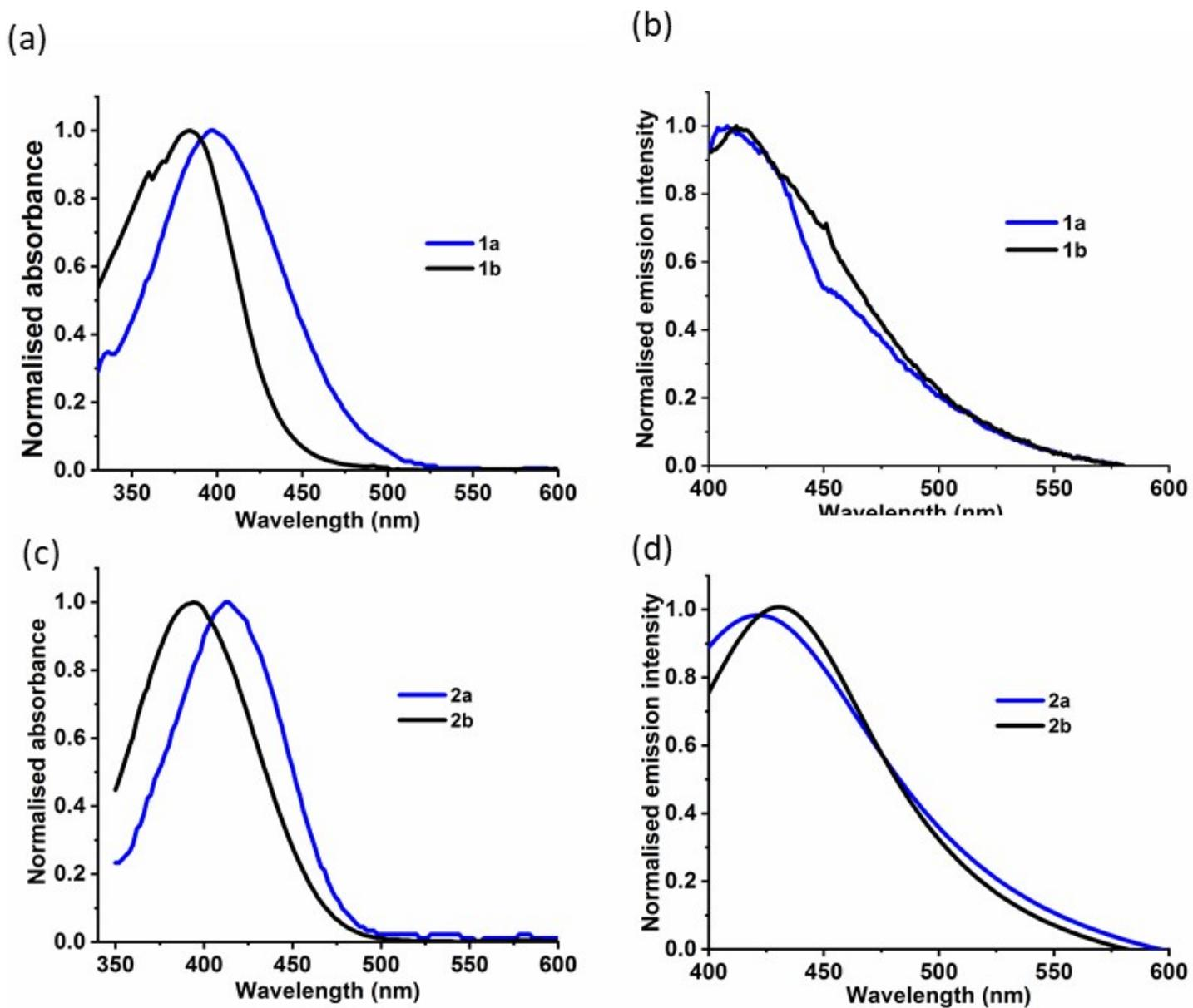
**Fig S9:** (a) Comparison of normalised absorption intensities of ligand **1a** and **1b**, (b) normalised emission intensities of ligands **1a** and **1b**, (c) normalised absorption intensities of zinc complexes **2a** and **2b**, (d) normalised emission intensity of zinc complexes **2a** and **2b**.
