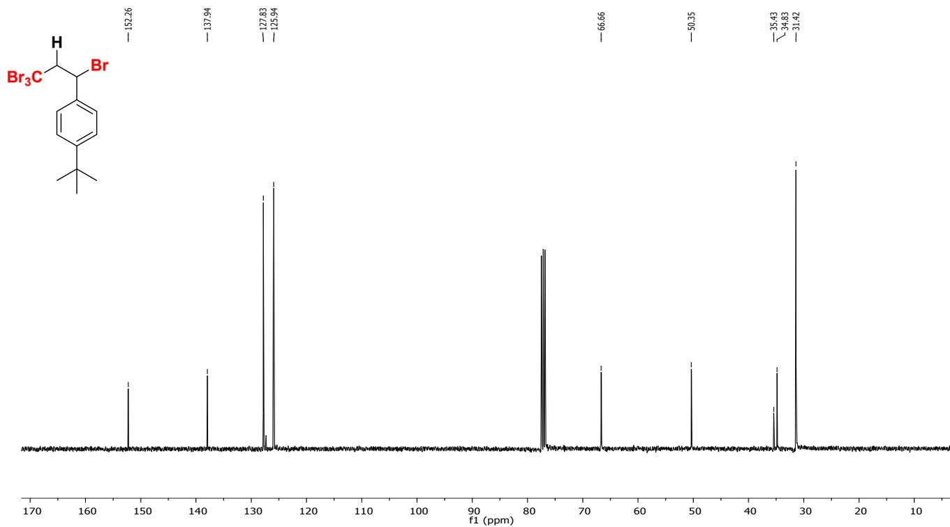
Fig S25:  $^{13}\text{C}$  NMR spectrum recorded in  $\text{CDCl}_3$ , solvent residual peak is at 77.4 ppm.
