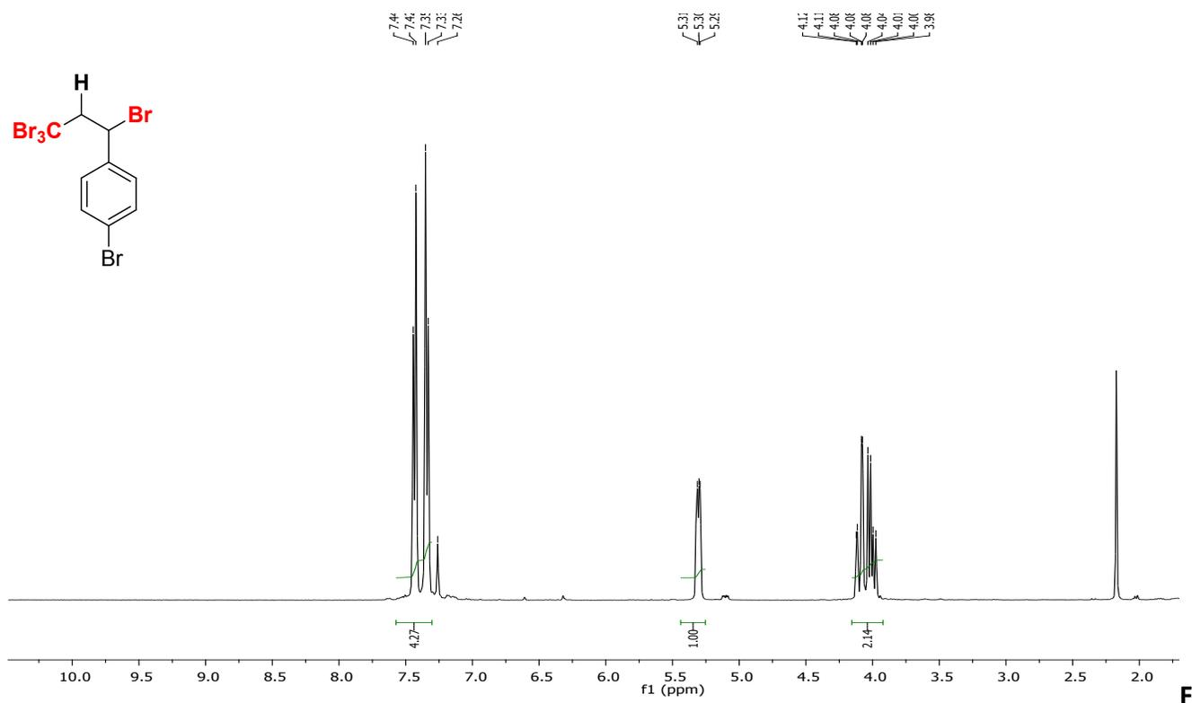
ig S26: <sup>1</sup>H NMR spectrum recorded in CDCl<sub>3</sub>, solvent residual peak is at 7.26 ppm.
