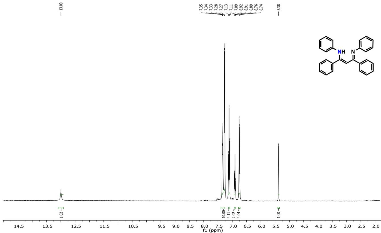
**Fig S1:**  $^1\text{H}$  NMR spectrum of **1a** recorded in  $\text{CDCl}_3$ , solvent residual peak is at 7.26 ppm.
