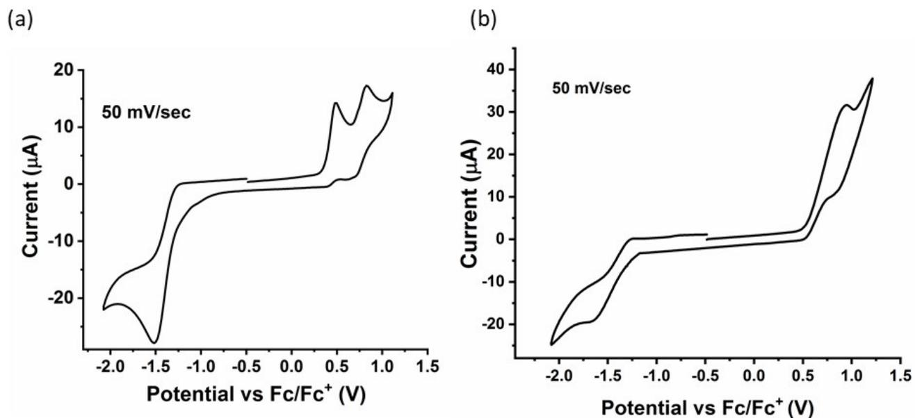
**Fig S13:** a) CV of 1 mM of **2a** in DCM where 0.1 M solution of tetrabutyl-ammonium hexafluorophosphate salt was used as an electrolyte, b) CV of **2b** in DCM under the same conditions.
