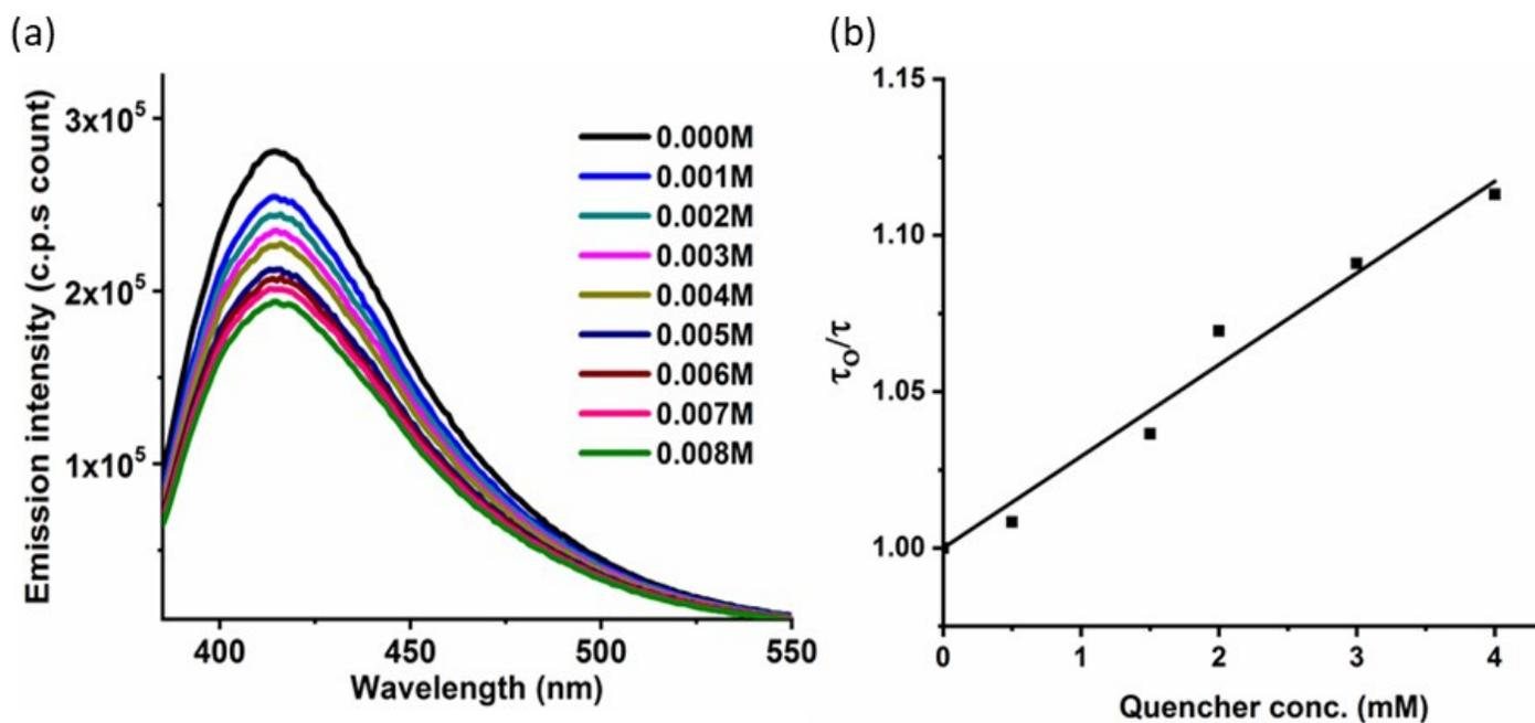
**Fig S16:** (a) Fluorescence-quenching of **2a** upon excitation at 370 nm in DCM (b) Lifetime-quenching of **2a** upon excitation at 374 nm laser in DCM in the presence of DIPEA
