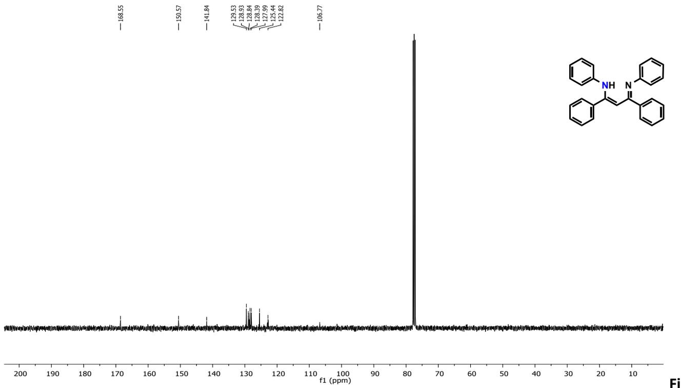
**g S2:**  $^{13}\text{C}$  NMR spectrum of **1a** recorded in  $\text{CDCl}_3$ , solvent residual peak is at 77.36 ppm.
