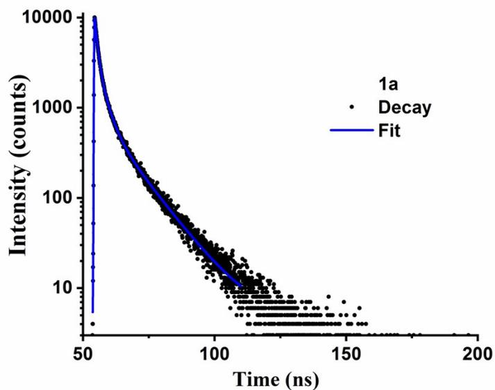
**Fig S12:** Bi-exponential fit for ligand **1a**, at 410 nm and 374 nm excitation laser.
