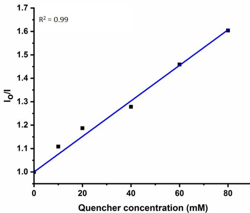
**Fig S17:** Stern-Volmer quenching of **2a** in anhydrous DCM under inert atmosphere when TEA is used as a sacrificial photoreductant.
