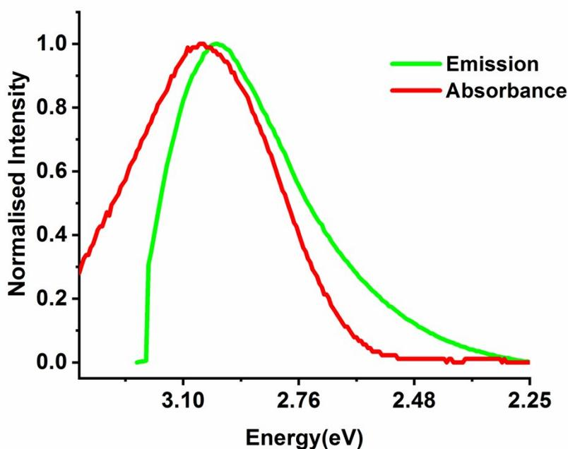
**Fig S14:** Normalized absorption and emission spectra of **2a** in DCM. The value of  $E_{00}$  has been considered as the energy at their point of intersection.
