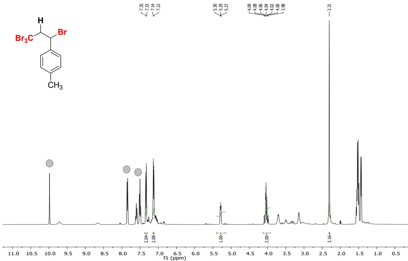
**Fig S28:** <sup>1</sup>H NMR spectrum recorded in CDCl<sub>3</sub>, the symbol (●) designates the resonances for internal standard 4-chlorobenzaldehyde.
