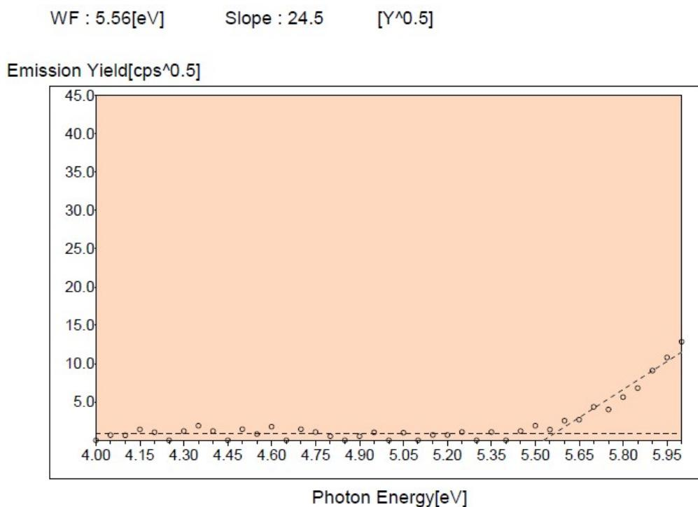
**Fig. S3.** PESA spectrum of thin film of **R1**. The dashed-lines show the fits to extract ionisation potential (-5.56 eV) which corresponds to the HOMO energy level.
