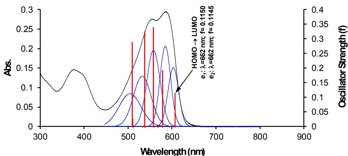
**Fig. S2.** The UV-vis spectrum of **R1** and the singlet electronic transitions as calculated using the TD-DFT at the B3LYP/6-311+G(d,p)//B3LYP/6-31G level of theory *in vacuo*.
