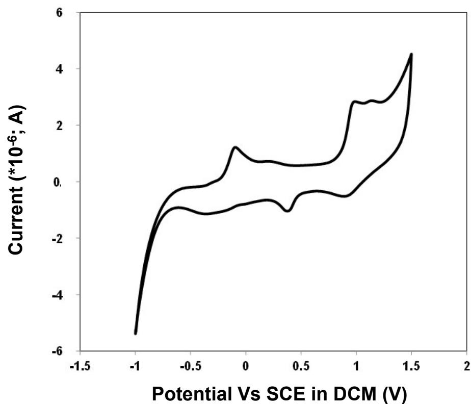
**Fig. S4.** Cyclic voltammogram of **R1**, run in dichloromethane at a sweep rate of 50 mV sec<sup>-1</sup>.
