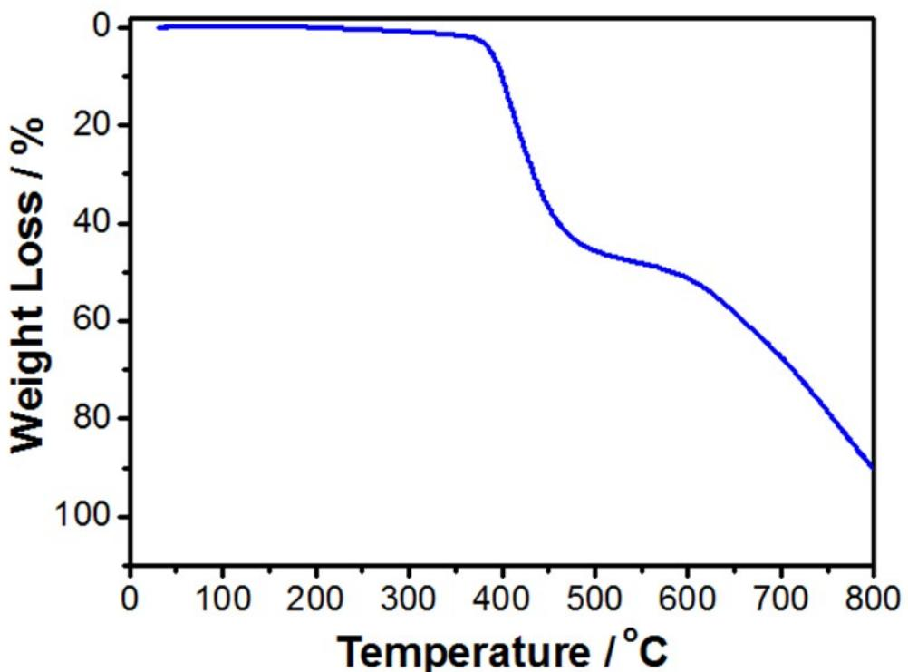
**Fig. S5.** TGA curve showing thermal stability of **R1**.
