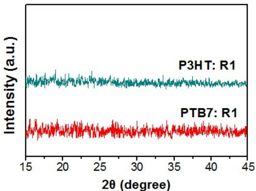
**Fig. S6.** XRD spectra for the active blend surfaces of R1. The XRD spectra indicate the blend surfaces to be amorphous.
