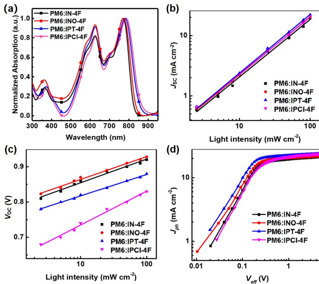
**Figure S15.** (a) Absorption spectra of the optimized blended films. (c)  $J_{SC}$  versus light intensity, (c)  $V_{OC}$  versus light intensity of the optimized devices, and (d)  $J_{ph}$  versus  $V_{eff}$ .
