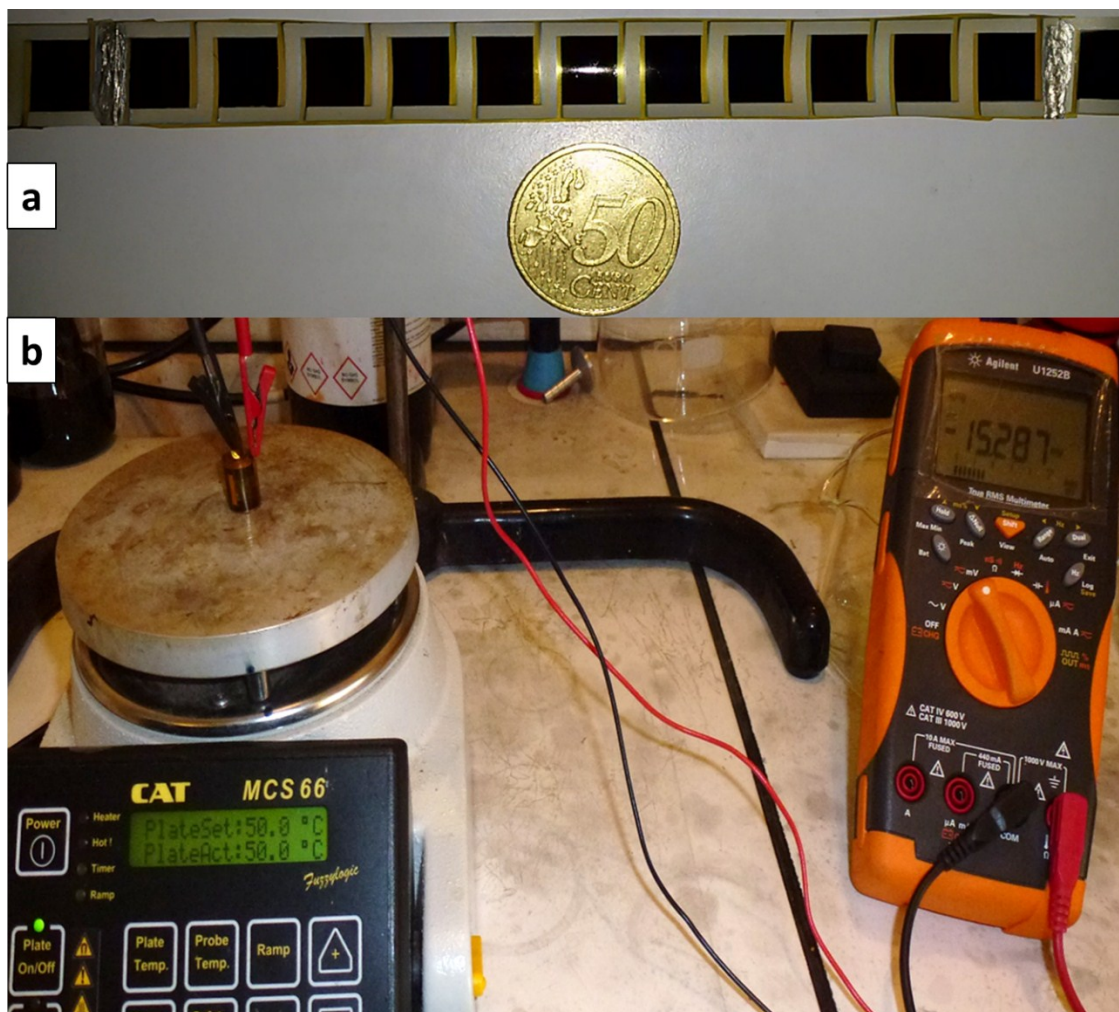
Figure S7. (a) Details of 2D PEDOT:OTf and silver thermocouples before rolling. (b) 156 rolled thermocouples used in real conditions on a hotplate. Here, R_i = 2,9 \text{ k}\Omega and due to poor thermal resistance between the hotplate and the TEG, the measured power on the picture is P_{OC} = 20 \text{ nW} .
