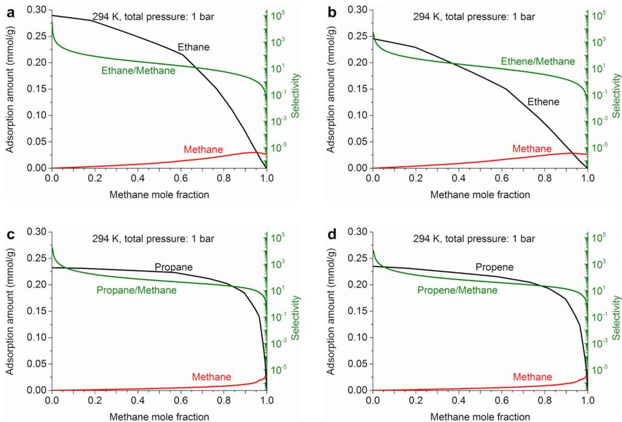
Figure S11. IAST-predicted adsorption amount and selectivity of mixed gases on Zn seed: a). Ethane and methane; b). Ethene and methane; c). Propane and methane; d). Propene and methane
