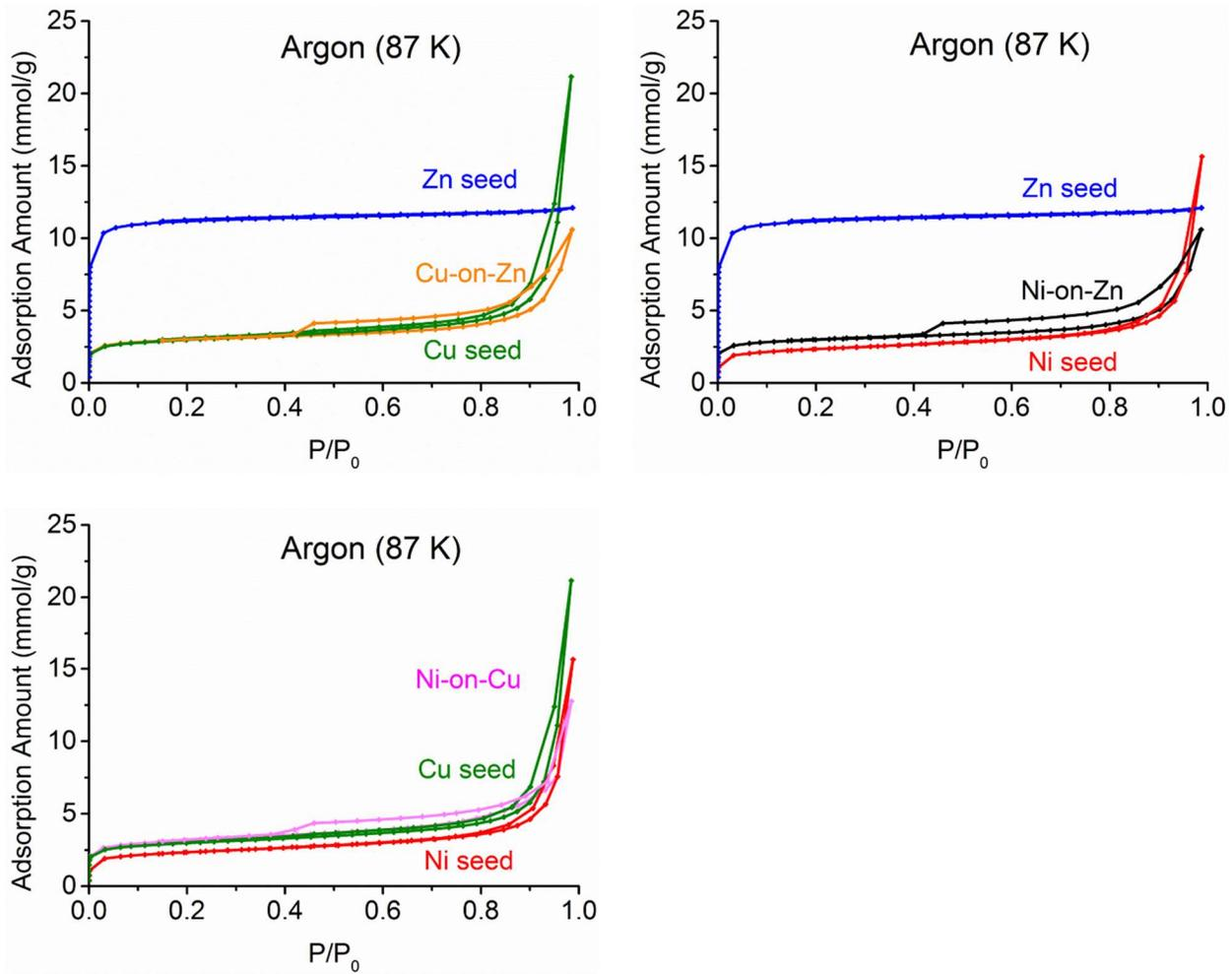
Figure S12. Adsorption isotherm of Argon on Zn seed, Cu seed and Cu-on-Zn intergrowth, Zn seed, Ni seed and Ni-on-Zn intergrowth, Ni seed, Cu seed and Ni-on-Cu intergrowth
