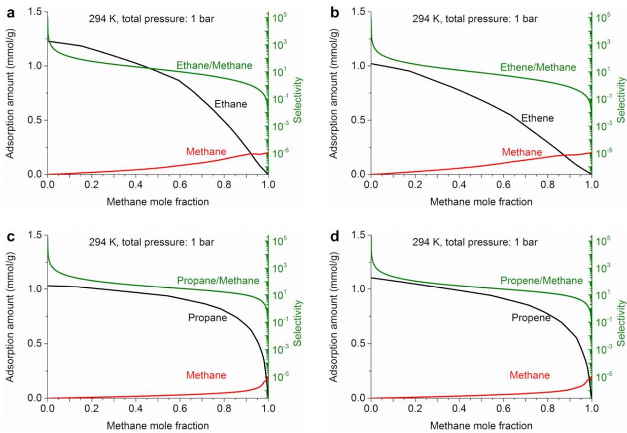
Figure S8. IAST-predicted adsorption amount and selectivity of mixed gases on Cu-on-Zn intergrowth: a). Ethane and methane; b). Ethene and methane; c). Propane and methane; d). Propene and methane
