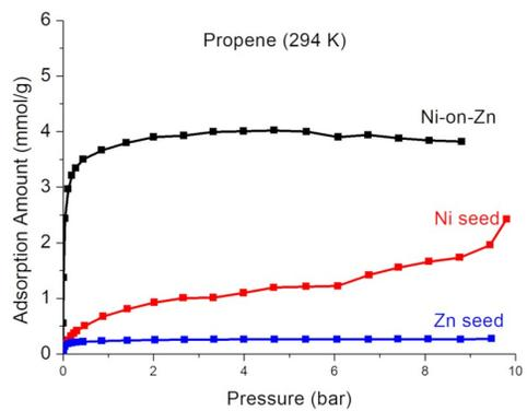
Figure S4. Adsorption isotherm of methane, ethane, ethene, propane, and propene on Ni seed, Zn seed and Ni-on-Zn intergrowth
