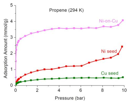
Figure S5. Adsorption isotherm of methane, ethane, ethene, propane, and propene on Ni seed, Cu seed and Ni-on-Cu intergrowth
