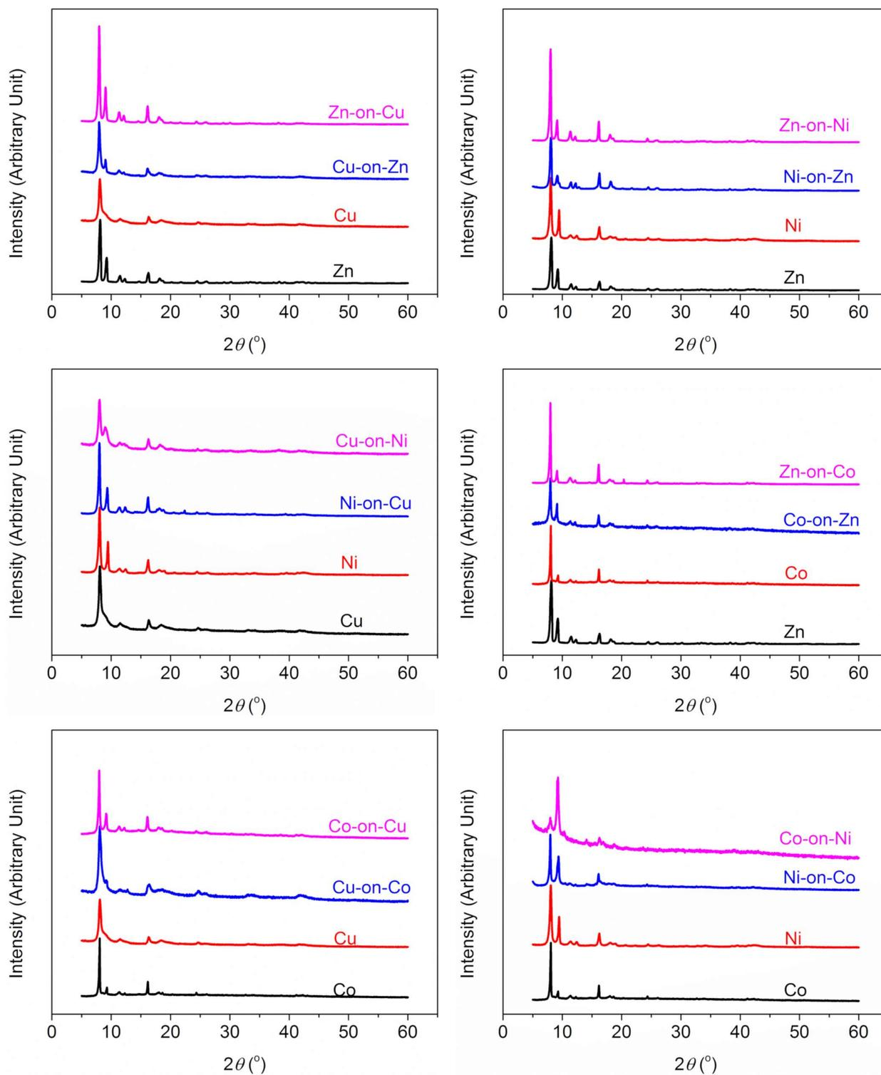
Figure S1. Powder XRD patterns of intergrowth MOFs  $M^{II}_2(ndc)_2(dabco)$  on  $M^I_2(ndc)_2(dabco)$  ( $M^{II}$  and  $M^I = Cu, Zn, Ni, Co$ )
