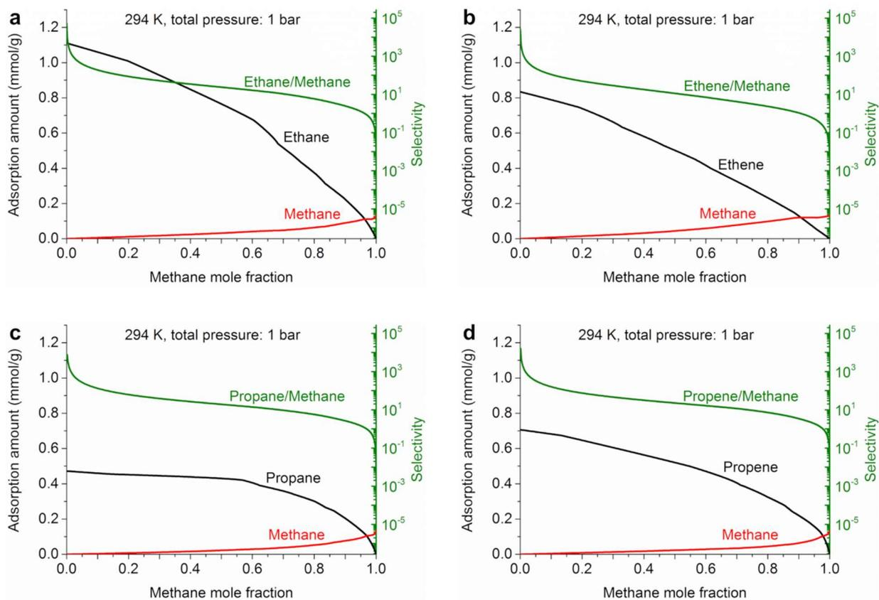
Figure S10. IAST-predicted adsorption amount and selectivity of mixed gases on Ni seed: a). Ethane and methane; b). Ethene and methane; c). Propane and methane; d). Propene and methane
