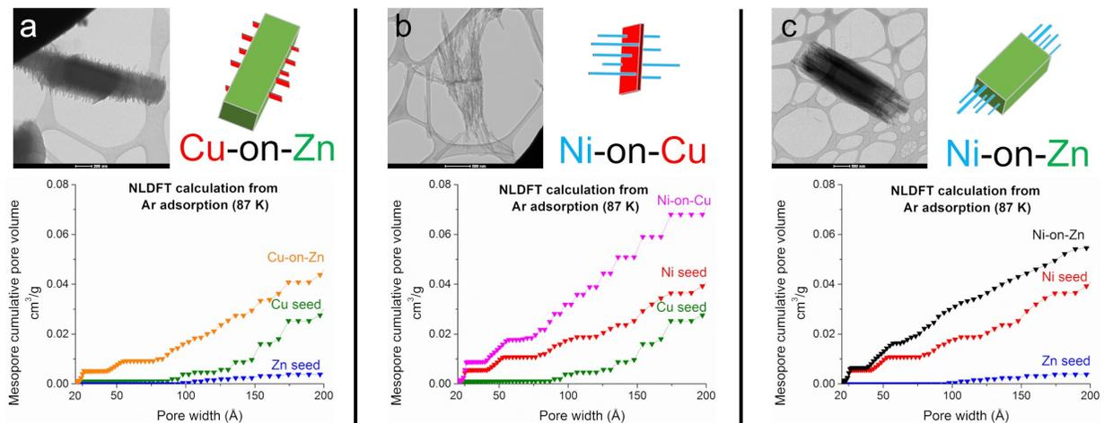
Figure S6. Cumulative pore volume 2-20nm measured by Ar adsorption at 87K for: (a) Cu-on-Zn, Cu and Zn seed, (b) Ni-on-Cu, Ni and Cu seed, (c) Ni-on-Zn, Ni and Zn seed.
