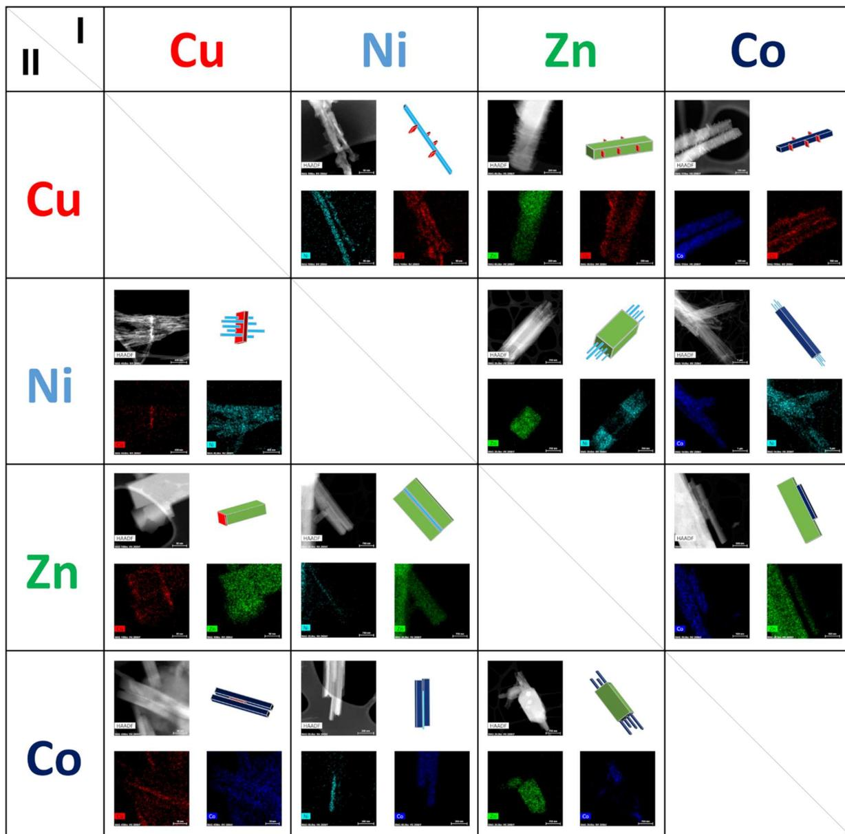
Figure S2. Particle morphology and EDX spectrum images of intergrowth MOFs  $M^{II}_2(ndc)_2(dabco)$  on  $M^I_2(ndc)_2(dabco)$  ( $M^{II}$  and  $M^I = Cu, Zn, Ni, Co$ )
