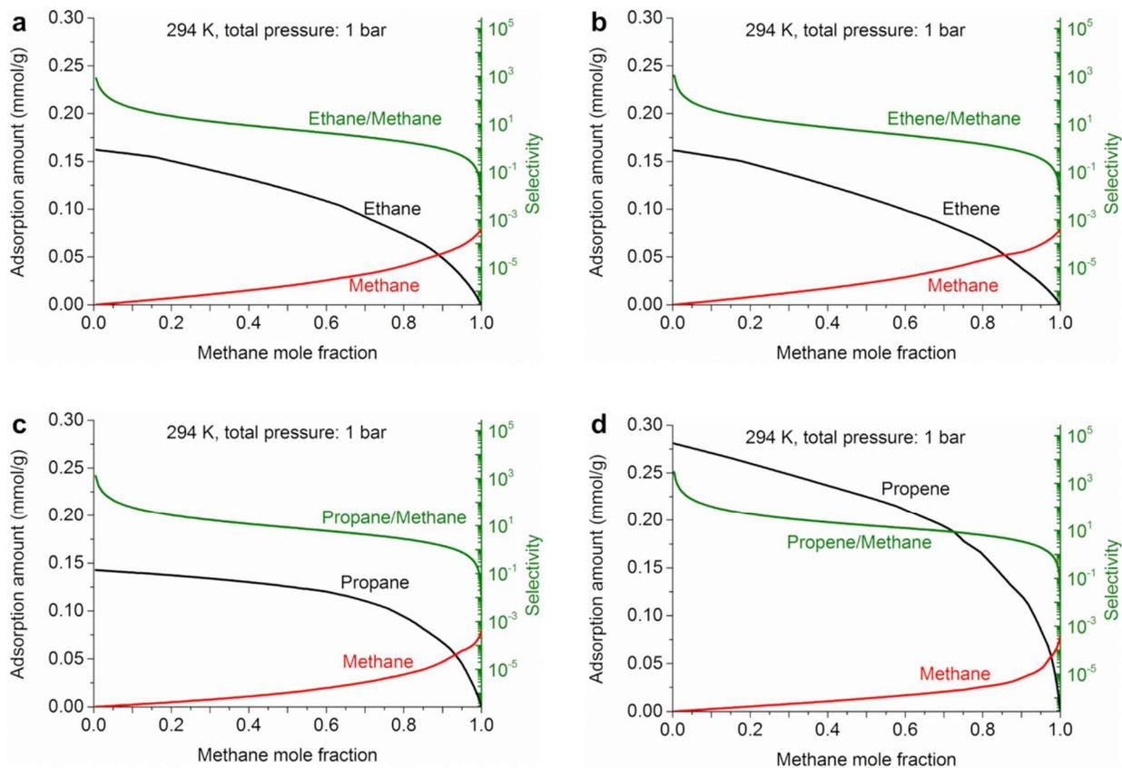
Figure S9. IAST-predicted adsorption amount and selectivity of mixed gases on Cu seed: a). Ethane and methane; b). Ethene and methane; c). Propane and methane; d). Propene and methane
