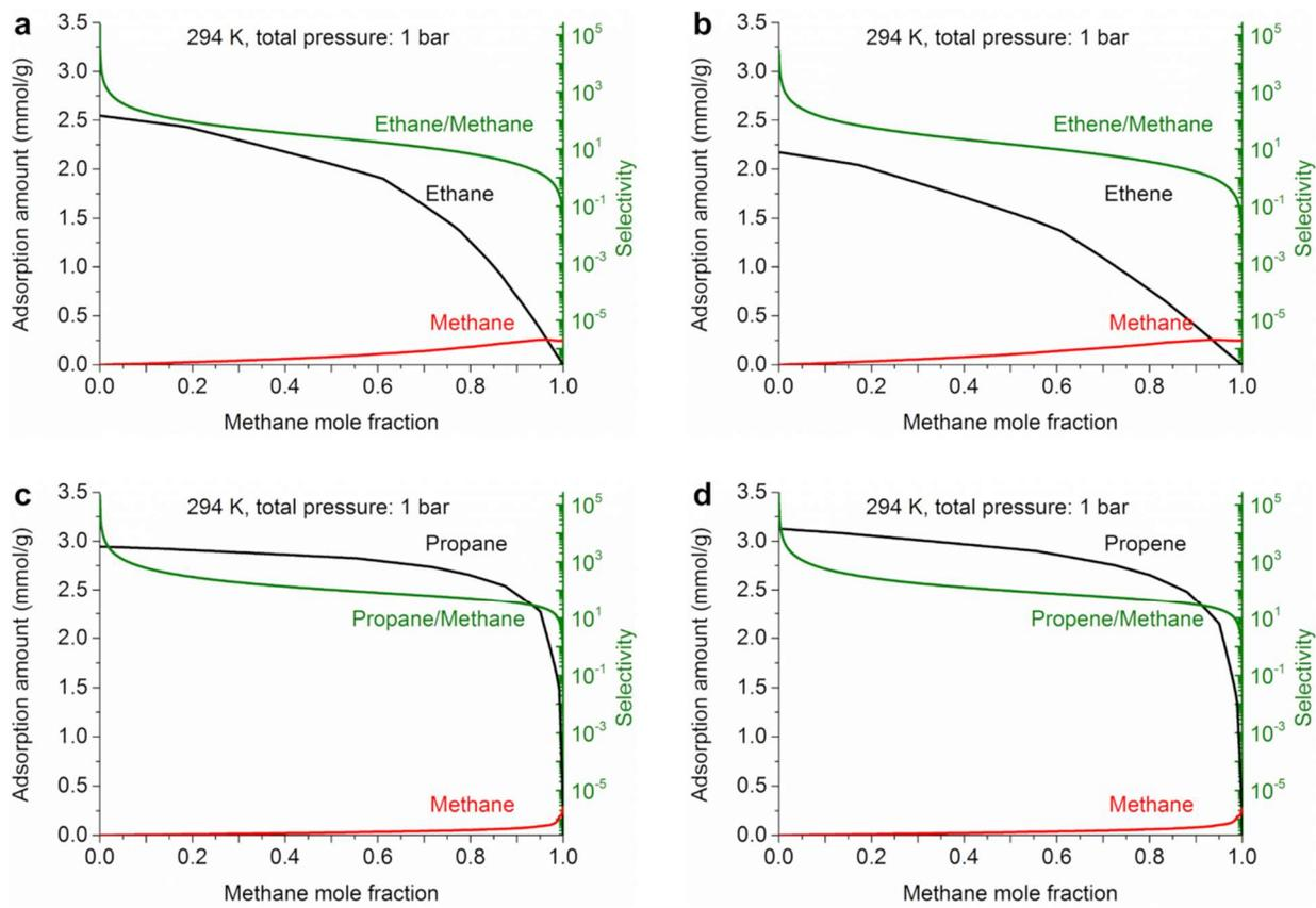
Figure S7. IAST-predicted adsorption amount and selectivity of mixed gases on Ni-on-Cu intergrowth: a). Ethane and methane; b). Ethene and methane; c). Propane and methane; d). Propene and methane
