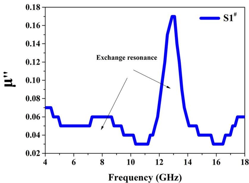
Fig. S10. Frequency dependence of  $\mu''$  for S1<sup>#</sup> in the frequency range of 4-18 GHz.
