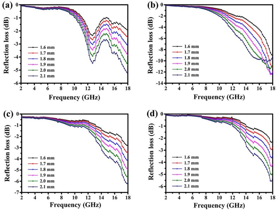
**Fig. S8.** RL curves of M-Co/RGO nanocomposites with different thicknesses in the frequency range 2-18 GHz: (a) S4<sup>#</sup>, (b) S5<sup>#</sup>, (c) S7<sup>#</sup>, (d) S8<sup>#</sup>.
