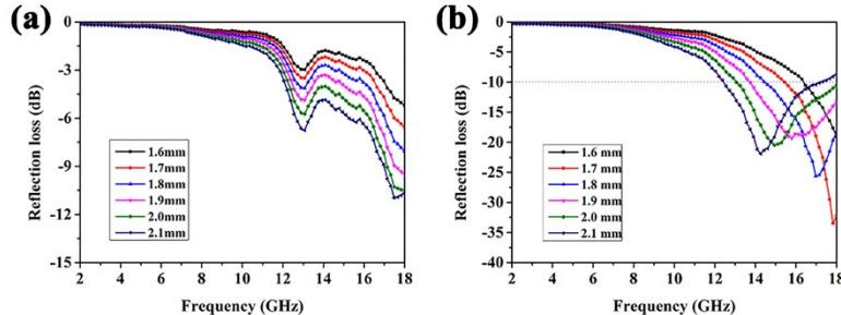
**Fig. S7.** RL curves of M-Co/RGO nanocomposites with different thicknesses in the frequency range 2-18 GHz: (a) S1<sup>#</sup>, (b) S2<sup>#</sup>.
