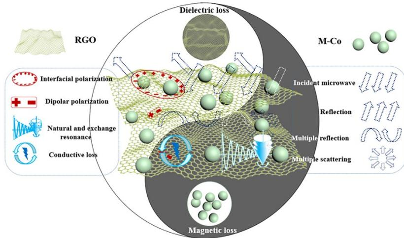
**Fig. S13.** Schematic illustration of microwave absorption mechanism of M-Co/RGO nanocomposites
