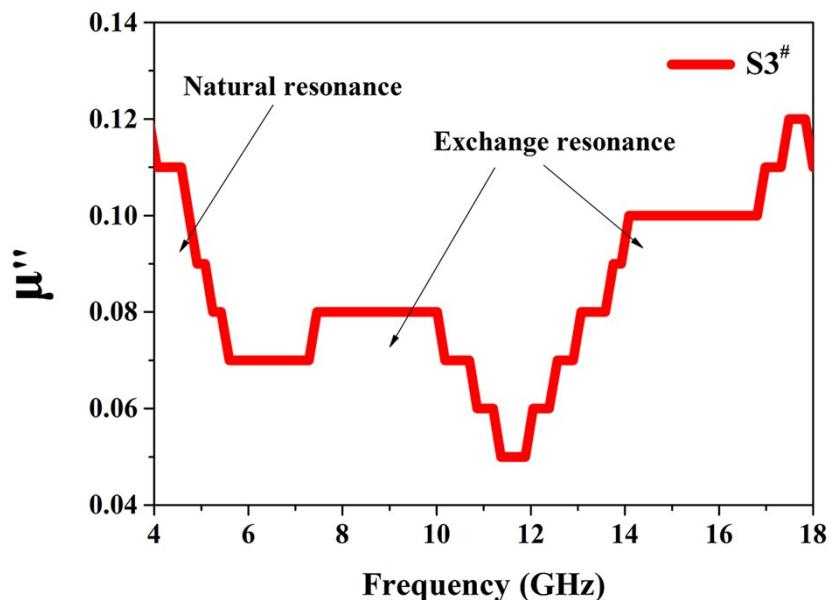
Fig. S11. Frequency dependence of  $\mu$  for S3<sup>#</sup> in the frequency range of 4-18 GHz.
