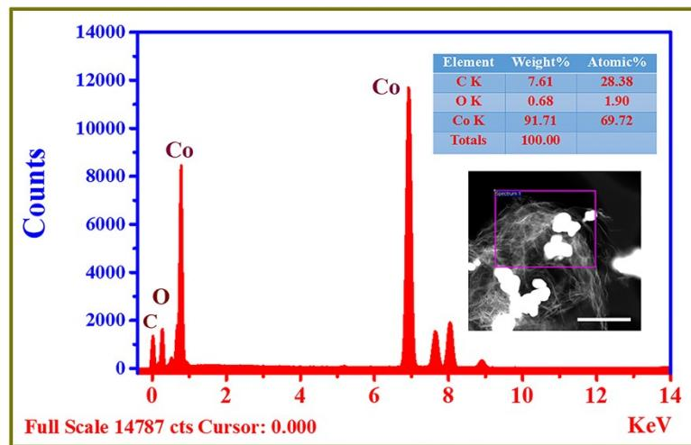
**Fig. S3.** EDS spectra of M-Co/RGO nanocomposites
