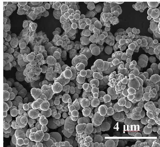
**Fig. S2.** SEM image of M-Co nanoparticles.
