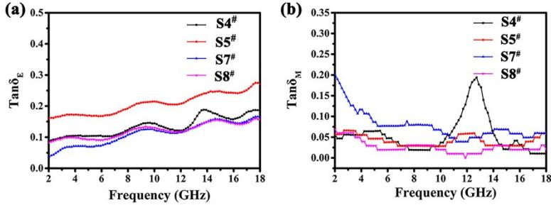
**Fig. S6.** (a)  $\tan\delta_E$  and (b)  $\tan\delta_M$  of S4<sup>#</sup>, S5<sup>#</sup>, S7<sup>#</sup> and S8<sup>#</sup> in the frequency range of 2-18 GH
