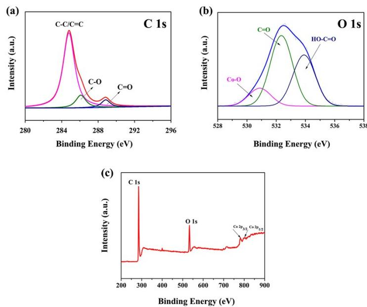
**Fig. S4.** (a) C 1s XPS spectra for M-Co/RGO nanocomposites. (b) O 1s XPS spectra for M-Co/RGO nanocomposites. (c) XPS spectra of the M-Co/RGO nanocomposites.
