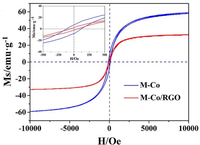
**Fig. S9.** Magnetic hysteresis loop of M-Co nanoparticles and M-Co/RGO nanocomposites (S3<sup>#</sup>) at 300 K (the inset is amplified views of hysteresis loops at low applied fields).
