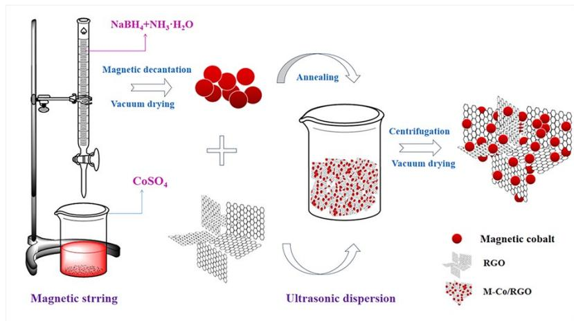
**Fig. S1.** Schematic illustration of the formation process for M-Co/RGO nanocomposites.
