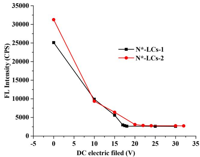
**Fig. S12** PL Intensity-voltage curves of N\*-LCs-1 (Guest, 1.0wt% M1) and N\*-LCs-2 (Guest, 1.0wt% M2) on ITO glass LCDs ( $\lambda_{ex} = 360$  nm, DC 10-32 V, 15s). (cells: homeotropic surface anchoring conditions).
