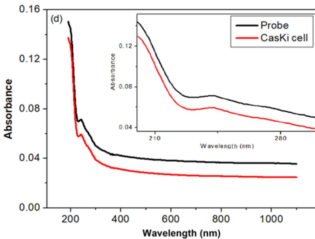
**Figure S2.** Absorbance spectra for Chi/CNT/cpHPV16Probe (---) exposed to (a) JHU28 cell solution, (b) JHU12 cell solution, (c) PCA3 DNA solution, (d) CasKi cell solution, (e) SiHa cell solution (---). All solutions were prepared in PBS.
