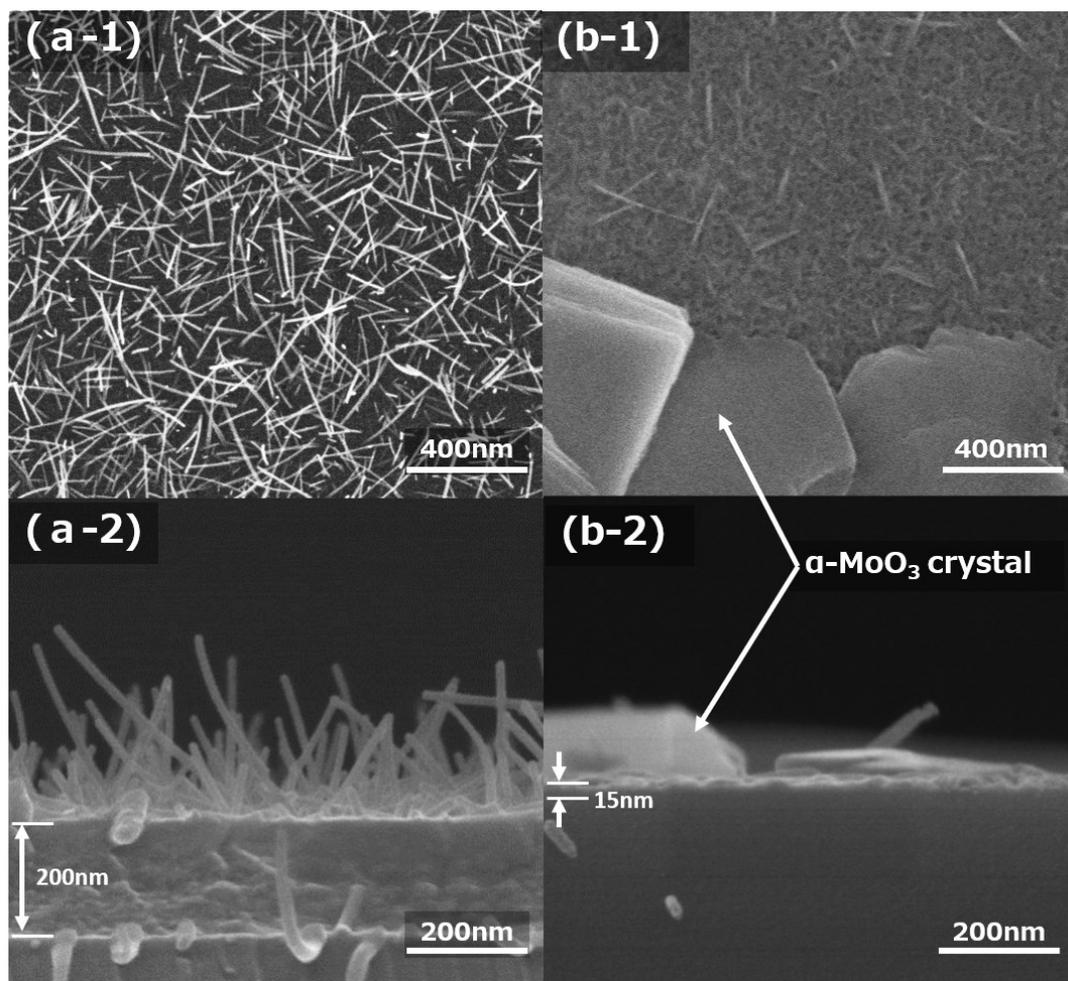
Figure SI-1 The top view / cross sectional FE-SEM Images of  $\alpha$ -MoO<sub>3</sub> nanorods growth from seed layers after sintering at 673K for (a) 15min and (b) 40min, when as deposited thickness after spin coating are thin. (The thickness after drying at 373K is about 1 $\mu$ m).
