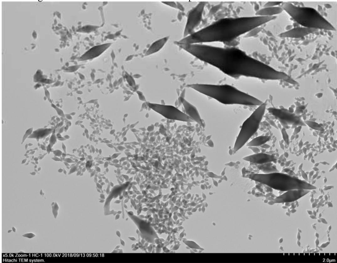
**Fig. S32.** TEM image of SLN-5-Flu after the solvent evaporation.
