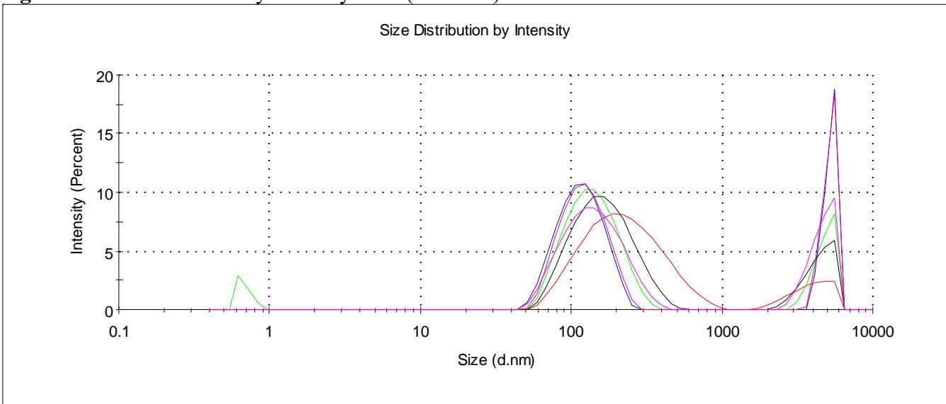
**Fig. S76.** Size distribution by intensity for **4** ( $1 \times 10^{-3}$ M) in  $\text{CHCl}_3$ .
