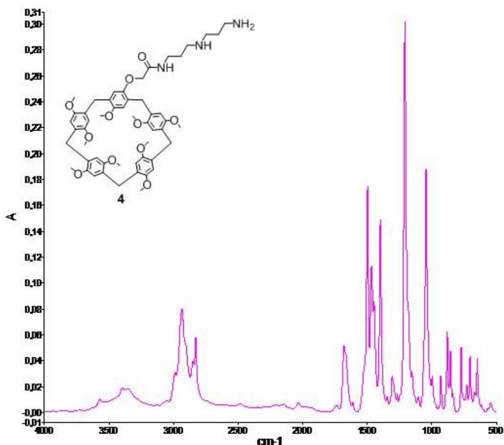
**Fig. S11.** IR spectrum of 4-N-[2-(2-aminopropylamino)propyl]acetamidoxy-8,14,18,23,26,28,31,32,35-nonamethoxypillar[5]arene (**4**).
