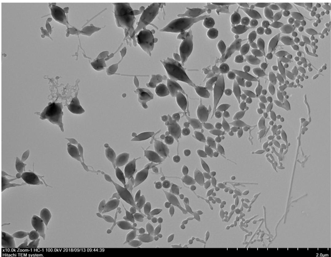
**Fig. S29.** TEM image of SLN-4-Flu after the solvent evaporation.
