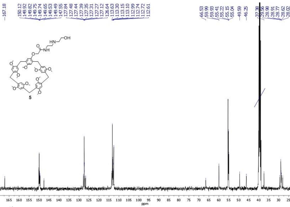
**Fig. S6.**  $^{13}\text{C}$  NMR spectrum of 4-N-[2-(2-aminoethylhydroxy)ethyl]acetamidoxy-8,14,18,23,26,28,31,32,35-nonamethoxypillar[5]arene (**5**), DMSO-*d*<sub>6</sub>, 298 K, 100 MHz.
