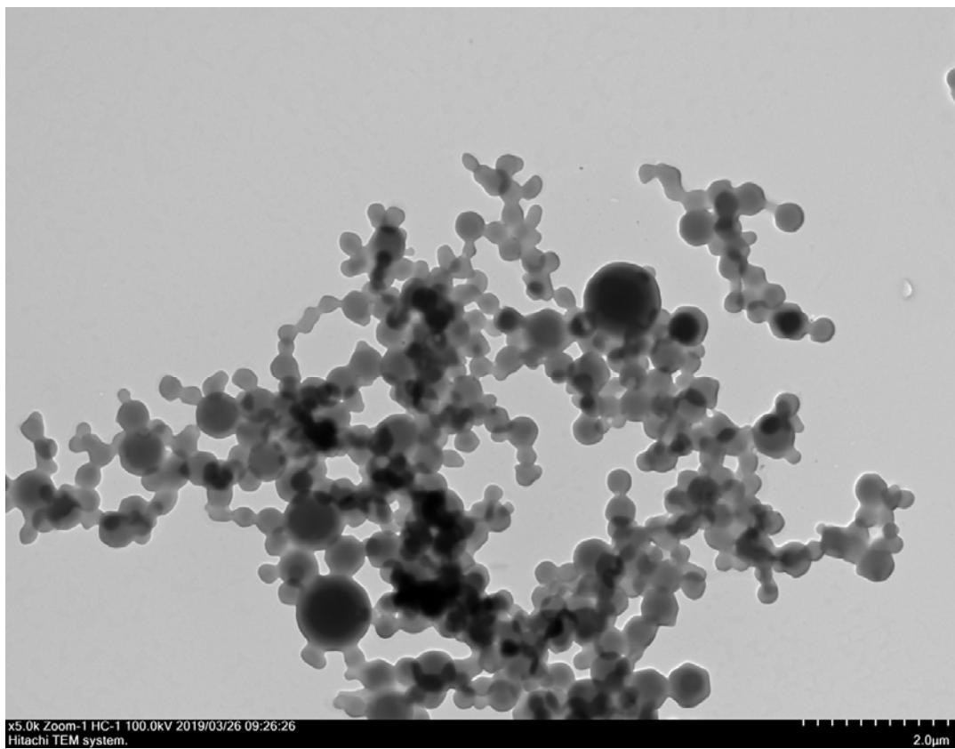
**Fig. S22.** TEM image of SLN-6 after the solvent evaporation.
