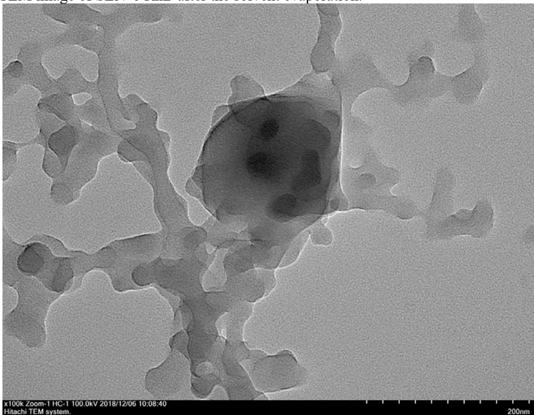
**Fig. S44.** TEM image of SLN-4-RhB after the solvent evaporation.
