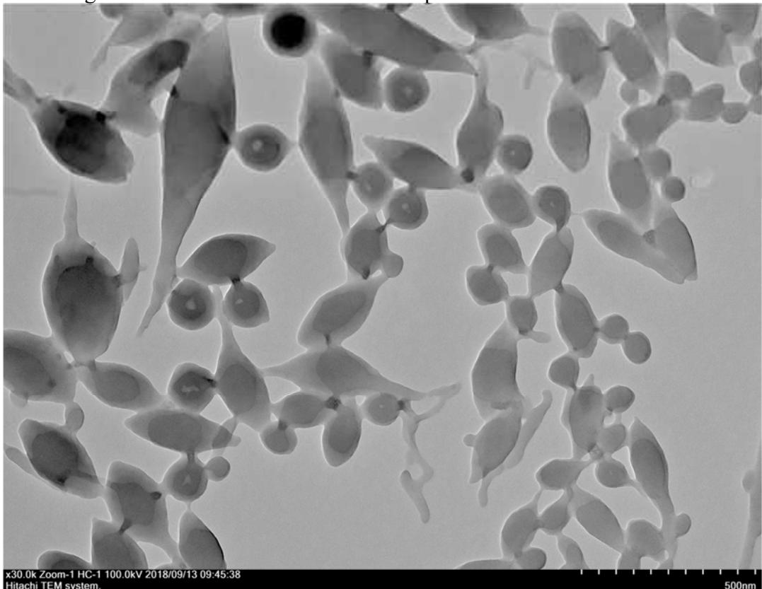
**Fig. S30.** TEM image of SLN-4-Flu after the solvent evaporation.
