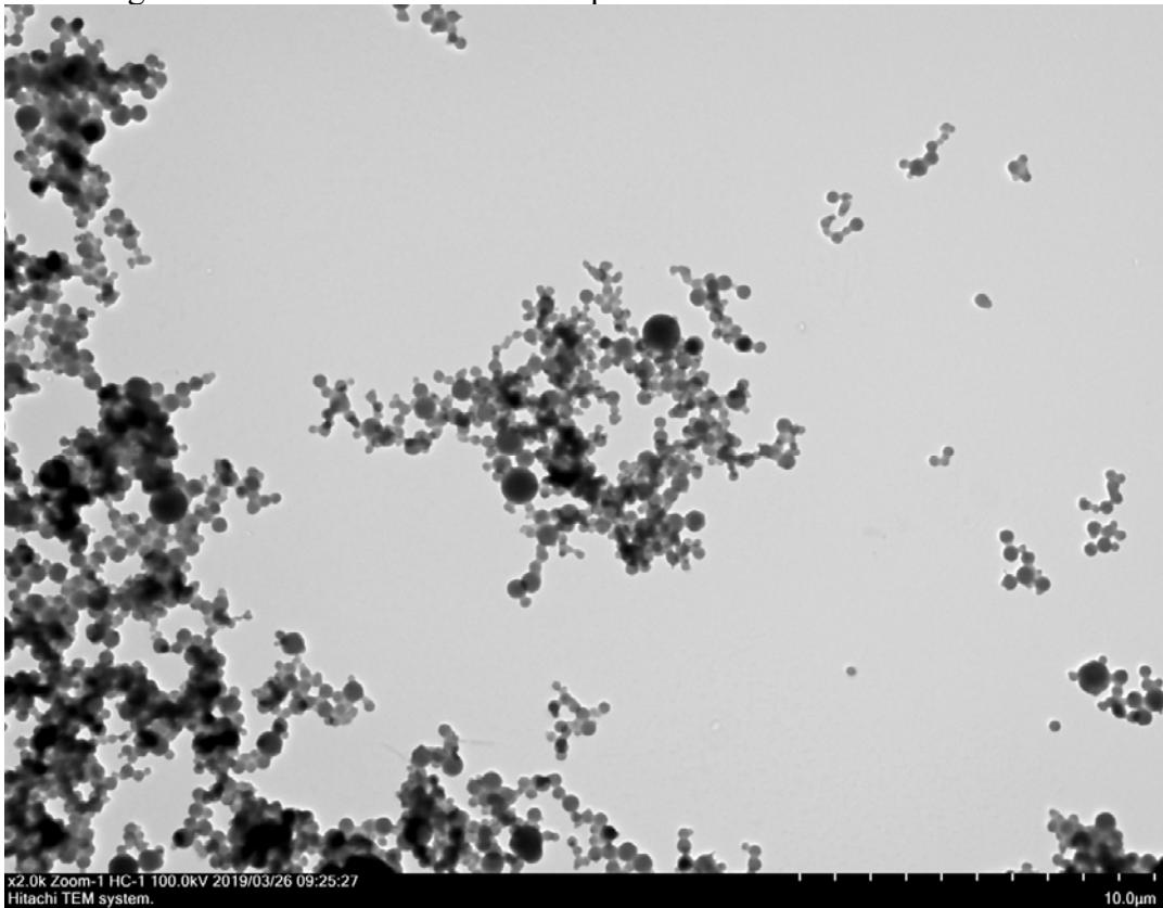
**Fig. S21.** TEM image of SLN-6 after the solvent evaporation.
