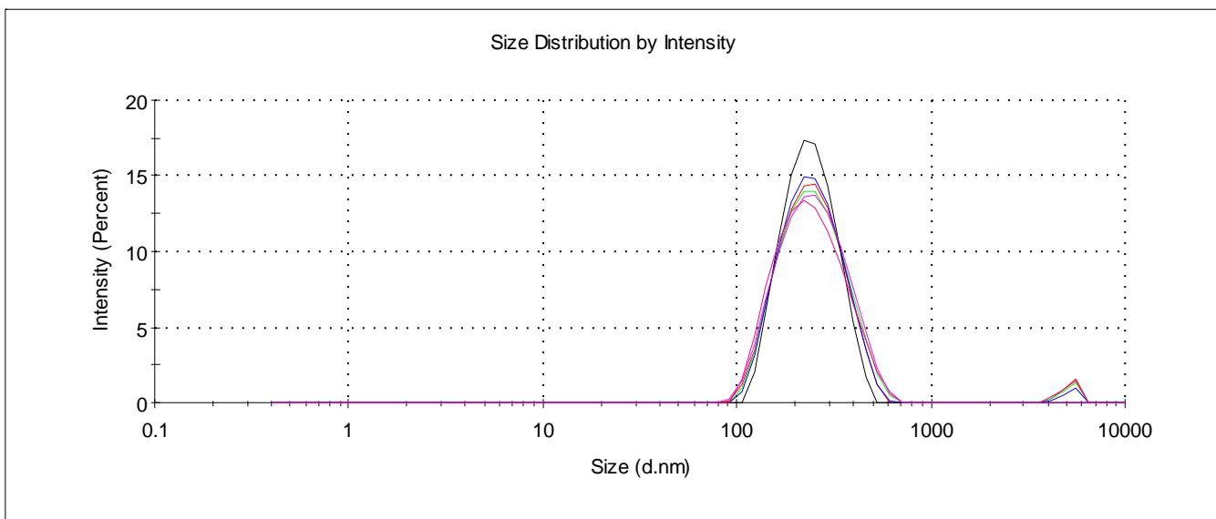
**Fig. S104.** Size distribution of the particles by intensity for SLN-6-RhB ( $3 \times 10^{-5}$ M) in water.
