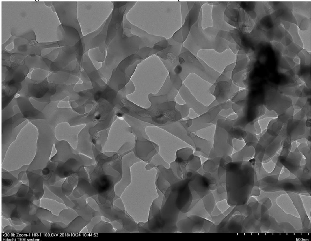
**Fig. S48.** TEM image of SLN-5-RhB after the solvent evaporation.
