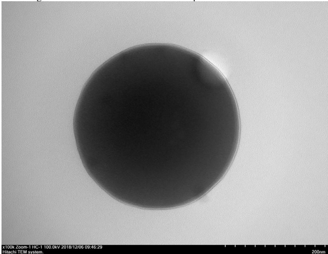
**Fig. S67.** TEM image of SLN-6-Rh6G after the solvent evaporation.
