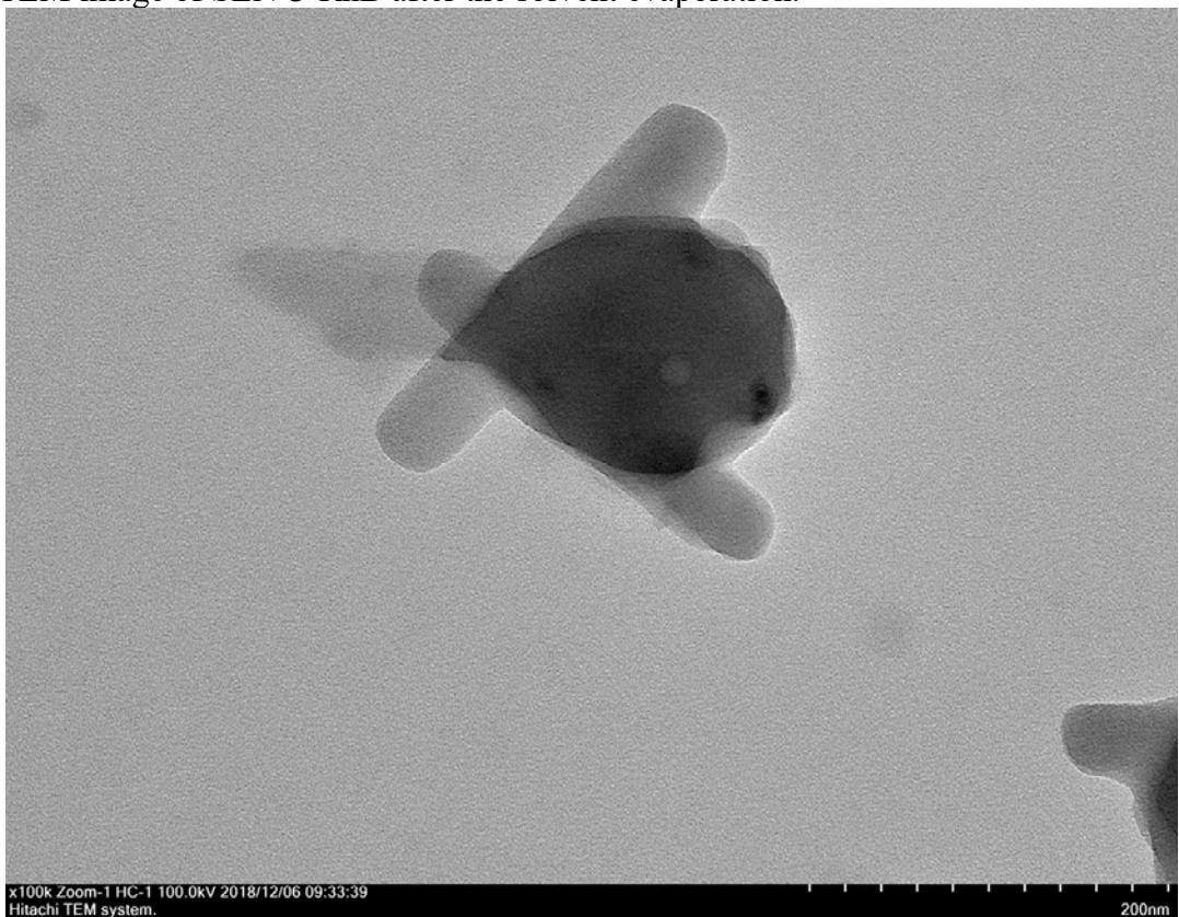
**Fig. S40.** TEM image of SLN-3-RhB after the solvent evaporation.
