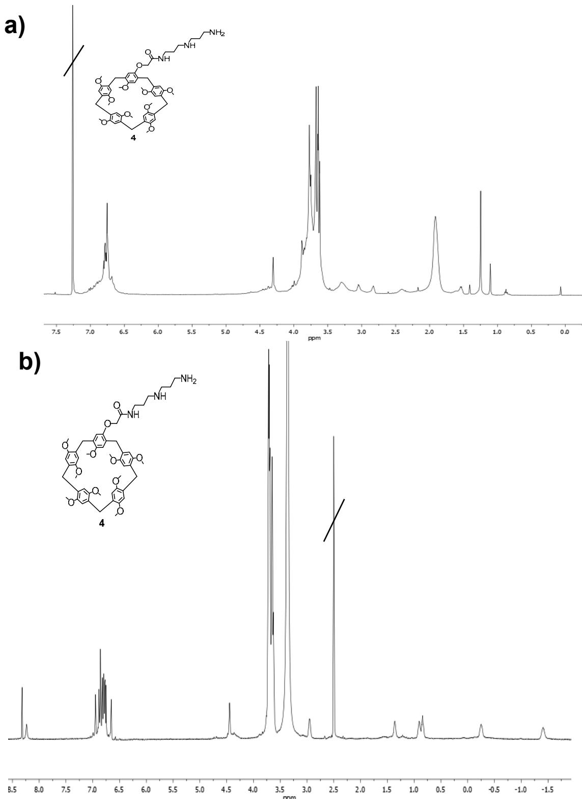
**Fig. S1.**  $^1\text{H}$  NMR spectrum of 4-N-[2-(2-aminopropylamino)propyl]acetamidoxy-8,14,18,23,26,28,31,32,35-nonamethoxypillar[5]arene (**4**): a).  $\text{CDCl}_3$ , 298 K, 400 MHz; b).  $\text{DMSO}-d_6$ , 298 K, 400 MHz.
