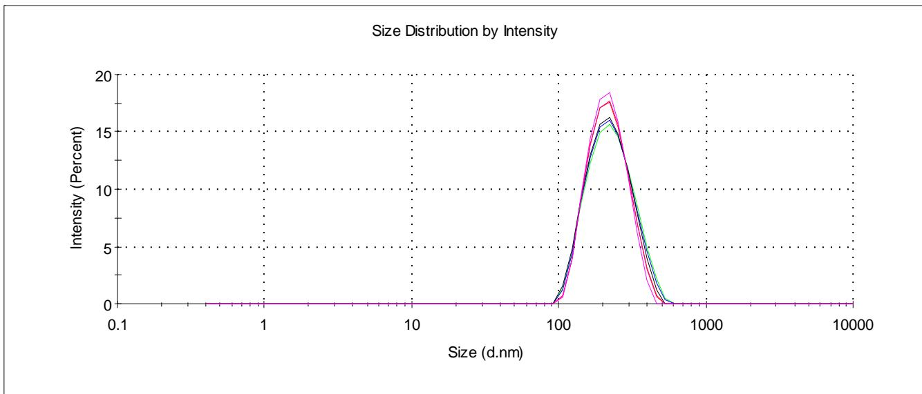
**Fig. S92.** Size distribution of the particles by intensity for SLN-4-Flu ( $3 \times 10^{-5}$ M) in water.
