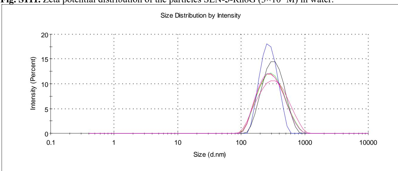
**Fig. S112.** Size distribution of the particles by intensity for SLN-6-Rh6G ( $3 \times 10^{-5}$ M) in water.
