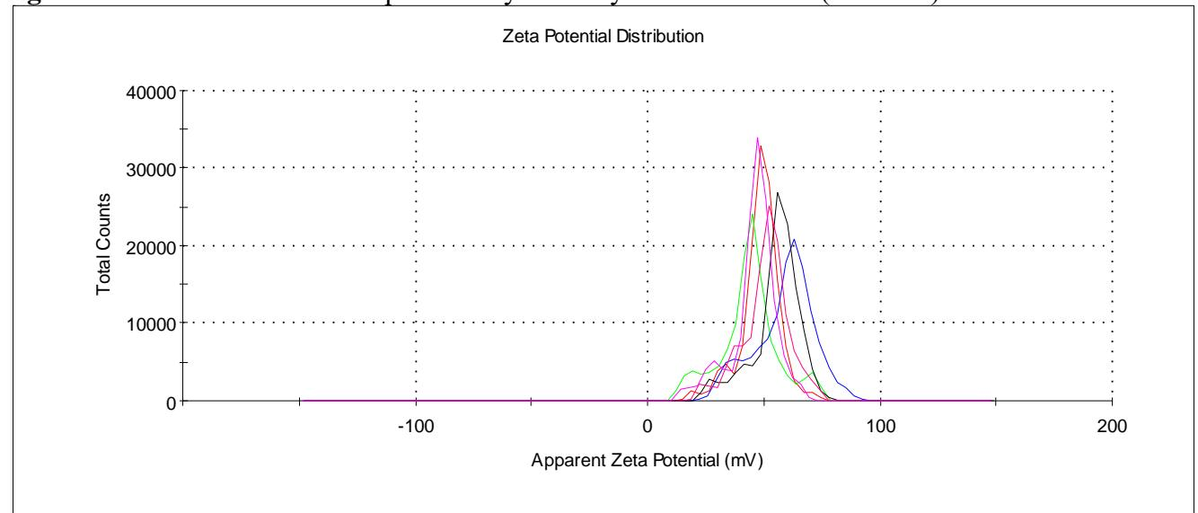
**Fig. S99.** Zeta potential distribution of the particles SLN-3-RhB ( $3 \times 10^{-5}$ M) in water.
