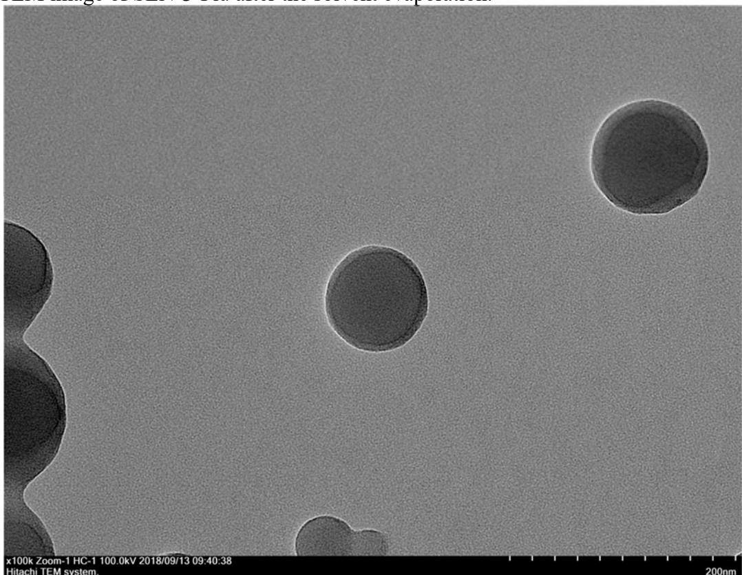
**Fig. S28.** TEM image of SLN-3-Flu after the solvent evaporation.
