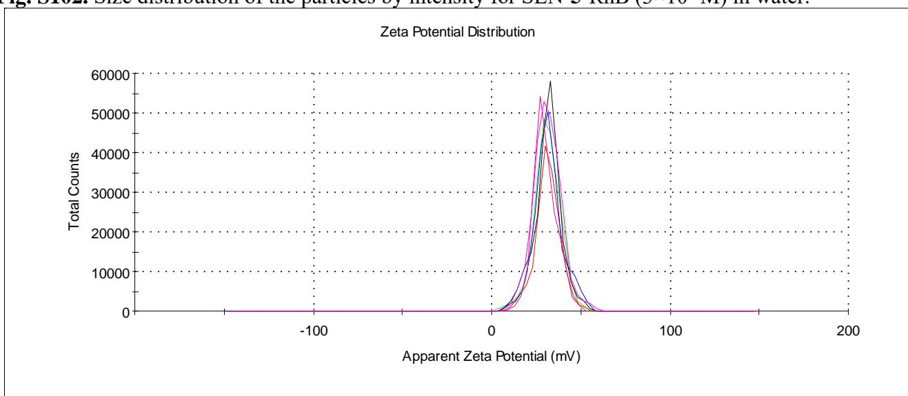
**Fig. S103.** Zeta potential distribution of the particles SLN-5-RhB ( $3 \times 10^{-5}$ M) in water.
