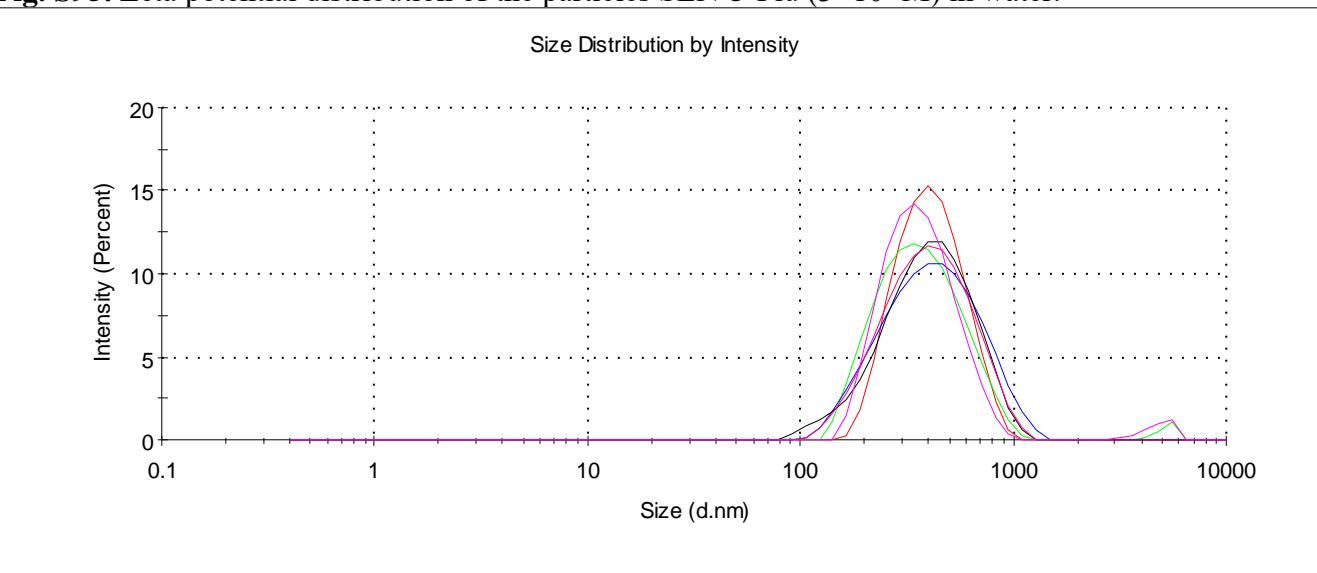
**Fig. S96.** Size distribution of the particles by intensity for SLN-6-Flu ( $3 \times 10^{-5}$ M) in water.
