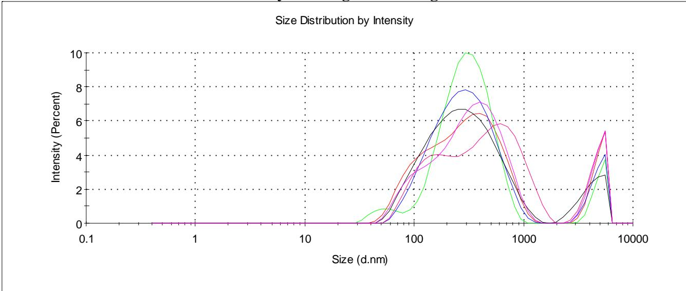
**Fig. S74.** Size distribution by intensity for **3** ( $1 \times 10^{-3}$ M) in  $\text{CHCl}_3$ .
