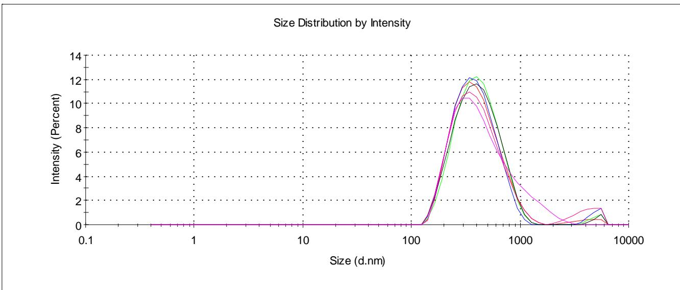
**Fig. S86.** Size distribution of the particles by intensity for SLN-5 ( $3 \times 10^{-5}$ M) in water.
