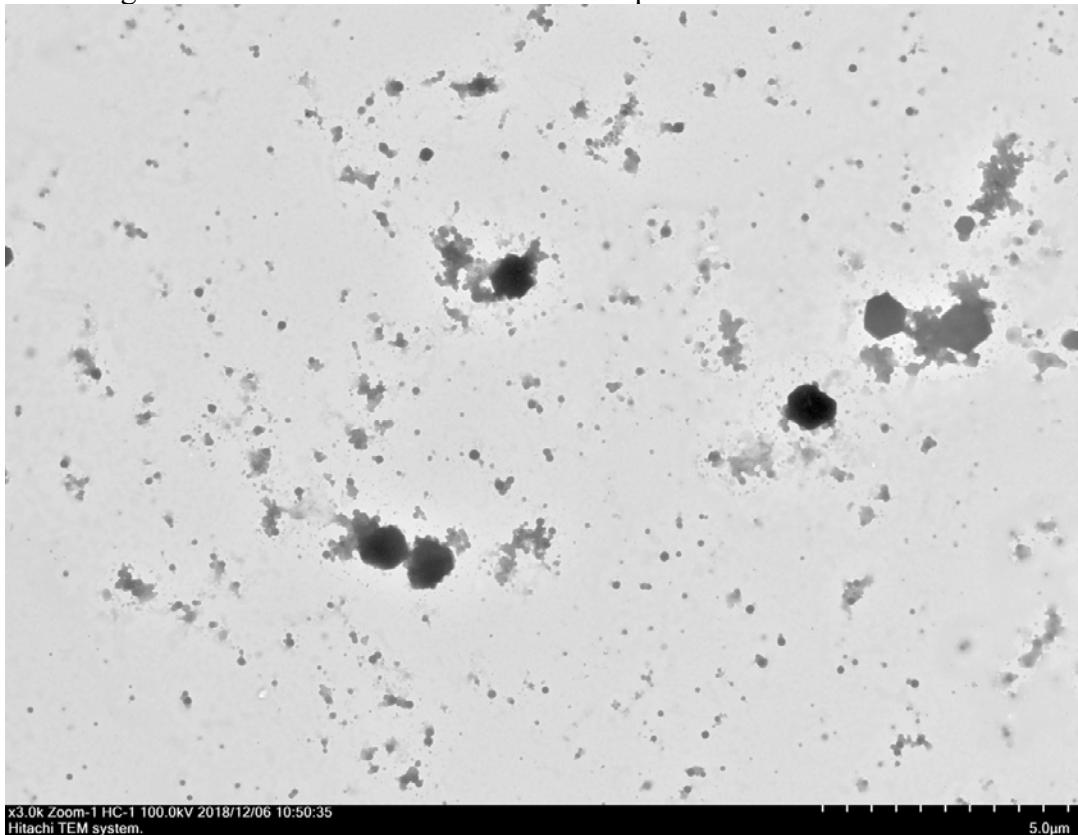
**Fig. S57.** TEM image of SLN-4-Rh6G after the solvent evaporation.
