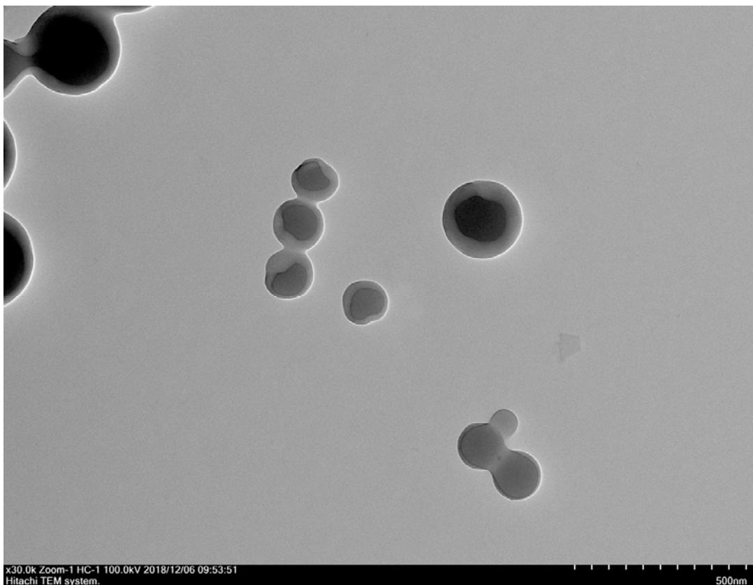
**Fig. S66.** TEM image of SLN-6-Rh6G after the solvent evaporation.
