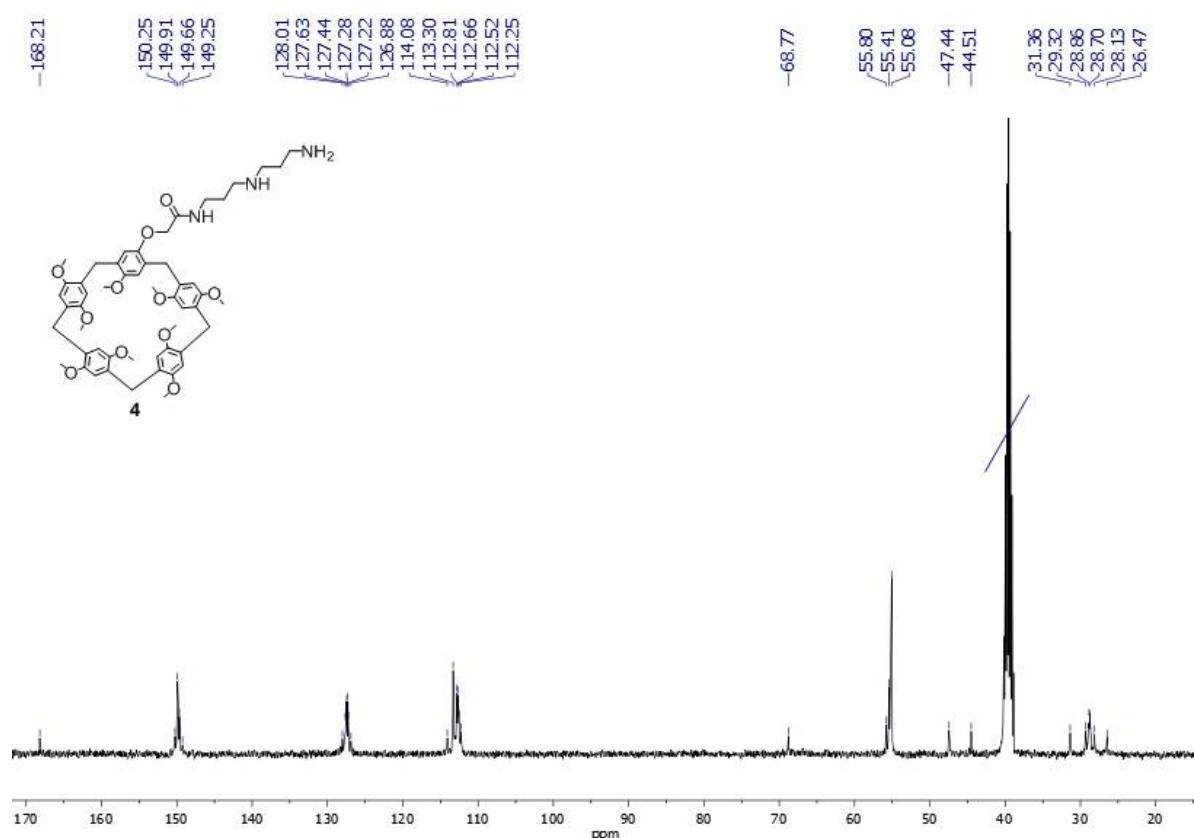
**Fig. S5.**  $^{13}\text{C}$  NMR spectrum of 4-N-[2-(2-aminopropylamino)propyl]acetamidoxy-8,14,18,23,26,28,31,32,35-nonamethoxypillar[5]arene (**4**), DMSO- $d_6$ , 298 K, 100 MHz.
