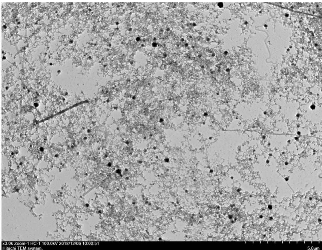
**Fig. S41.** TEM image of SLN-4-RhB after the solvent evaporation.
