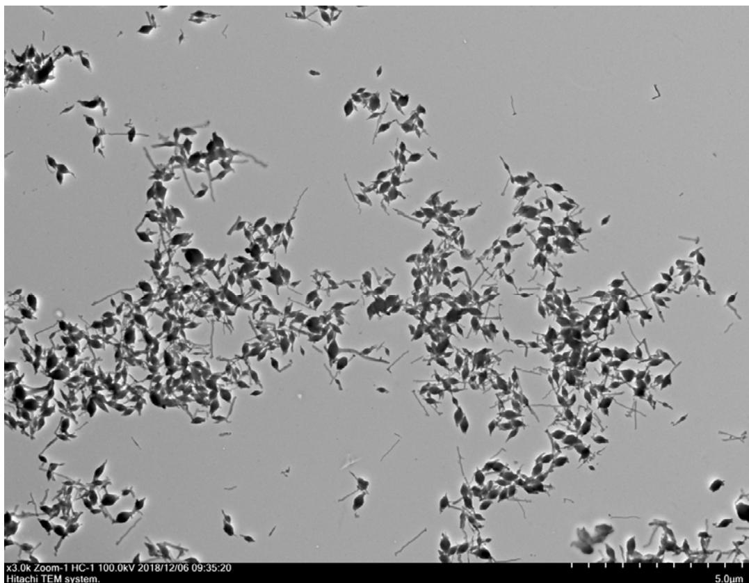
**Fig. S60.** TEM image of SLN-5-Rh6G after the solvent evaporation.
