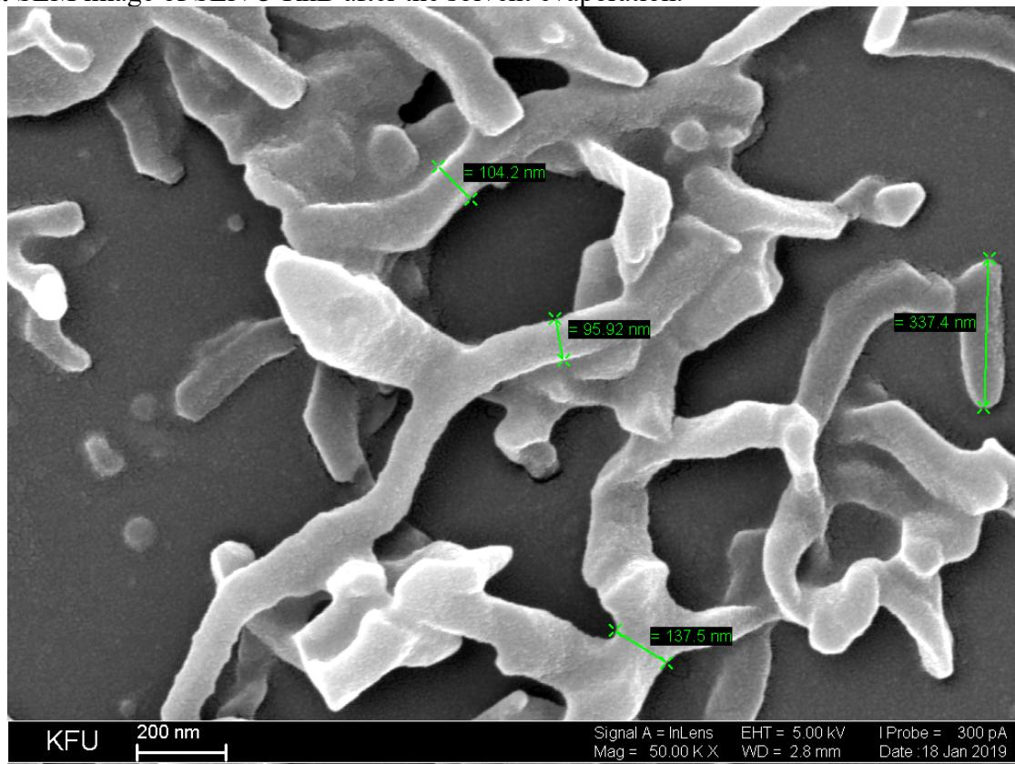
**Fig. S73.** SEM image of SLN-5-RhB after the solvent evaporation.
