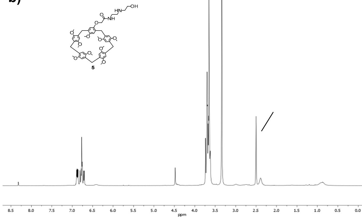
**Fig. S2.** <sup>1</sup>H NMR spectrum of 4-N-[2-(2-aminoethylhydroxy)ethyl]acetamidoxy-8,14,18,23,26,28,31,32,35-nonamethoxypillar[5]arene (**5**): a).  $\text{CDCl}_3$ , 298 K, 400 MHz; b).  $\text{DMSO}-d_6$ , 298 K, 400 MHz.
