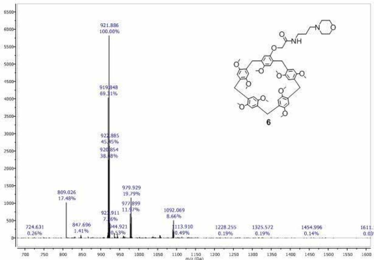
**Fig. S10.** Mass spectrum (MALDI-TOF, 4-nitroaniline matrix) of 4-N-[2-(2-aminomorpholine)propyl]acetamidoxy-8,14,18,23,26,28,31,32,35-nonamethoxypillar[5]arene (**6**).
