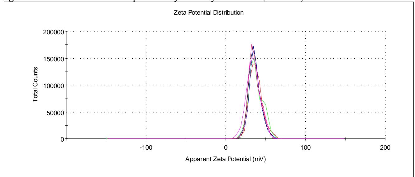
**Fig. S87.** Zeta potential distribution of the particles SLN-5 ( $3 \times 10^{-5}$ M) in water.
