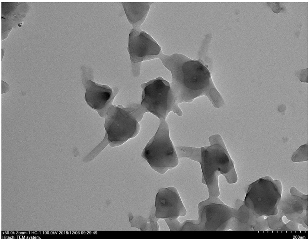
**Fig. S39.** TEM image of SLN-3-RhB after the solvent evaporation.
