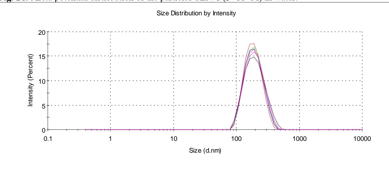
**Fig. S90.** Size distribution of the particles by intensity for SLN-3-Flu ( $3 \times 10^{-5}$ M) in water.
