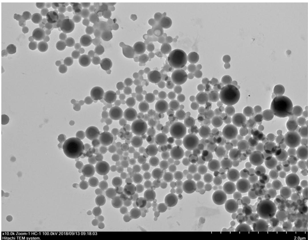
**Fig. S35.** TEM image of SLN-6-Flu after the solvent evaporation.
