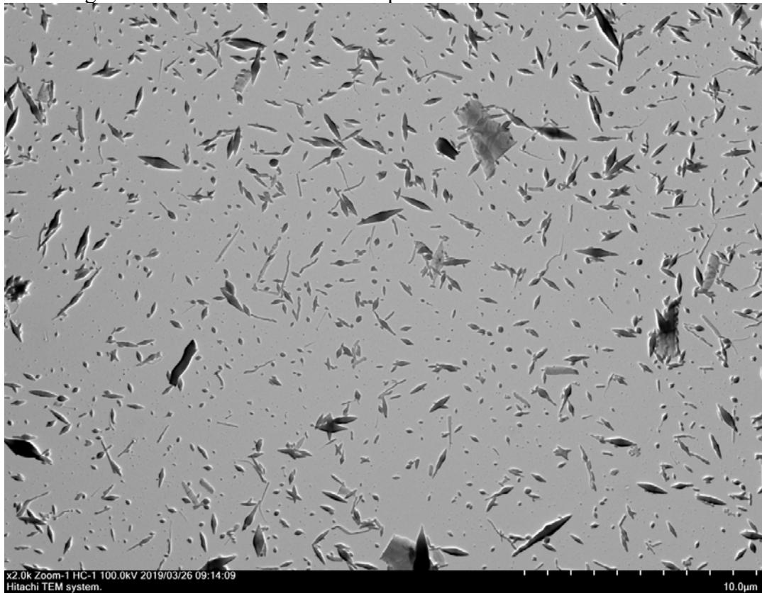
**Fig. S17.** TEM image of SLN-5 after the solvent evaporation.
