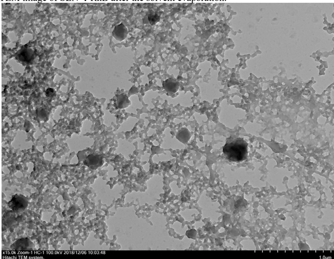
**Fig. S42.** TEM image of SLN-4-RhB after the solvent evaporation.
