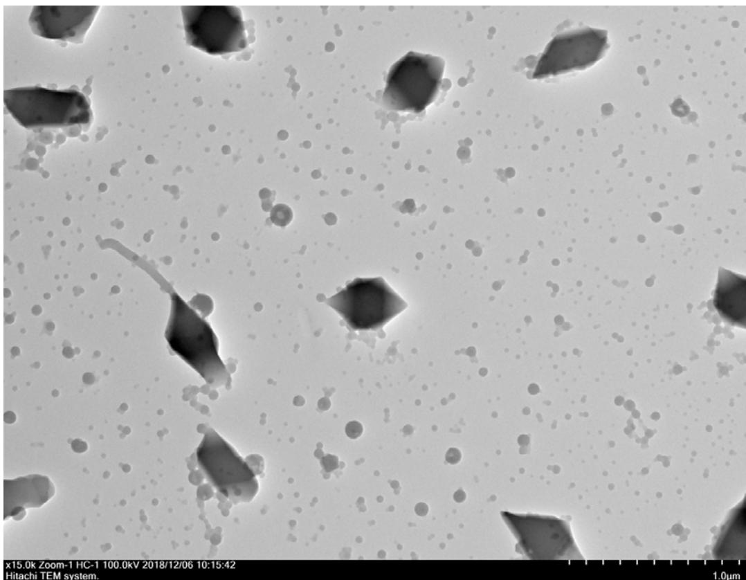
**Fig. S56.** TEM image of SLN-3-Rh6G after the solvent evaporation.
