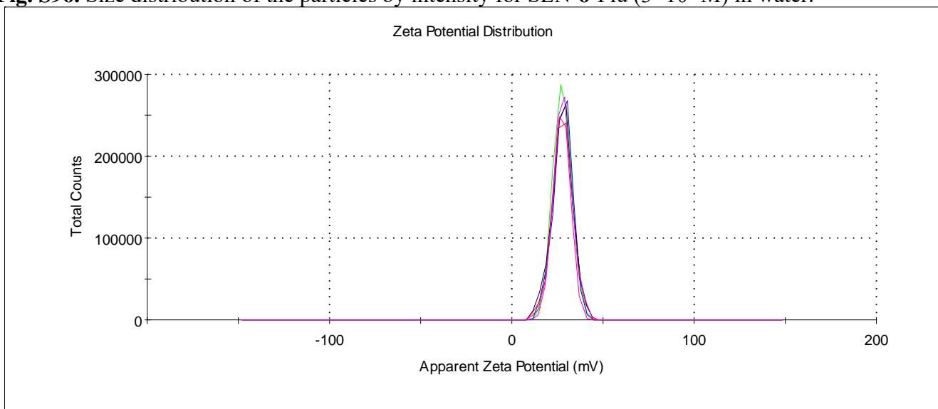
**Fig. S97.** Zeta potential distribution of the particles SLN-6-Flu ( $3 \times 10^{-5}$ M) in water.
