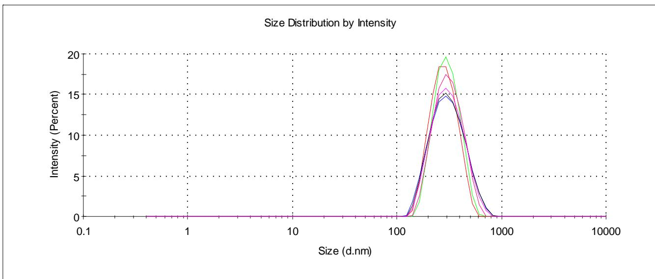
**Fig. S110.** Size distribution of the particles by intensity for SLN-5-Rh6G ( $3 \times 10^{-5}$ M) in water.
