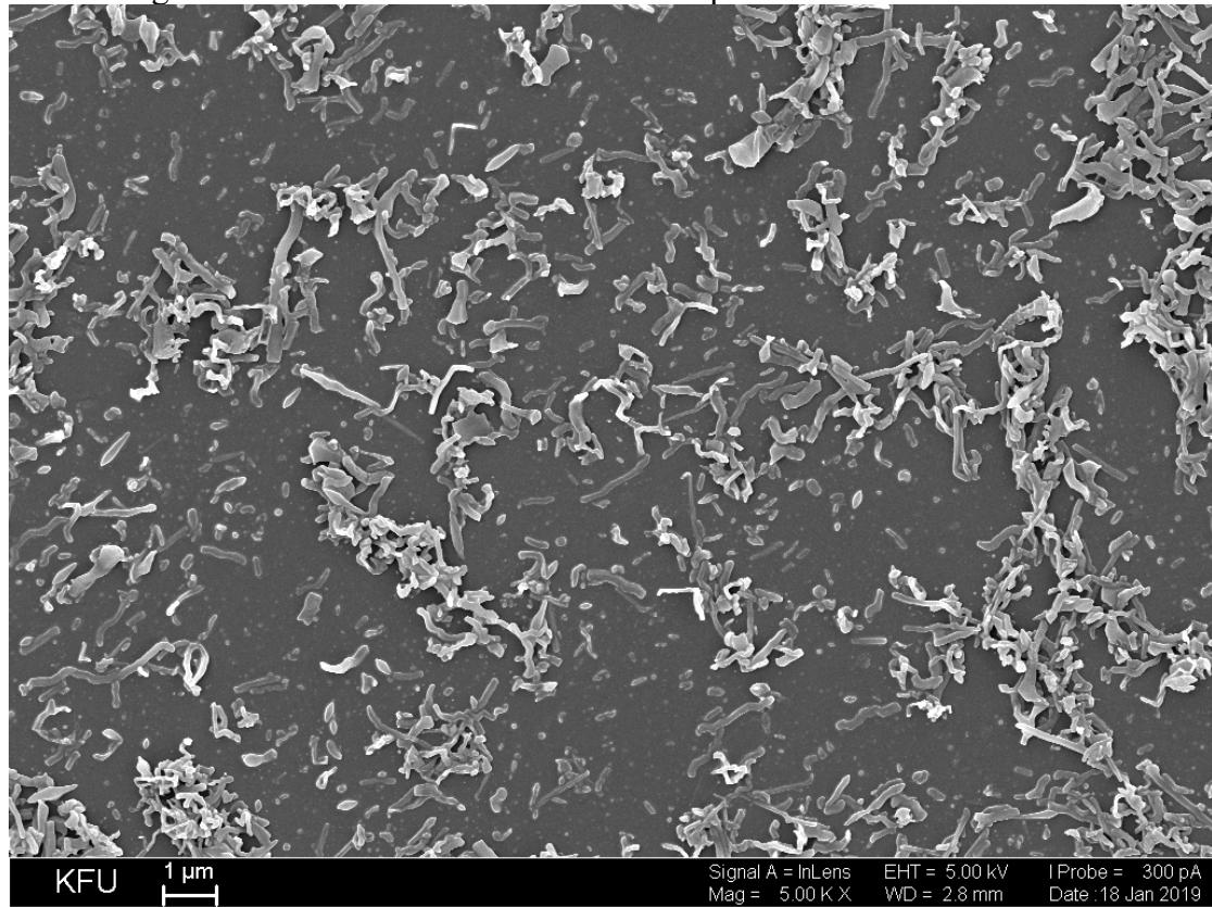
**Fig. S71.** SEM image of SLN-5-RhB after the solvent evaporation.
