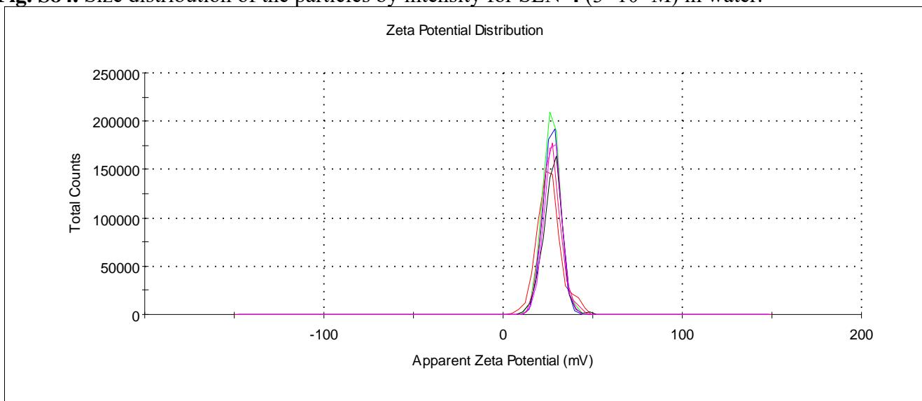
**Fig. S85.** Zeta potential distribution of the particles SLN-4 ( $3 \times 10^{-5}$ M) in water.
