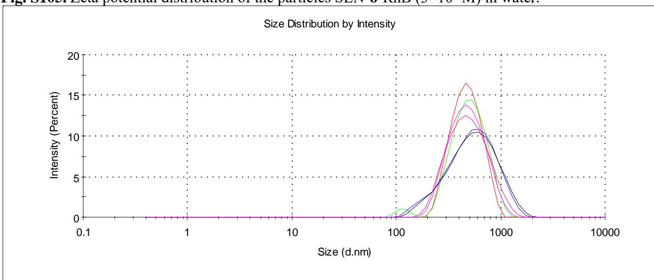
**Fig. S106.** Size distribution of the particles by intensity for SLN-3-Rh6G ( $3 \times 10^{-5}$ M) in water.
