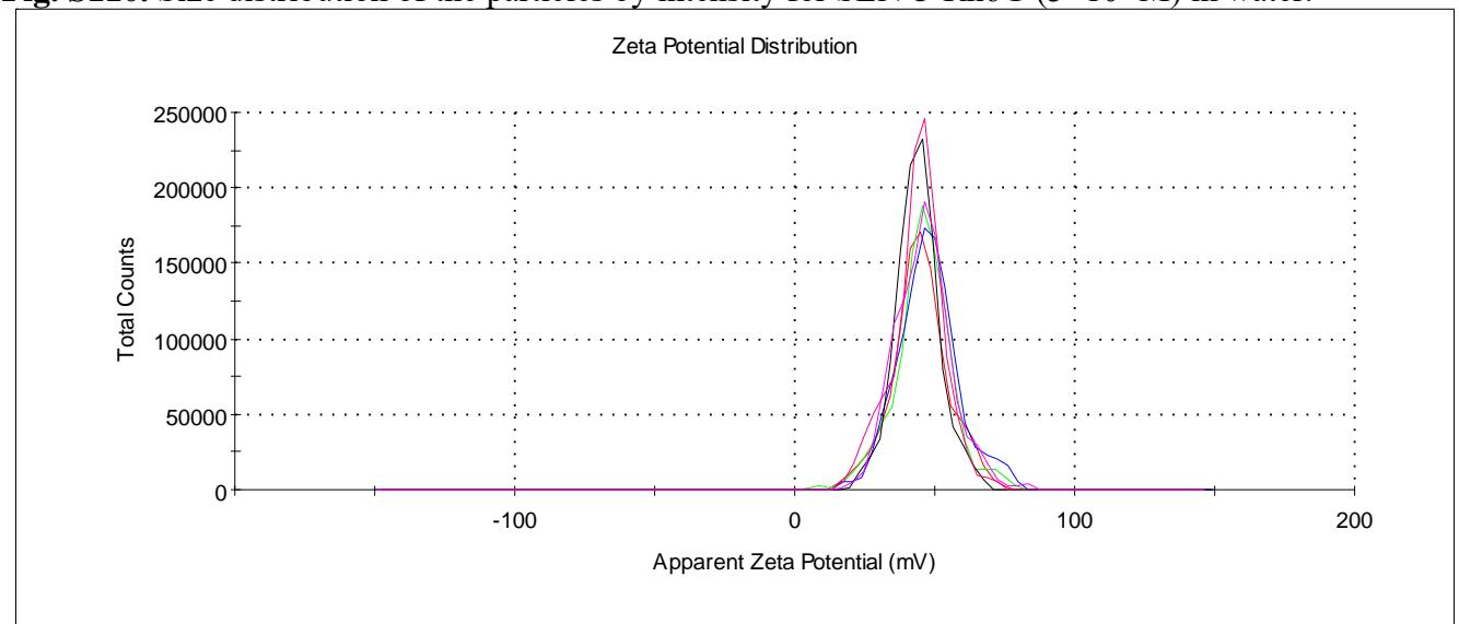
**Fig. S111.** Zeta potential distribution of the particles SLN-5-Rh6G ( $3 \times 10^{-5}$ M) in water.
