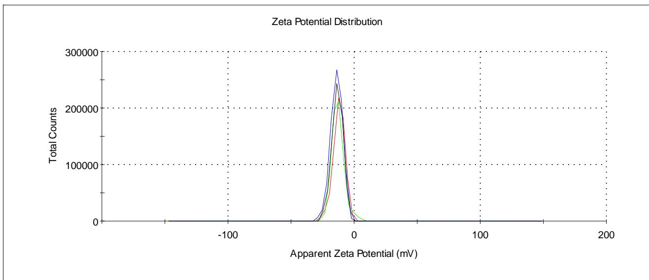
**Fig. S89.** Zeta potential distribution of the particles SLN-6 ( $3 \times 10^{-5}$ M) in water.
