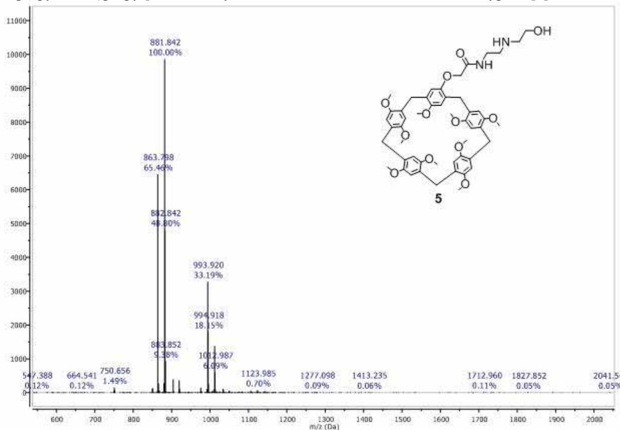
**Fig. S9.** Mass spectrum (MALDI-TOF, 4-nitroaniline matrix) of 4-N-[2-(2-aminoethylhydroxy)ethyl]acetamidoxy-8,14,18,23,26,28,31,32,35-nonamethoxypillar[5]arene (**5**).
