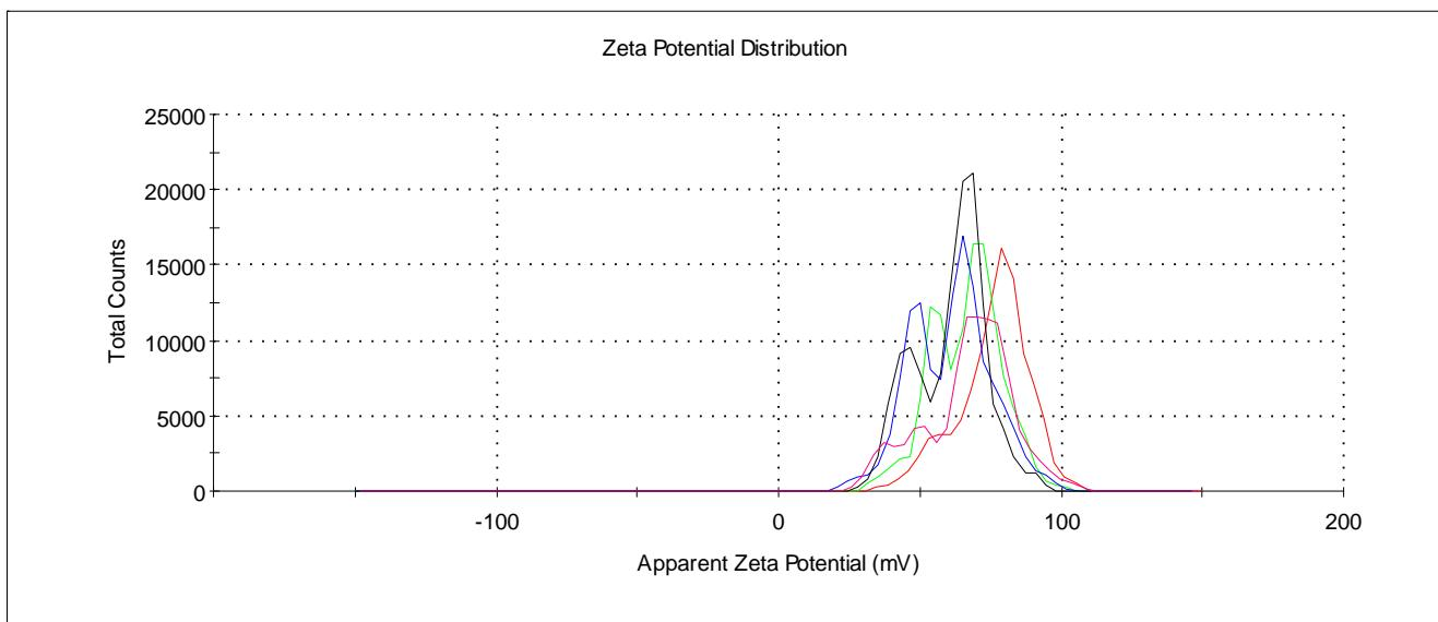
**Fig. S101.** Zeta potential distribution of the particles SLN-4-RhB ( $3 \times 10^{-5}$ M) in water.
