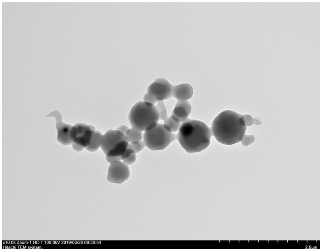
**Fig. S24.** TEM image of SLN-6 after the solvent evaporation.
