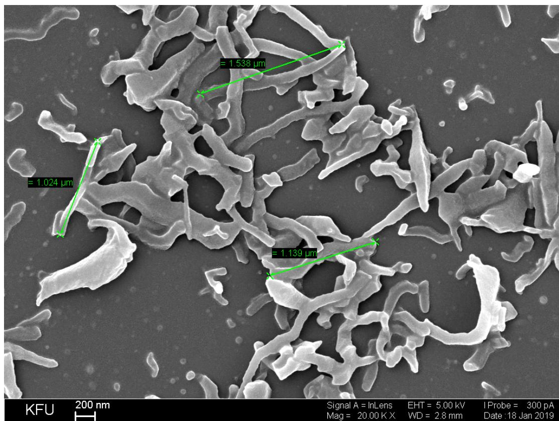
**Fig. S72.** SEM image of SLN-5-RhB after the solvent evaporation.
