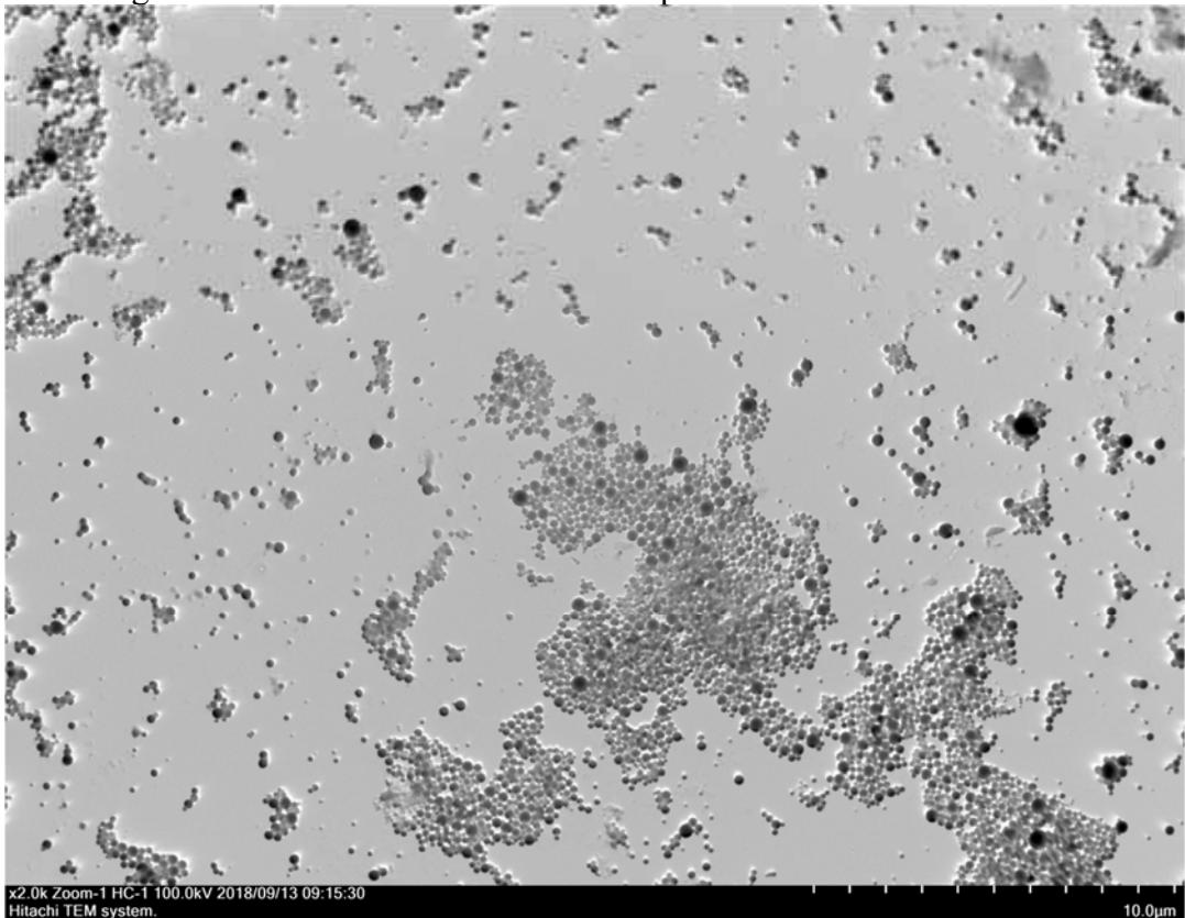
**Fig. S34.** TEM image of SLN-6-Flu after the solvent evaporation.
