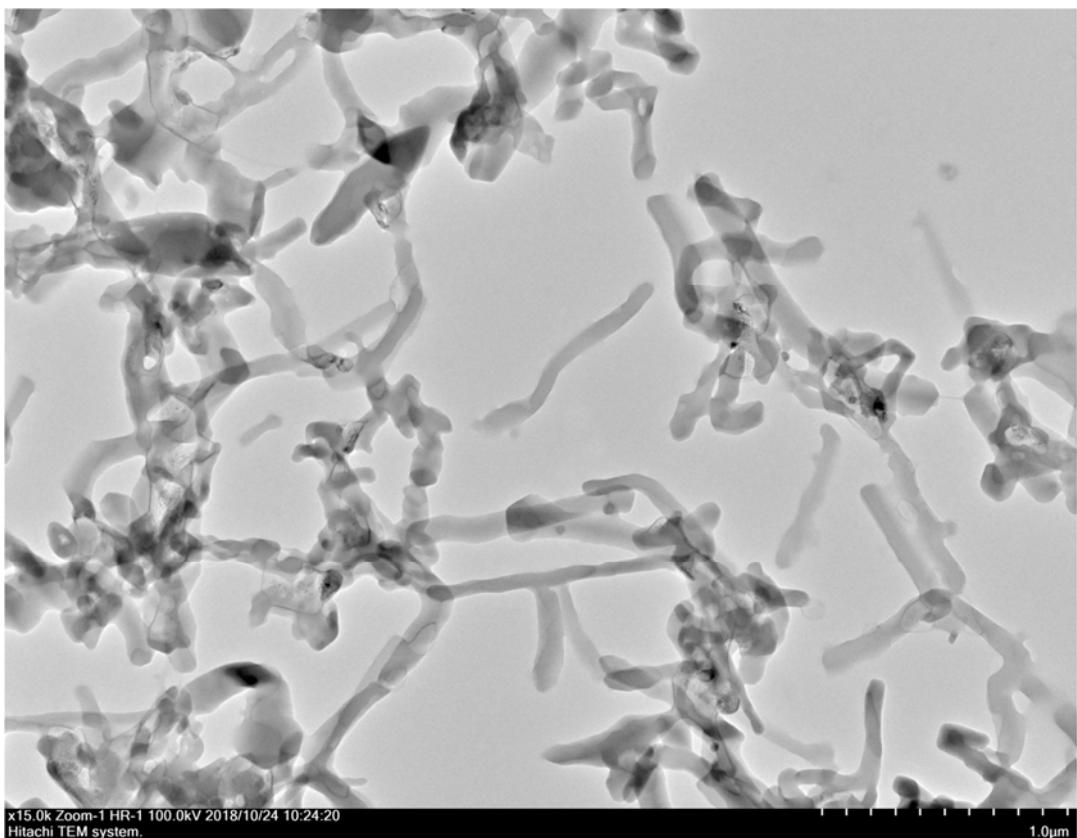
**Fig. S47.** TEM image of SLN-5-RhB after the solvent evaporation.
