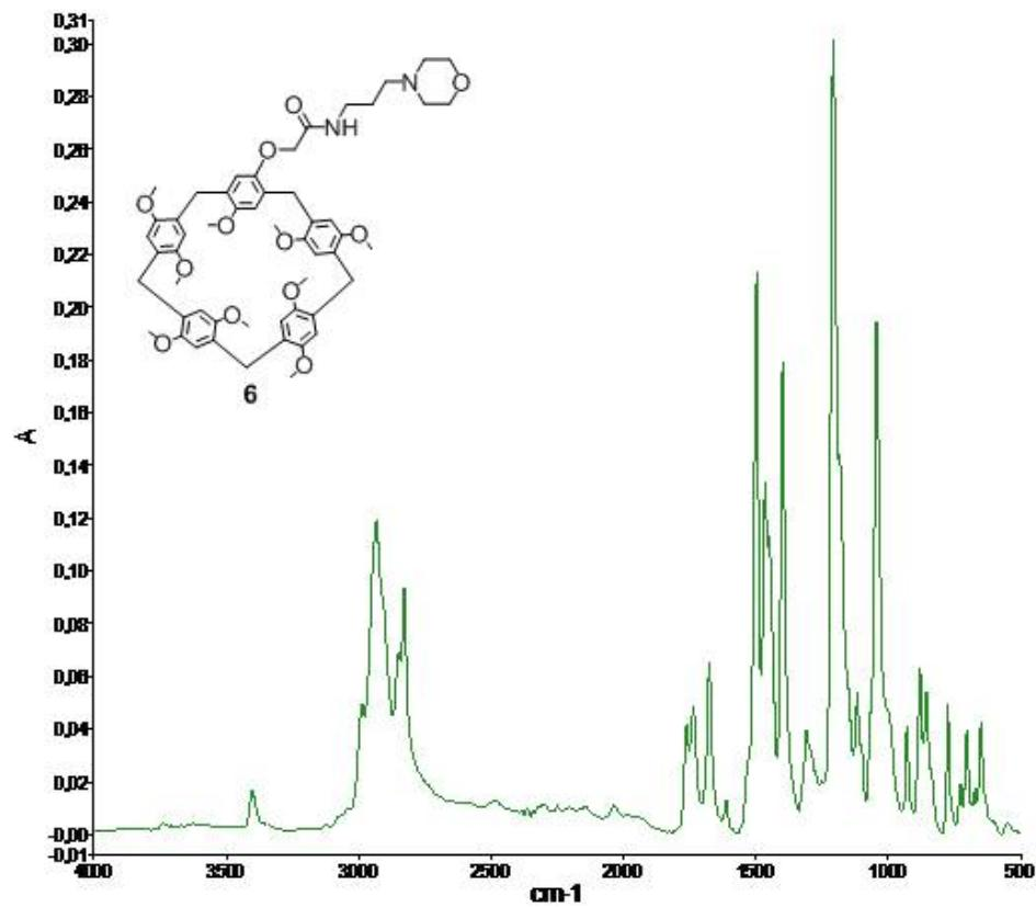
**Fig. S13.** IR spectrum of 4-N-[2-(2-aminomorpholine)propyl]acetamidoxy-8,14,18,23,26,28,31,32,35-nonamethoxypillar[5]arene (**6**).
