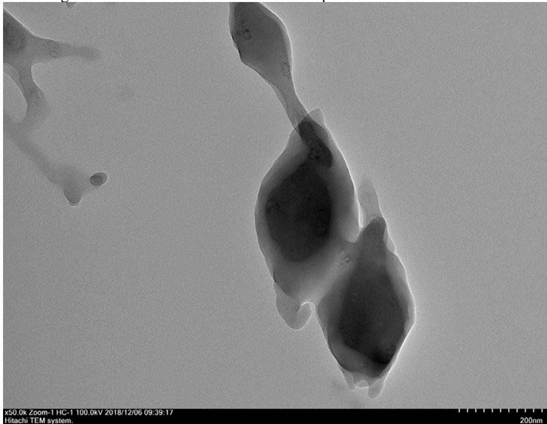
**Fig. S63.** TEM image of SLN-5-Rh6G after the solvent evaporation.
