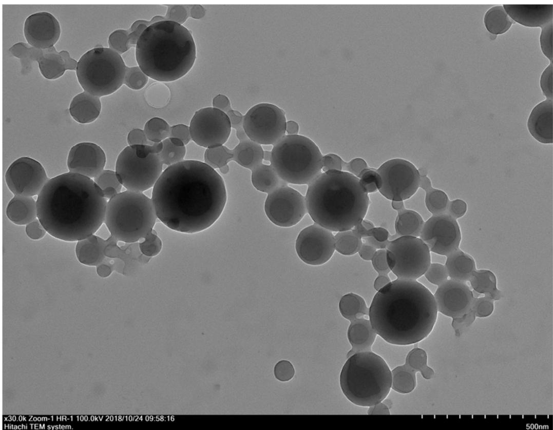
**Fig. S51.** TEM image of SLN-6-RhB after the solvent evaporation.
