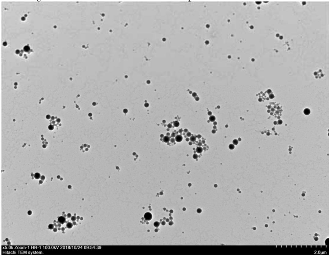
**Fig. S50.** TEM image of SLN-6-RhB after the solvent evaporation.
