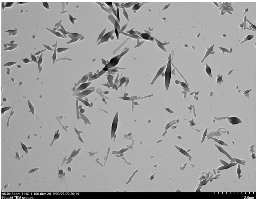
**Fig. S18.** TEM image of SLN-5 after the solvent evaporation.
