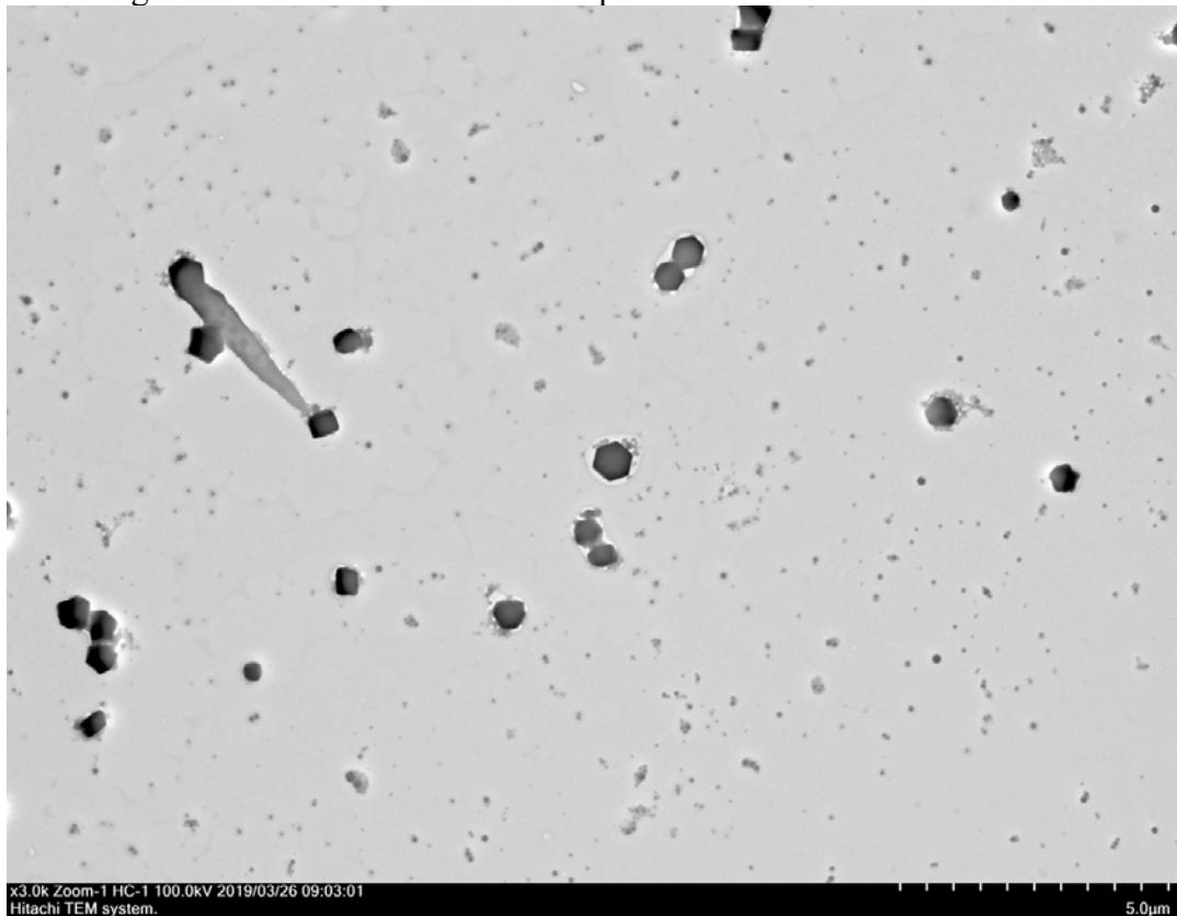
**Fig. S15.** TEM image of SLN-4 after the solvent evaporation.
