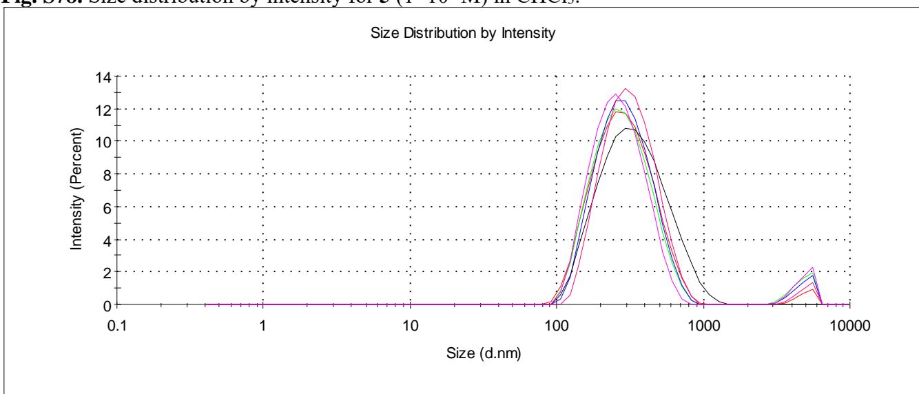
**Fig. S79.** Size distribution by intensity for **5** ( $1 \times 10^{-3}$ M) in DMSO.
