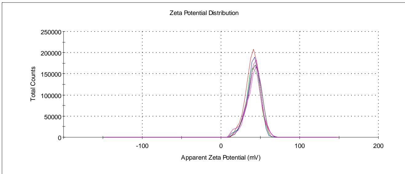
**Fig. S83.** Zeta potential distribution of the particles SLN-3 ( $3 \times 10^{-5}$ M) in water.
