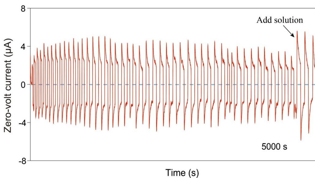
**Fig. S7.** Zero-volt current through  $Ti_3C_2T_x$  membrane within 5000 seconds when the illumination was applied to the left or right side of the membrane, showing the good stability and repeatability of ion pump device.
