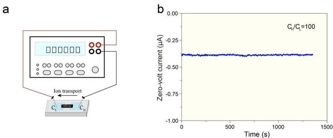
**Fig. S6.** Illustration of the appearance of ionic current. (a) Schematic of measurement. The positive (red) and negative (black) probes of Keithley 2400 were connected with Ag/AgCl electrodes that inserted into the left and right reservoirs. Ion diffusion current was measured at I-T mode when the left and right reservoirs were filled with solutions of  $C_L$  and  $C_H$ , respectively. (b) Ion diffusion current under 100-fold ( $C_H$
