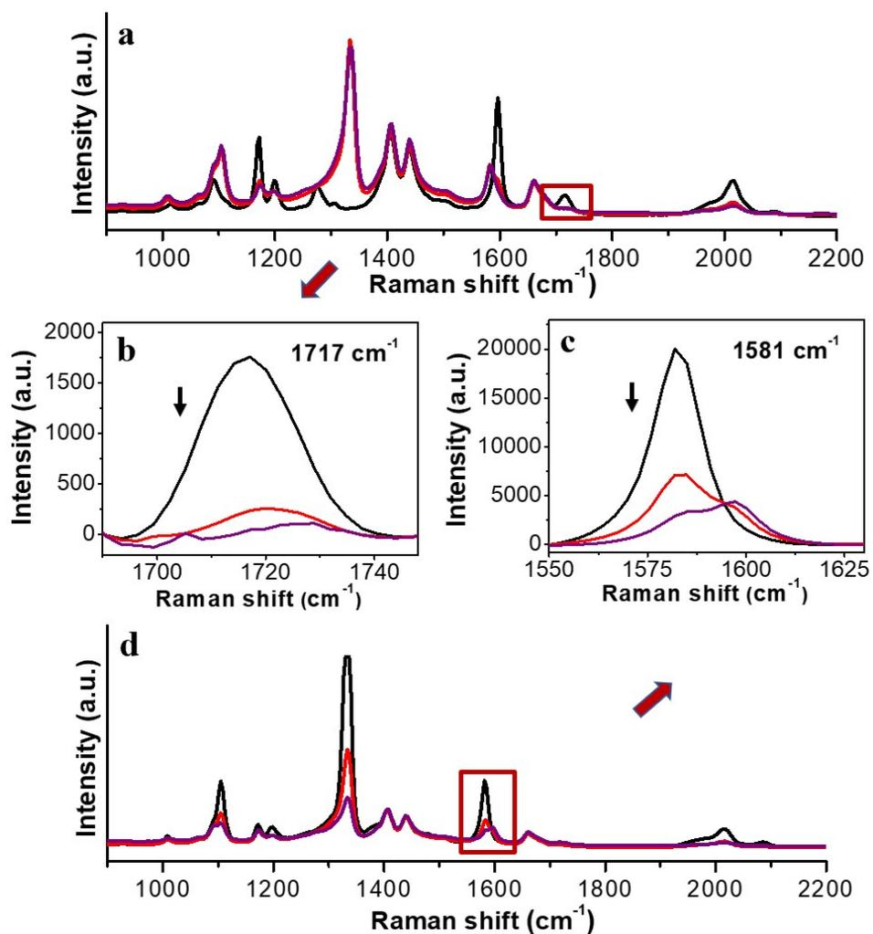
**Figure S35.** (a) Temporal evolution of the SERS intensity of 8.3  $\mu\text{M}$  5-AuNPs incubated with 8.2  $\mu\text{M}$  (red) and 82  $\mu\text{M}$  (purple) 3 in DMF. (b) Expansion of the framed region in a. (c) Expansion of the framed region in d. (d) Temporal evolution of the SERS intensity of 8.3  $\mu\text{M}$  3-AuNPs incubated with 8.2  $\mu\text{M}$  (red) and 82  $\mu\text{M}$  (purple) 5 in DMF.
