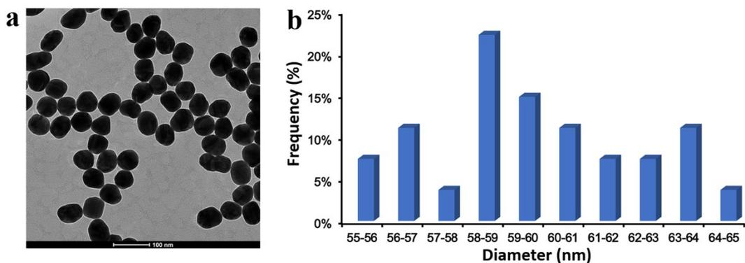
**Figure S2.** (a) TEM image of the as-synthesized 60 nm AuNPs; (b) the size distribution of the AuNPs.
