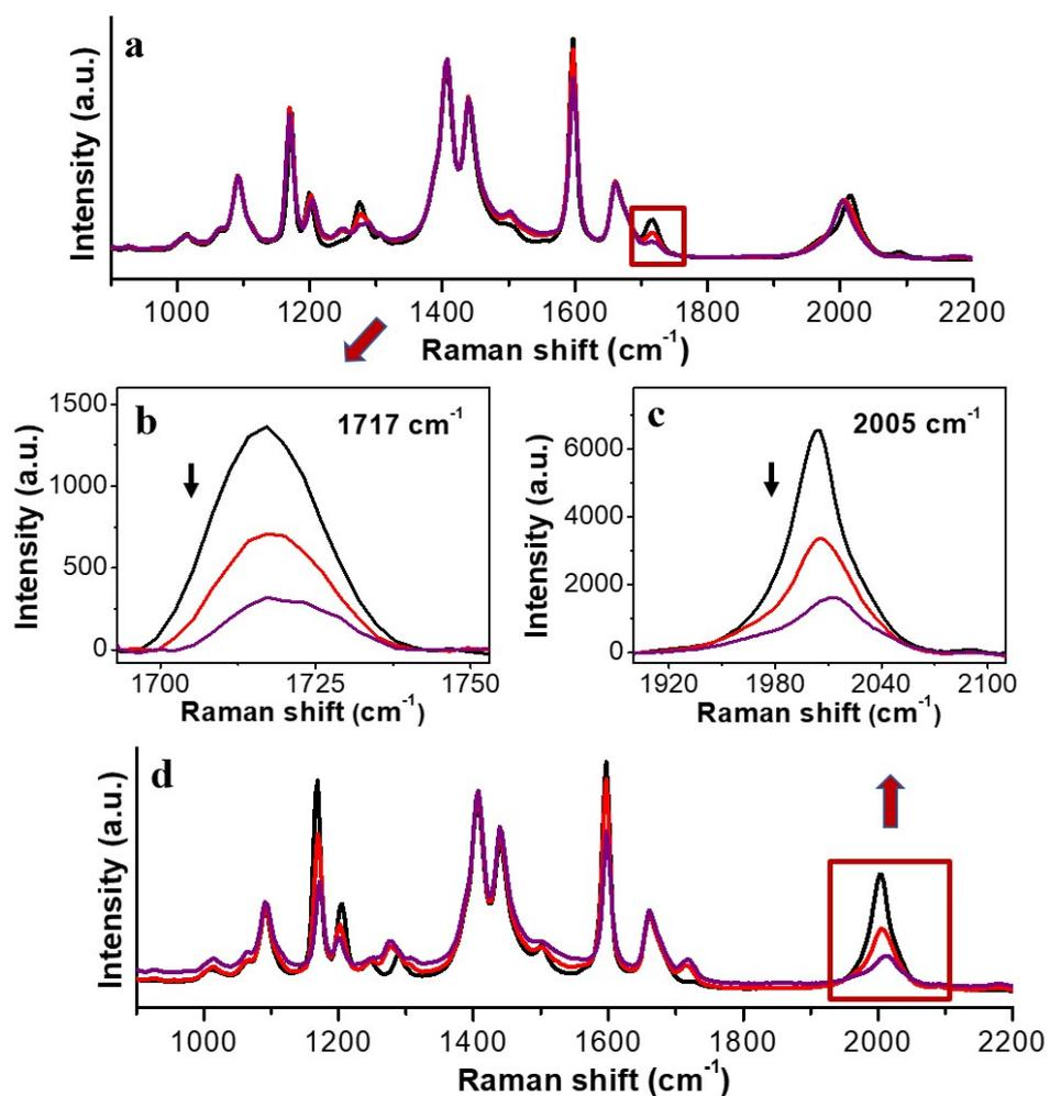
**Figure S36.** (a) Temporal evolution of the SERS intensity of 8.3  $\mu\text{M}$  5-AuNPs incubated with 8.2  $\mu\text{M}$  (red) and 82  $\mu\text{M}$  (purple) 4 in DMF. (b) Expansion of the framed region in a. (c) Expansion of the framed region in d. (d) Temporal evolution of the SERS intensity of 8.3  $\mu\text{M}$  4-AuNPs incubated with 8.2  $\mu\text{M}$  (red) and 82  $\mu\text{M}$  (purple) 5 in DMF.
