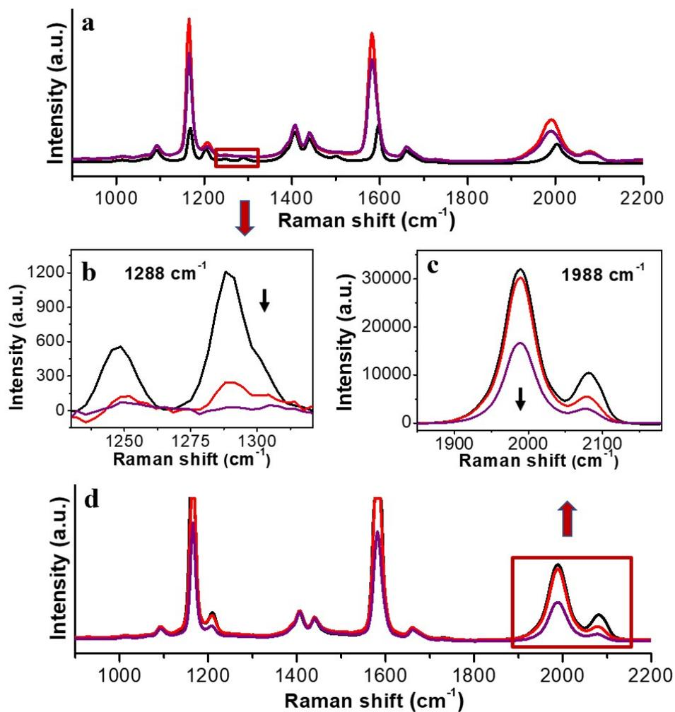
**Figure S31.** (a) Temporal evolution of the SERS intensity of  $8.3 \mu\text{M}$  4-AuNPs incubated with  $8.2 \mu\text{M}$  (red) and  $82 \mu\text{M}$  (purple) 1 in DMF. (b) Expansion of the framed region in a. (c) Expansion of the framed region in d. (d) Temporal evolution of the SERS intensity of  $8.3 \mu\text{M}$  1-AuNPs incubated with  $8.2 \mu\text{M}$  (red) and  $82 \mu\text{M}$  (purple) 4 in DMF.
