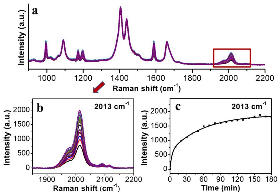
**Figure S11.** (a) Temporal evolution of the SERS intensity of citrate-AuNPs incubated with 8.3  $\mu\text{M}$  PhA under Ar atmosphere in a cuvette which was sealed in a glove box. (b) Expansion of the framed region in a. (c) Intensity traces of the peak in b.
