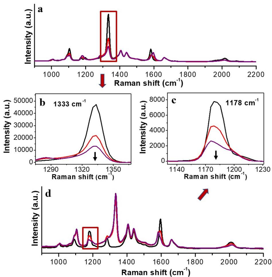
**Figure S32.** (a) Temporal evolution of the SERS intensity of 8.3  $\mu\text{M}$  3-AuNPs incubated with 8.2  $\mu\text{M}$  (red) and 82  $\mu\text{M}$  (purple) 2 in DMF. (b) Expansion of the framed region in a. (c) Expansion of the framed region in d. (b) Temporal evolution of the SERS intensity of 8.3  $\mu\text{M}$  2-AuNPs incubated with 8.2  $\mu\text{M}$  (red) and 82  $\mu\text{M}$  (purple) 3 in DMF.
