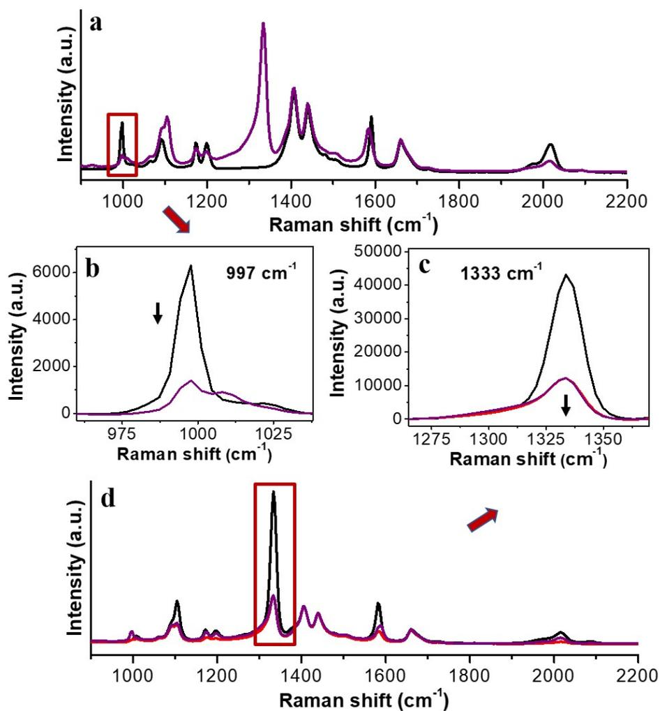
**Figure S24.** (a) Temporal evolution of the SERS intensity of 8.3  $\mu\text{M}$  PhA-AuNPs incubated with 8.2  $\mu\text{M}$  3 in DMF. (b) Expansion of the framed region in a. (c) Expansion of the framed region in d. (d) Temporal evolution of the SERS intensity of 8.3  $\mu\text{M}$  3-AuNPs incubated with 8.2  $\mu\text{M}$  (red) and 82  $\mu\text{M}$  (purple) PhA in DMF.
