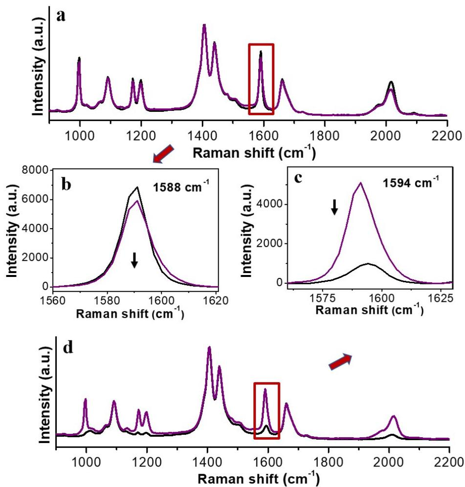
**Figure S28.** (a) Temporal evolution of the SERS intensity of 8.3 μM PhA-AuNPs incubated with 8.2 μM 7 in DMF. (b) Expansion of the framed region in a. (c) Expansion of the framed region in d. (d) Temporal evolution of the SERS intensity of 8.3 μM 7-AuNPs incubated with 8.2 μM PhA in DMF.
