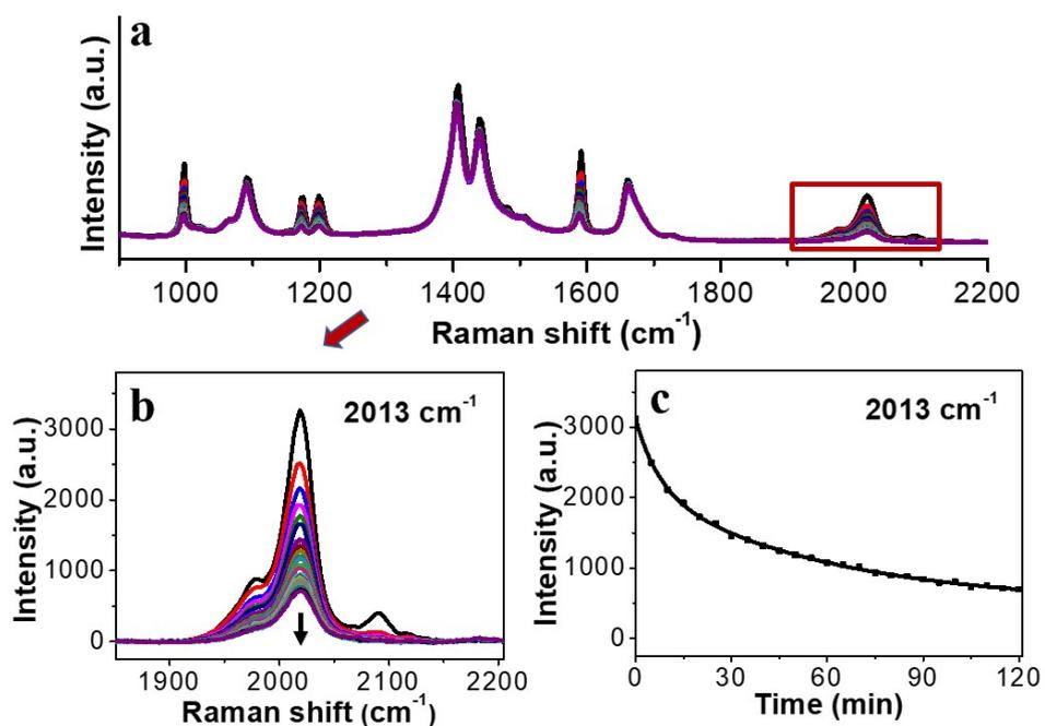
**Figure S20.** (a) Temporal evolution of the SERS intensity of 8.3  $\mu\text{M}$  PhA-AuNPs incubated with 2.5 mM PVP in DMF. (b) Expansion of the framed region in a. (c) Intensity traces of the peak in b.
