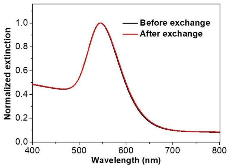
**Figure S18.** UV-vis spectra of AuNPs in DMF before and after PVP exchange PhA.
