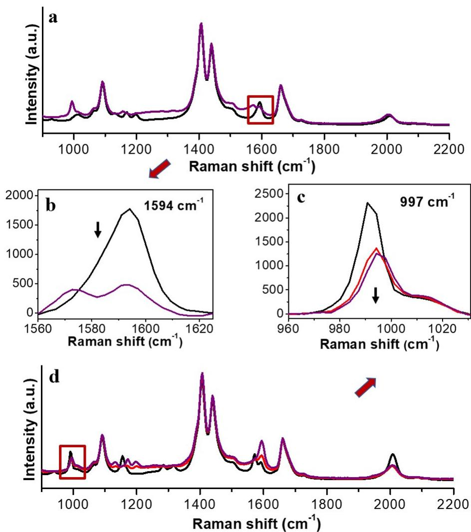
**Figure S37.** (a) Temporal evolution of the SERS intensity of 8.3  $\mu\text{M}$  7-AuNPs incubated with 8.2  $\mu\text{M}$  6 in DMF. (b) Expansion of the framed region in a. (c) Expansion of the framed region in d. (c) Temporal evolution of the SERS intensity of 8.3  $\mu\text{M}$  6-AuNPs incubated with 8.2  $\mu\text{M}$  (red) and 82  $\mu\text{M}$  (purple) 7 in DMF.
