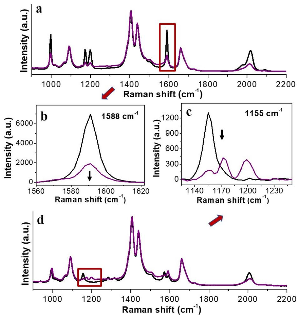
**Figure S27.** (a) Temporal evolution of the SERS intensity of 8.3  $\mu\text{M}$  PhA-AuNPs incubated with 8.2  $\mu\text{M}$  6 in DMF. (b) Expansion of the framed region in a. (c) Expansion of the framed region in d. (d) Temporal evolution of the SERS intensity of 8.3  $\mu\text{M}$  6-AuNPs incubated with 8.2  $\mu\text{M}$  PhA in DMF.
