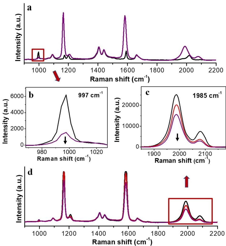
**Figure S22.** (a) Temporal evolution of the SERS intensity of 8.3  $\mu\text{M}$  PhA-AuNPs incubated with 8.2  $\mu\text{M}$  1 in DMF. (b) Expansion of the framed region in a. (c) Expansion of the framed region in d. (d) Temporal evolution of the SERS intensity of 8.3  $\mu\text{M}$  1-AuNPs incubated with 8.2  $\mu\text{M}$  (red) and 82  $\mu\text{M}$  (purple) PhA in DMF.
