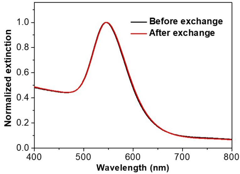
Figure S15. UV-vis spectra of AuNPs in DMF before and after PhA exchange 2-NT.
