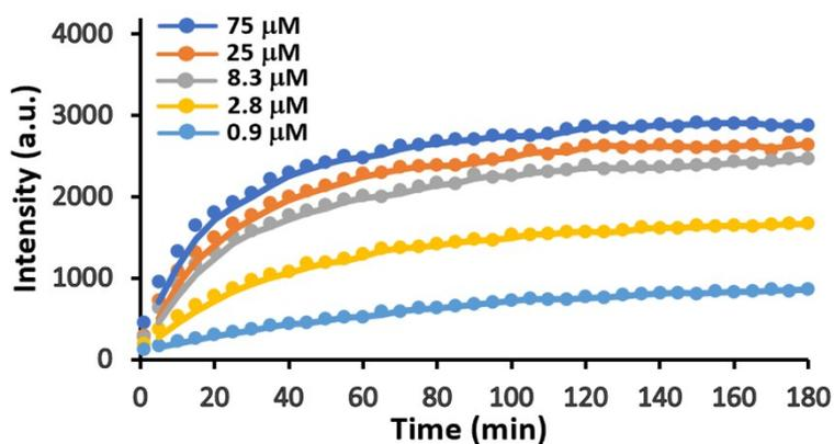
**Figure S9.** Normalized traces of SERS intensity at  $2013\text{ cm}^{-1}$  during the incubation of citrate-AuNPs with PhA in DMF for the different concentration samples.
