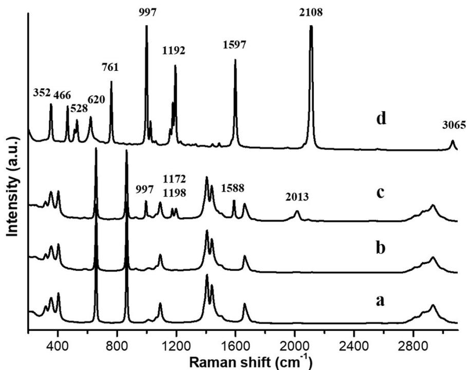
**Figure S6** (a) Raman spectra of pure DMF. (b) SERS intensity of 60 nm citrate-AuNPs in DMF. (c) SERS intensity of 8.3  $\mu$ M PhA-AuNPs in DMF. (d) Raman spectra of pure PhA.
