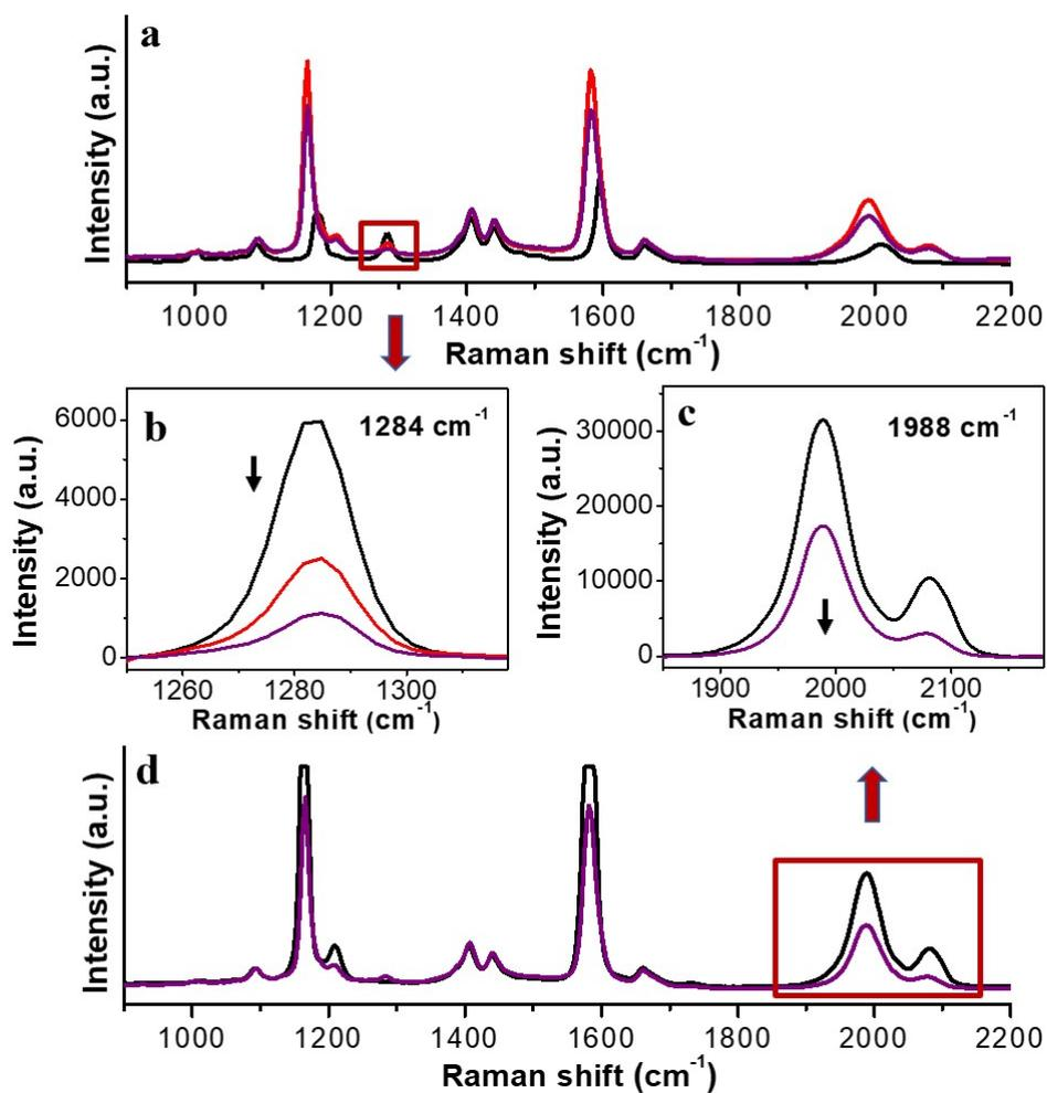
**Figure S29.** (a) Temporal evolution of the SERS intensity of 8.3  $\mu\text{M}$  2-AuNPs incubated with 8.2  $\mu\text{M}$  (red) and 82  $\mu\text{M}$  (purple) 1 in DMF. (b) Expansion of the framed region in a. (c) Expansion of the framed region in d. (d) Temporal evolution of the SERS intensity of 8.3  $\mu\text{M}$  1-AuNPs incubated with 82  $\mu\text{M}$  2 in DMF.
