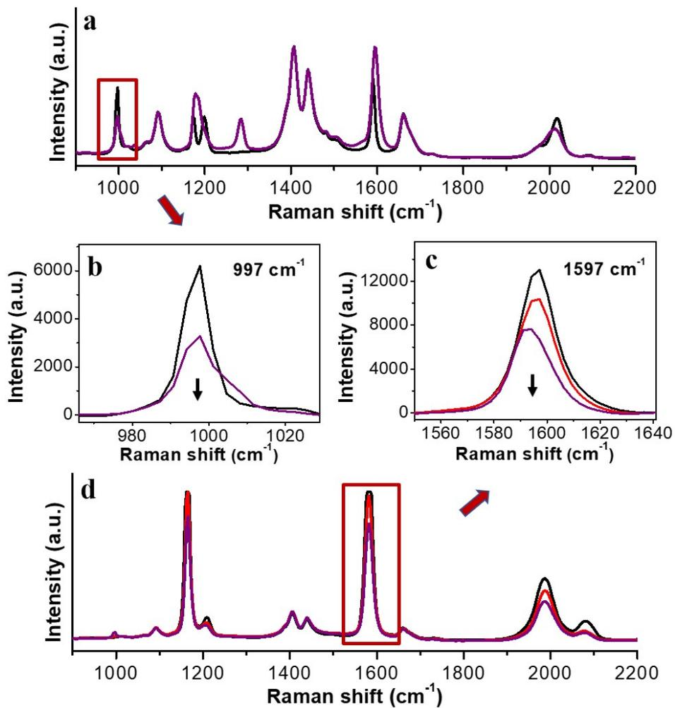
**Figure S23.** (a) Temporal evolution of the SERS intensity of 8.3  $\mu\text{M}$  PhA-AuNPs incubated with 8.2  $\mu\text{M}$  2 in DMF. (b) Expansion of the framed region in a. (c) Expansion of the framed region in d. (d) Temporal evolution of the SERS intensity of 8.3  $\mu\text{M}$  2-AuNPs incubated with 8.2  $\mu\text{M}$  (red) and 82  $\mu\text{M}$  (purple) PhA in DMF.
