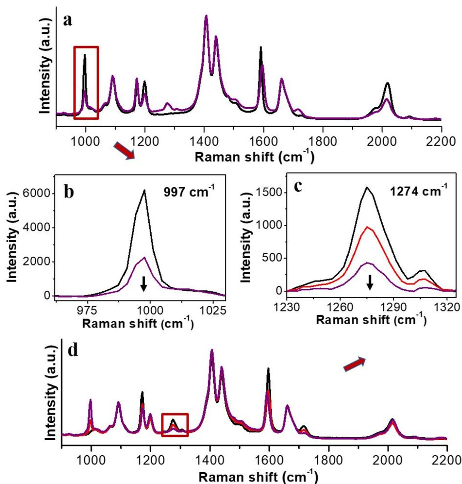
**Figure S26.** (a) Temporal evolution of the SERS intensity of 8.3  $\mu\text{M}$  PhA-AuNPs incubated with 8.2  $\mu\text{M}$  5 in DMF. (b) Expansion of the framed region in a. (c) Expansion of the framed region in d. (d) Temporal evolution of the SERS intensity of 8.3  $\mu\text{M}$  5-AuNPs incubated with 8.2  $\mu\text{M}$  (red) and 82  $\mu\text{M}$  (purple) PhA in DMF.
