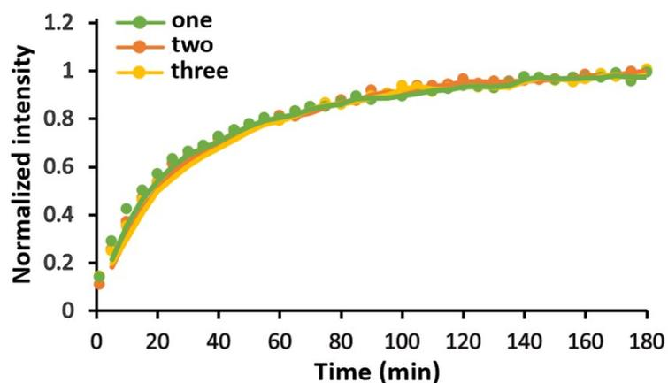
**Figure S8.** Normalized traces of SERS intensity at  $2013\text{ cm}^{-1}$  during the incubation of citrate-AuNPs with  $8.3\text{ }\mu\text{M}$  PhA in DMF for the same three samples.
