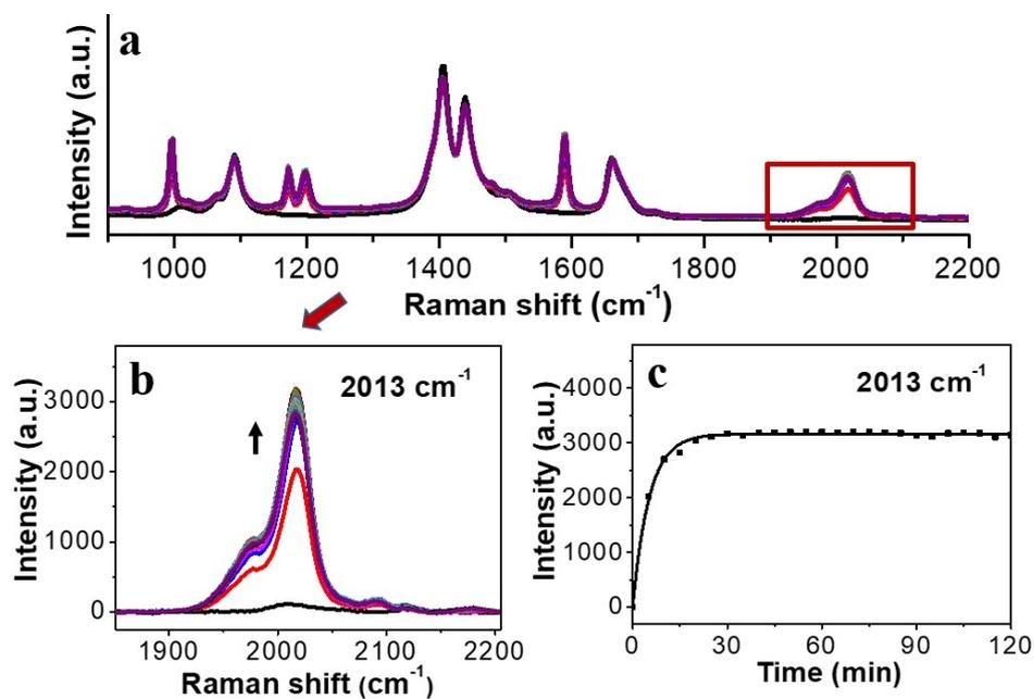
**Figure S21.** (a) Temporal evolution of the SERS intensity of 8.3  $\mu\text{M}$  PVP-AuNPs incubated with 8.2  $\mu\text{M}$  PhA in DMF. (b) Expansion of the framed region in a. (c) Intensity traces of the peak in b.
