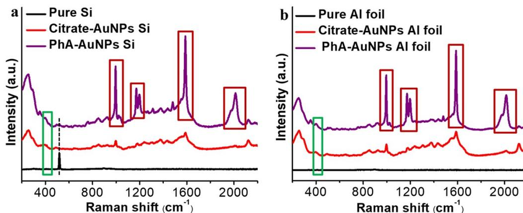
**Figure S13.** (a) Raman spectra of pure Si (black); SERS intensity of 60 nm citrate-AuNPs (red), PhA-AuNPs (purple) on Si. (b) Raman spectra of pure Al foil (black); SERS intensity of 60 nm citrate-AuNPs (red), PhA-AuNPs on Al foil.
