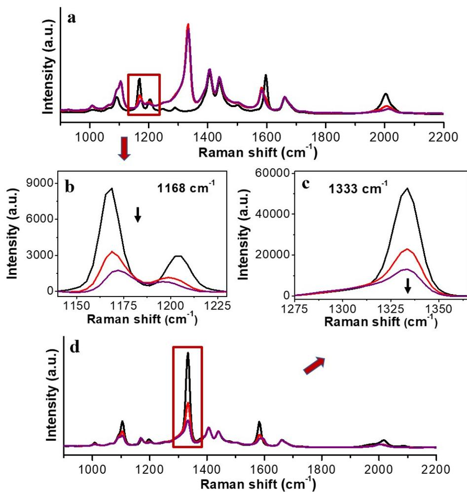
**Figure S34.** (a) Temporal evolution of the SERS intensity of 8.3  $\mu\text{M}$  4-AuNPs incubated with 8.2  $\mu\text{M}$  (red) and 82  $\mu\text{M}$  (purple) 3 in DMF. (b) Expansion of the framed region in a. (c) Expansion of the framed region in d. (d) Temporal evolution of the SERS intensity of 8.3  $\mu\text{M}$  3-AuNPs incubated with 8.2  $\mu\text{M}$  (red) and 82  $\mu\text{M}$  (purple) 4 in DMF.
