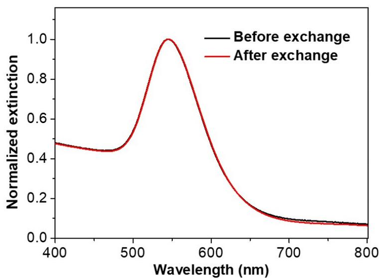
**Figure S19.** UV-vis spectra of AuNPs in DMF before and after PhA exchange PVP.
