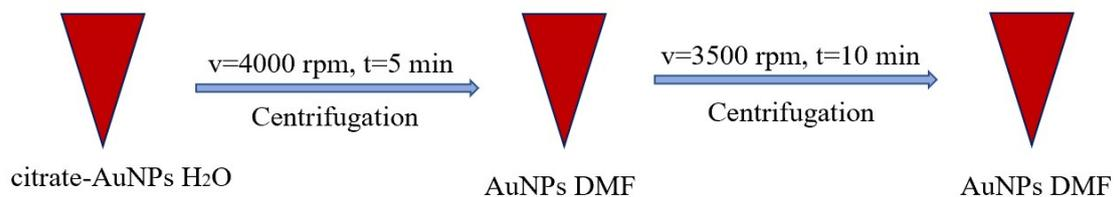
**Figure S4.** Schematics illustrating the phase transfer of 60 nm citrate-AuNPs from water to DMF.
