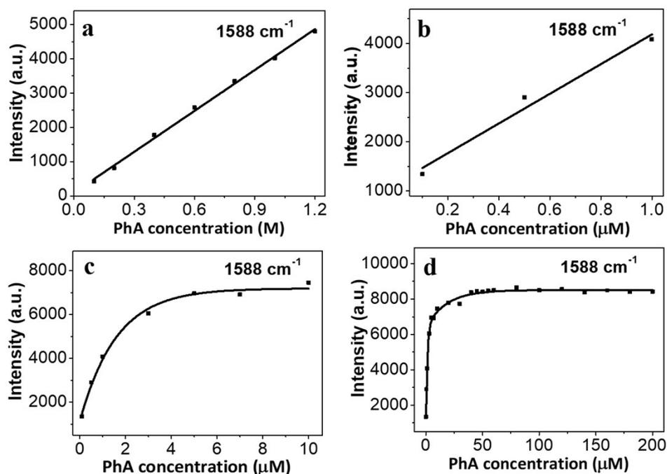
**Figure S5.** (a) Plot and linear fit of Raman intensity vs PhA concentration in DMF (0~1.2 M) for 1588  $\text{cm}^{-1}$  Raman peak. SERS intensity of (b) 0.1~1  $\mu\text{M}$ , (c) 0.1~10  $\mu\text{M}$ , (d) 0.1~200  $\mu\text{M}$  PhA-AuNPs in DMF.
