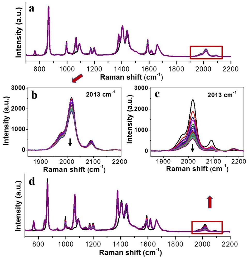
Figure S16. (a) Temporal evolution of the SERS intensity of 8.3  $\mu\text{M}$  PhA-AuNPs incubated with 8.2  $\mu\text{M}$  2-NT in DMF at room temperature. (b) Expansion of the framed region in a. (c)
