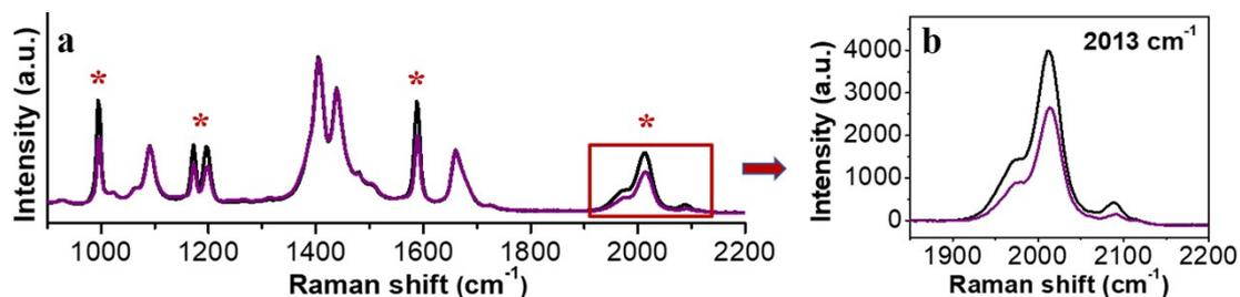
**Figure S10.** (a) SERS intensity of citrate-AuNPs after 3 h incubation with  $8.3\text{ }\mu\text{M}$  PhA ligand without (black) and with (purple) Ar gas bubbling. (b) Expansion of the framed region in a.
