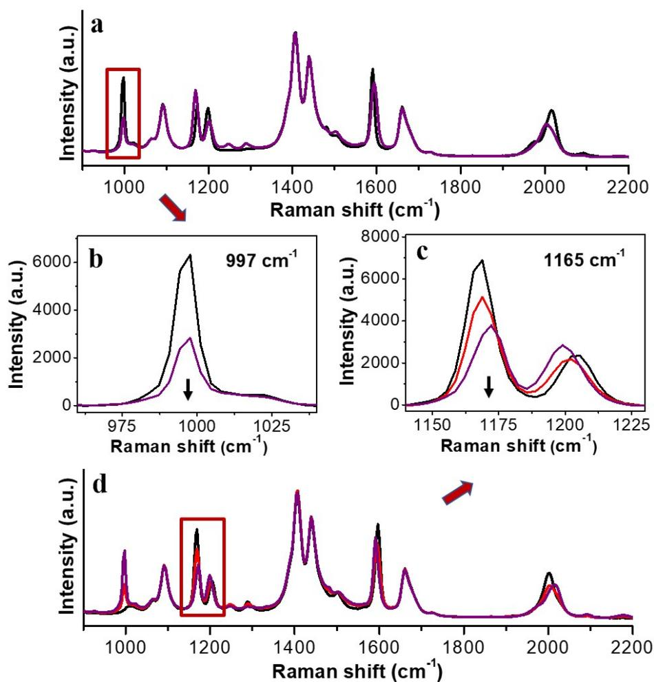
**Figure S25.** (a) Temporal evolution of the SERS intensity of 8.3 μM PhA-AuNPs incubated with 8.2 μM 4 in DMF. (b) Expansion of the framed region in a. (c) Expansion of the framed region in d. (d) Temporal evolution of the SERS intensity of 8.3 μM 4-AuNPs incubated with 8.2 μM (red) and 82 μM (purple) PhA in DMF.
