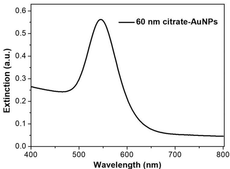
**Figure S3.** UV-vis spectra of 60 nm citrate-AuNPs.
