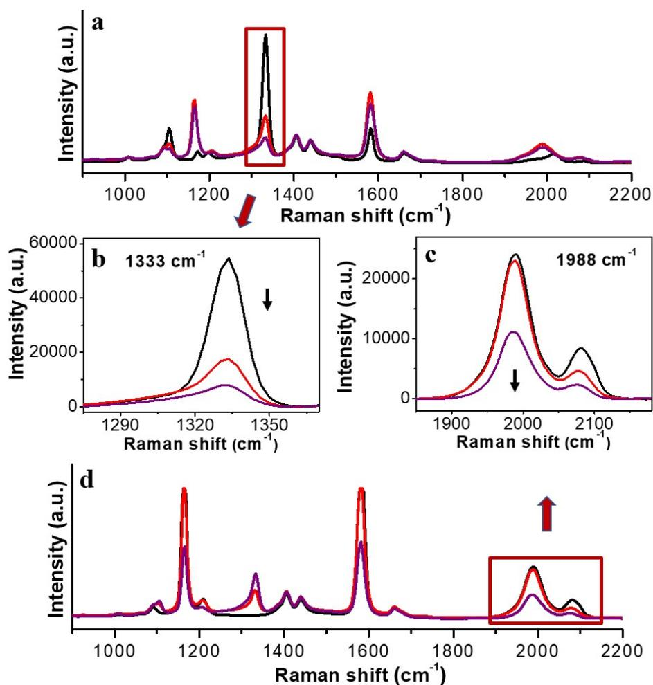
**Figure S30.** (a) Temporal evolution of the SERS intensity of 8.3  $\mu\text{M}$  3-AuNPs incubated with 8.2  $\mu\text{M}$  (red) and 82  $\mu\text{M}$  (purple) 1 in DMF. (b) Expansion of the framed region in a. (c) Expansion of the framed region in d. (d) Temporal evolution of the SERS intensity of 8.3  $\mu\text{M}$  1-AuNPs incubated with 8.2  $\mu\text{M}$  (red) and 82  $\mu\text{M}$  (purple) 3 in DMF.
