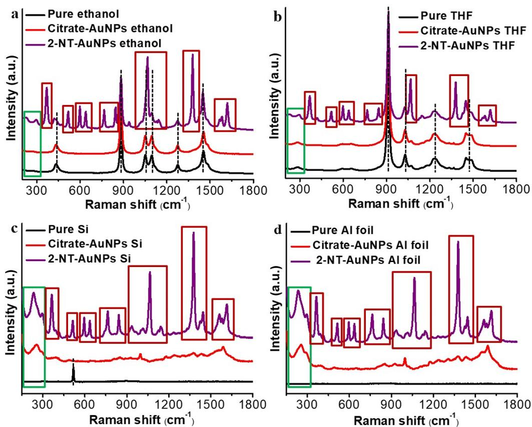
**Figure S38.** (a) Raman spectra of pure ethanol (black); SERS intensity of 60 nm citrate-AuNPs (red), 2-NT-AuNPs (purple) in ethanol. (b) Raman spectra of pure THF (black); SERS intensity of 60 nm citrate-AuNPs (red), 2-NT-AuNPs (purple) in THF. (c) Raman spectra of pure Si (black); SERS intensity of 60 nm citrate-AuNPs (red), 2-NT-AuNPs (purple) on Si. (d) Raman spectra of pure Al foil (black); SERS intensity of 60 nm citrate-AuNPs (red), 2-NT-AuNPs (purple) on Al foil.
