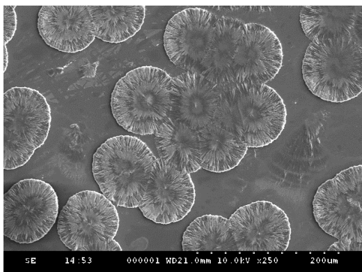
Figure 14c: - FESEM image for self-assembly of aspartic acid in 0.1 M NH 3 n aqueous medium
