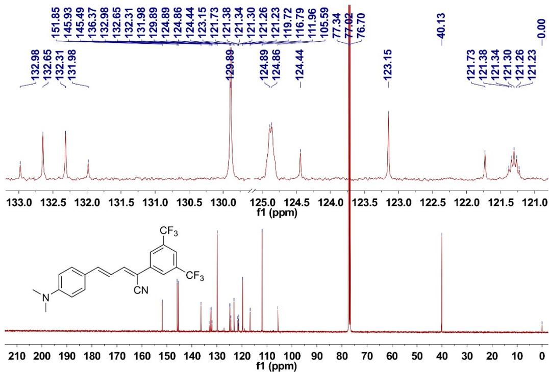
Fig. S2. <sup>13</sup>C NMR spectrum of ABCXF in CDCl<sub>3</sub>
