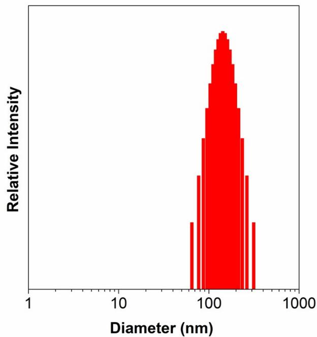
**Fig. S7.** Dynamic light scattering data of ABCXF in water containing 1% of THF. Hydrated diameter: 142 nm.
