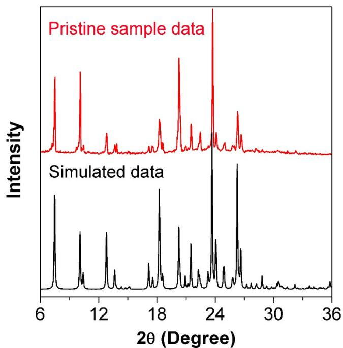
**Fig. S8.** XRD pattern of the pristine sample and simulated XRD pattern of ABCXF.
