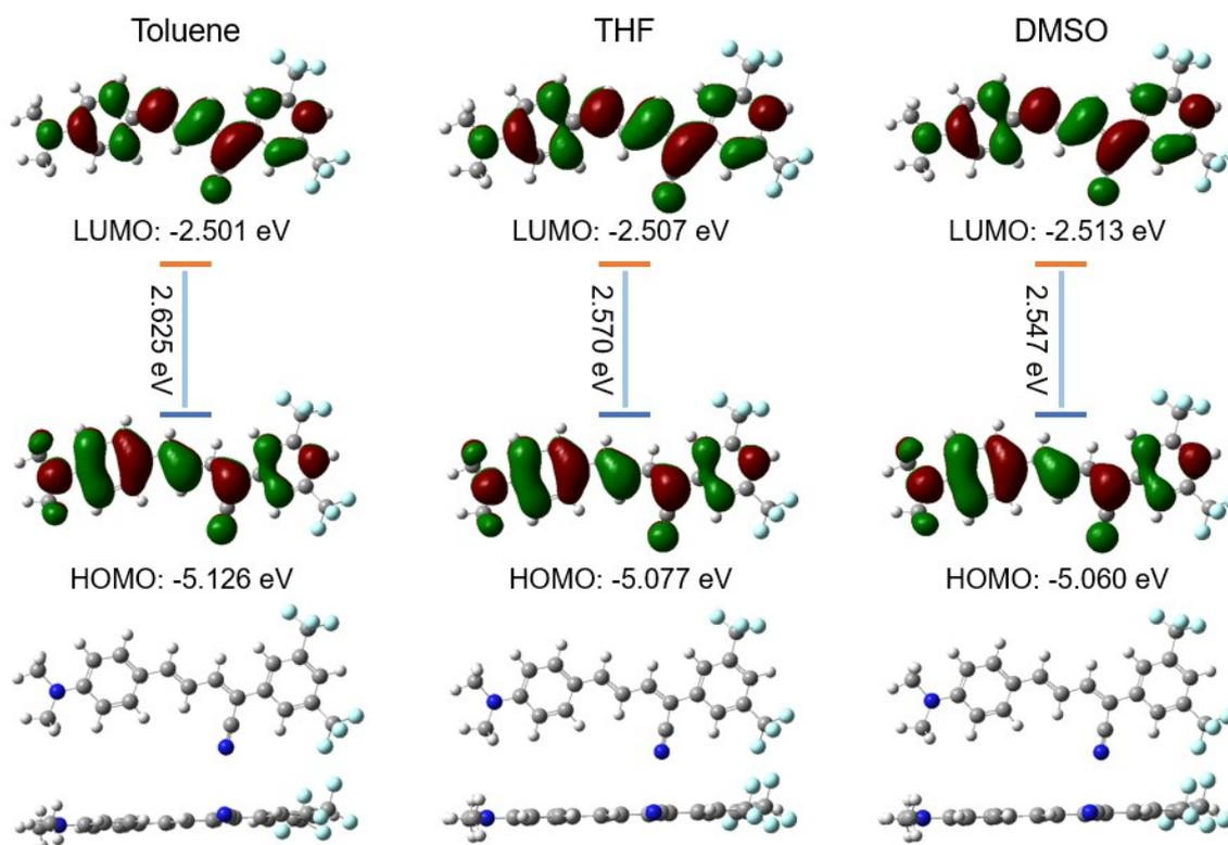
**Fig. S12.** Frontier molecular orbitals of ABCXF in toluene, THF and DMSO, at excited state calculated by B3LYP/6-31G(d, p) method, Gaussian 09 program.
