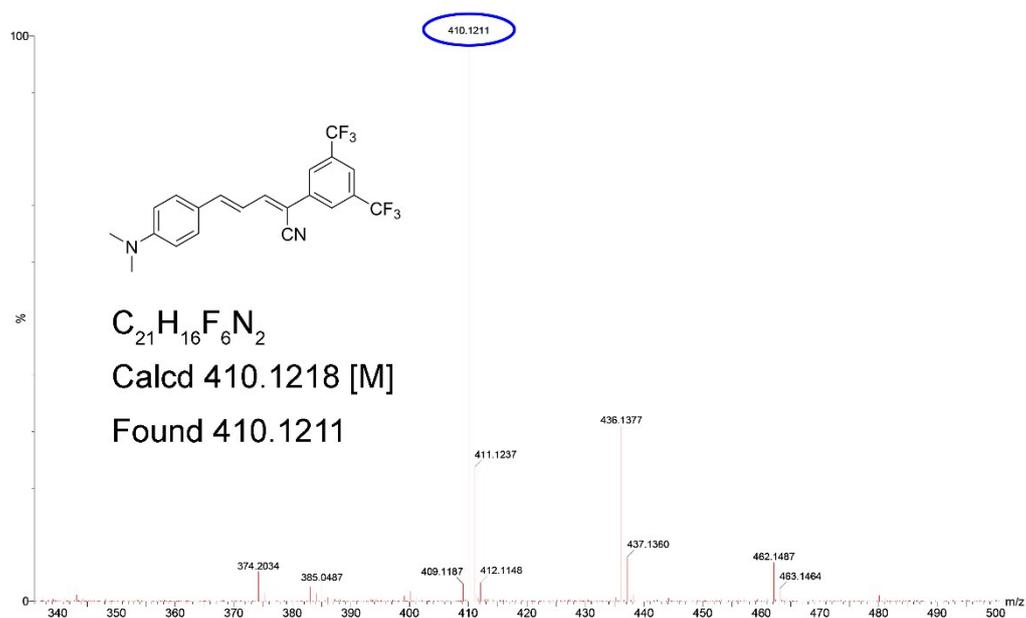
**Fig. S4.** High-resolution mass spectrum of ABCXF.
