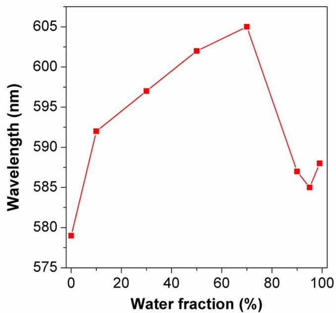
**Fig. S6.** The plot of the maximum emission wavelength versus the composition of THF/water mixture containing ABCXF (10 μM).
