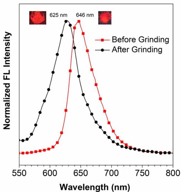
**Fig. S11.** Change in the emission spectrum of ABCXF after grinding process.
