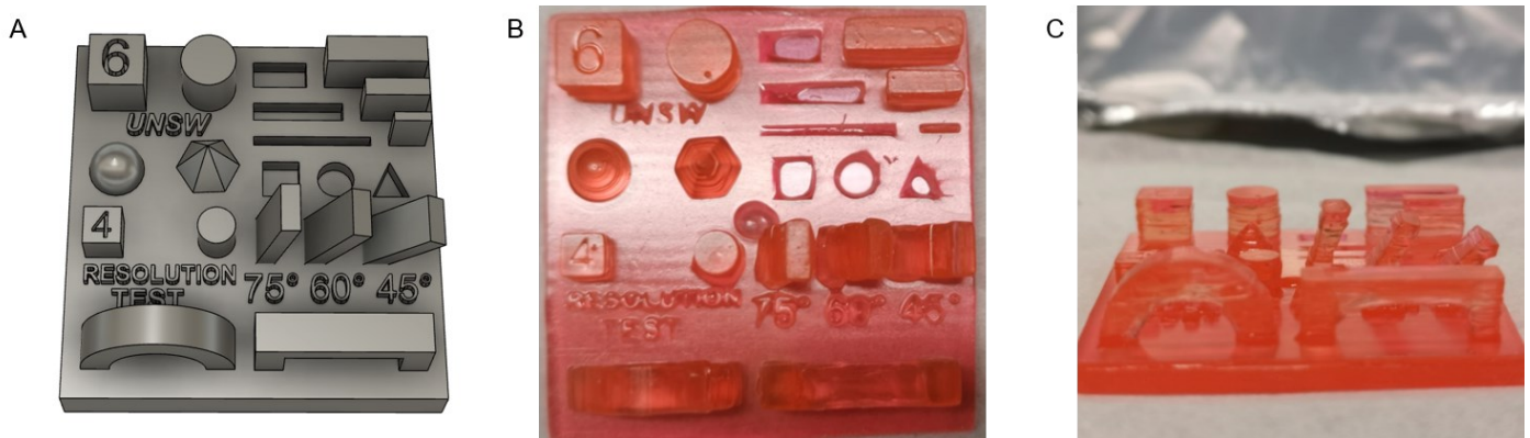
Figure S6. Resolution study of developed photocurable resin. A) Designed model for resolution test. B) Top view of printed resolution test model. C) Side view of printed resolution test model. Note: The model was printed under 0.32\text{ mWcm}^{-2} green light ( \lambda_{\text{max}} = 530\text{ nm} ) with t_c of 30s and layer thickness ( T_{la} ) of 20\text{ }\mu\text{m} . using [\text{F1}]:[\text{EA}]:[\text{PEGDA}]:[\text{EB}]:[\text{TEtOHA}] = 5:860:2004:0.1:40 .
