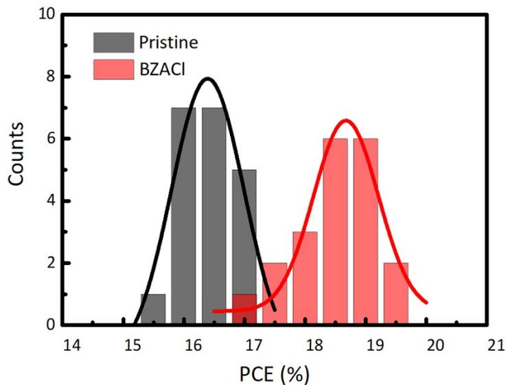
**Figure S2.** Statistical PCE distribution histogram of 20 devices based on pristine and BZACl doped perovskite, respectively.
