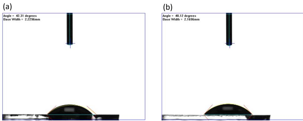
**Figure S1.** The contact angle measurements performed on the (a) pristine and (b) BZACl doped perovskite substrate. The contact angles are  $42.31^\circ$  and  $48.12^\circ$  in (a) and (b), respectively.
