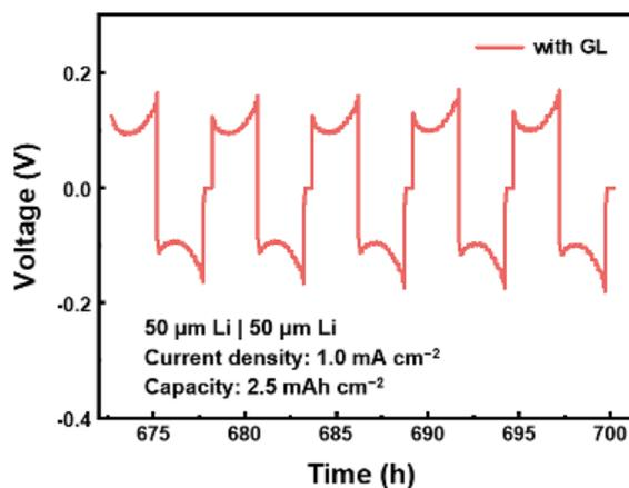
**Figure S1.** The partial enlarged voltage–time curves of the Li | Li symmetric cell with GL additives at  $1.0 \text{ mA cm}^{-2}$  and a capacity of  $2.5 \text{ mAh cm}^{-2}$ .
