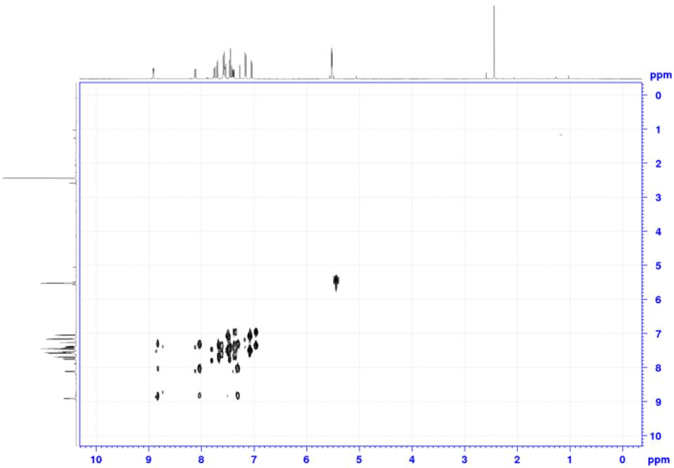
**Figure S84:** COSY NMR spectrum of compound **2h** in  $\text{CDCl}_3$  at 298 K.
