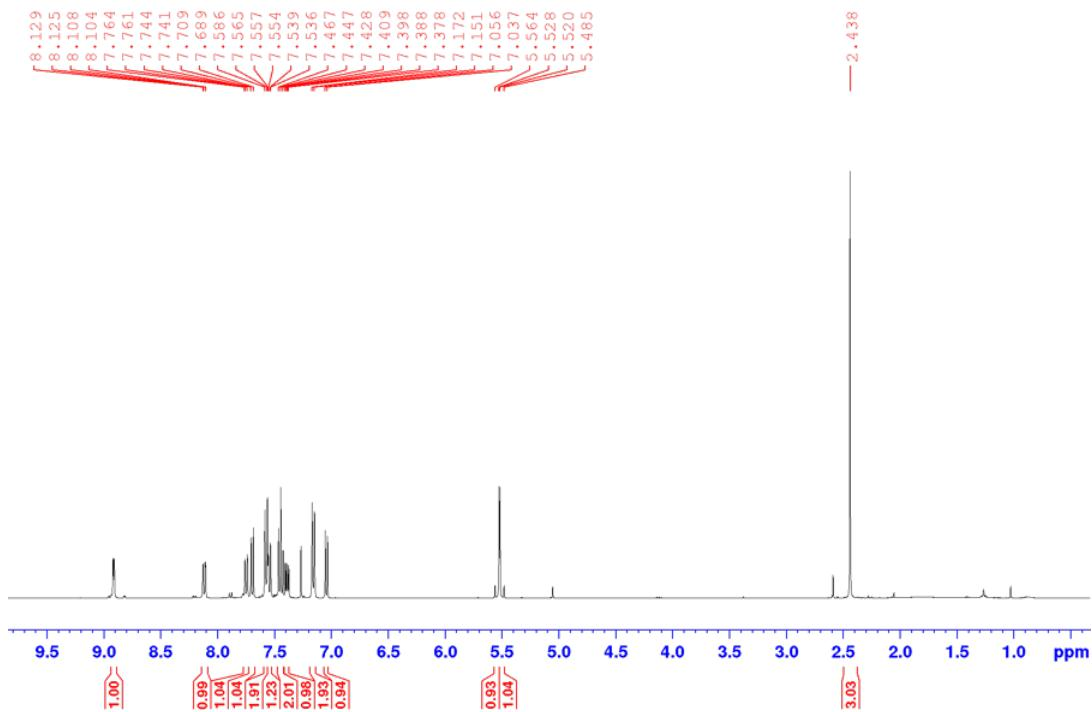
**Figure S82:**  $^1\text{H}$  NMR spectrum of compound **2h** in  $\text{CDCl}_3$  at 298 K.
