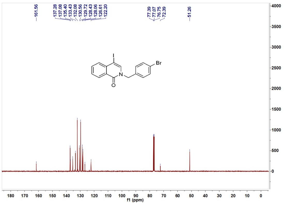
The <sup>1</sup>H NMR and <sup>13</sup>C NMR spectra of 5k
