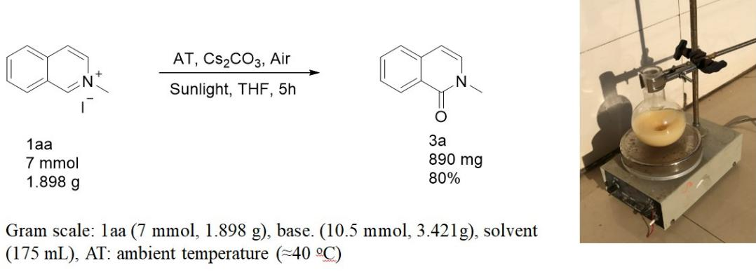
**Figure S1.** Apparatus and scalable visible light induced synthesis of isoquinolone 3a
