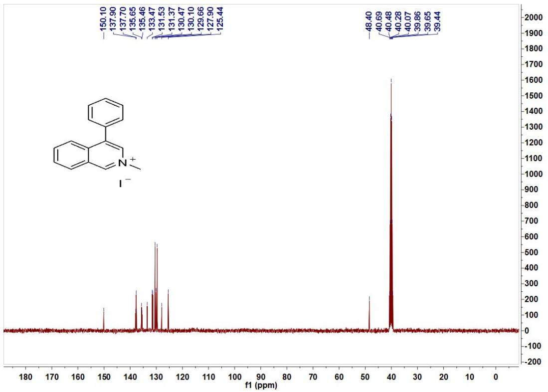
The  $^1\text{H}$  NMR and  $^{13}\text{C}$  NMR spectra of **1r**
