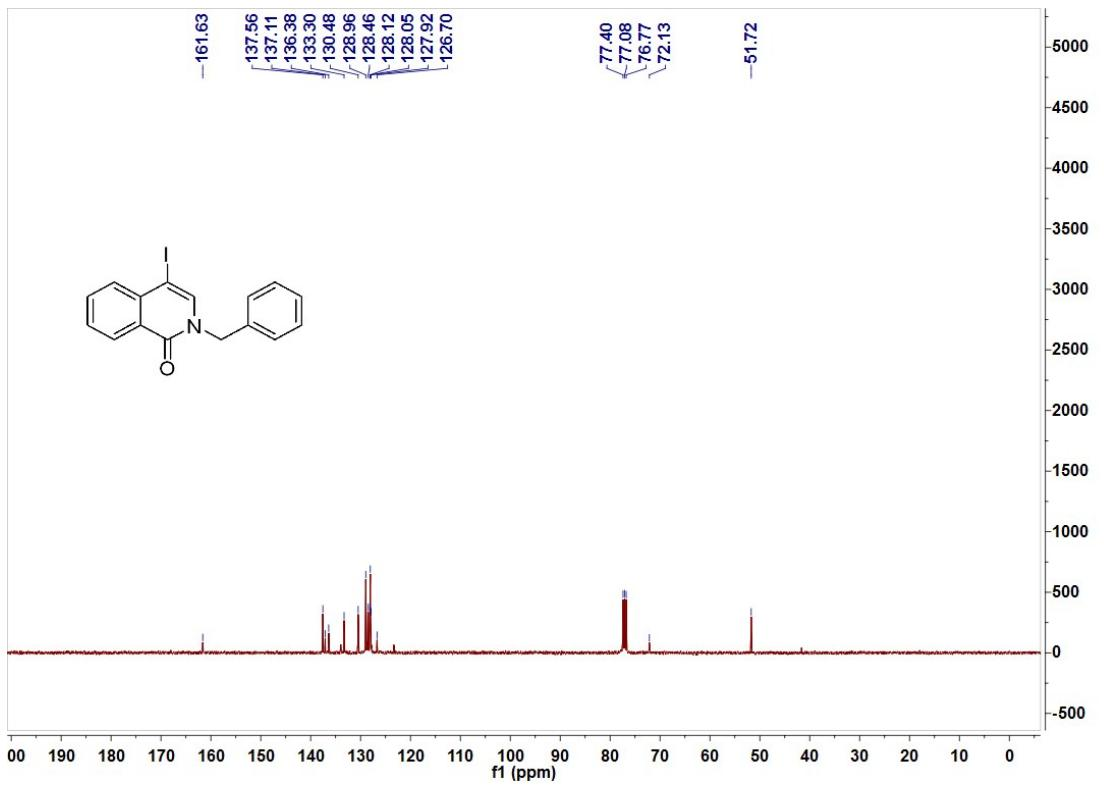
The <sup>1</sup>H NMR and <sup>13</sup>C NMR spectra of 5f
