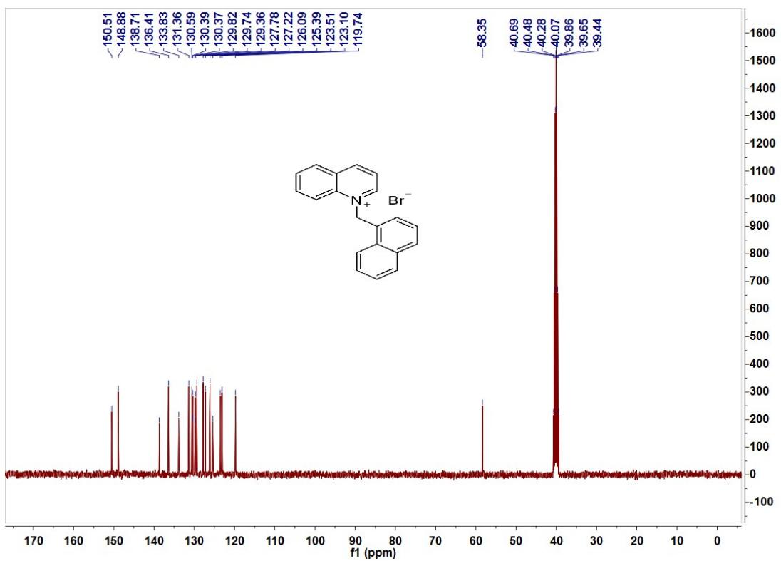
The <sup>1</sup>H NMR and <sup>13</sup>C NMR spectra of 2l
