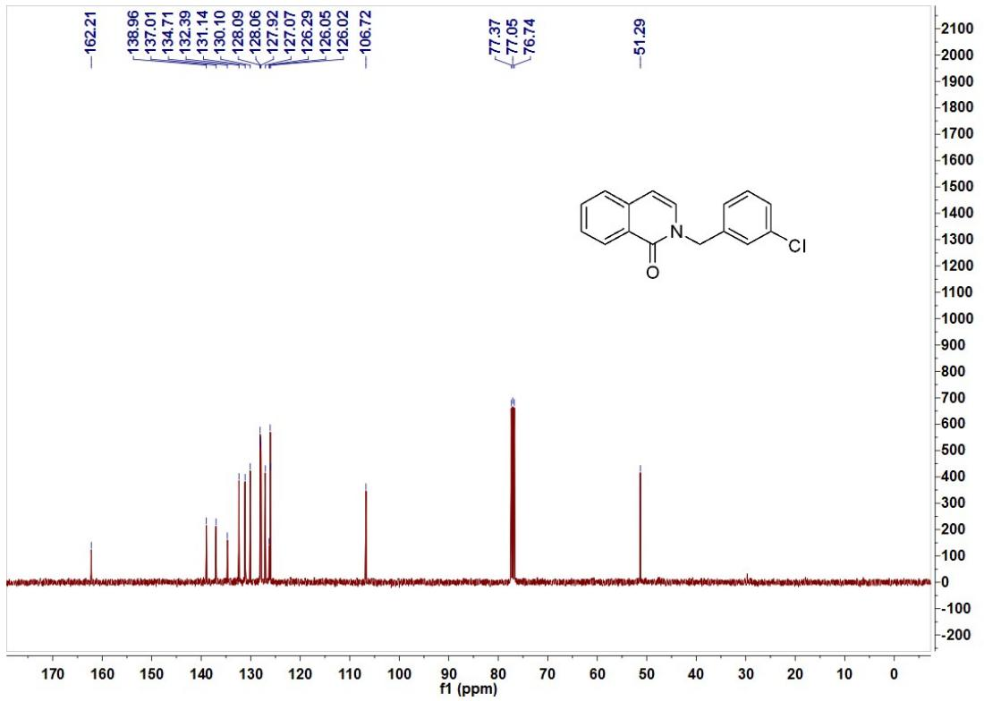
The <sup>1</sup>H NMR and <sup>13</sup>C NMR spectra of 3l
