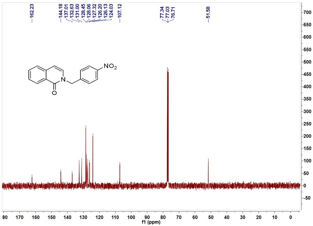
The  $^1\text{H}$  NMR and  $^{13}\text{C}$  NMR spectra of **3i**
