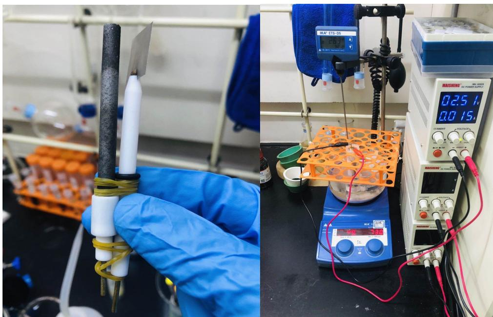
Figure S1 electrodes and batch reactor
