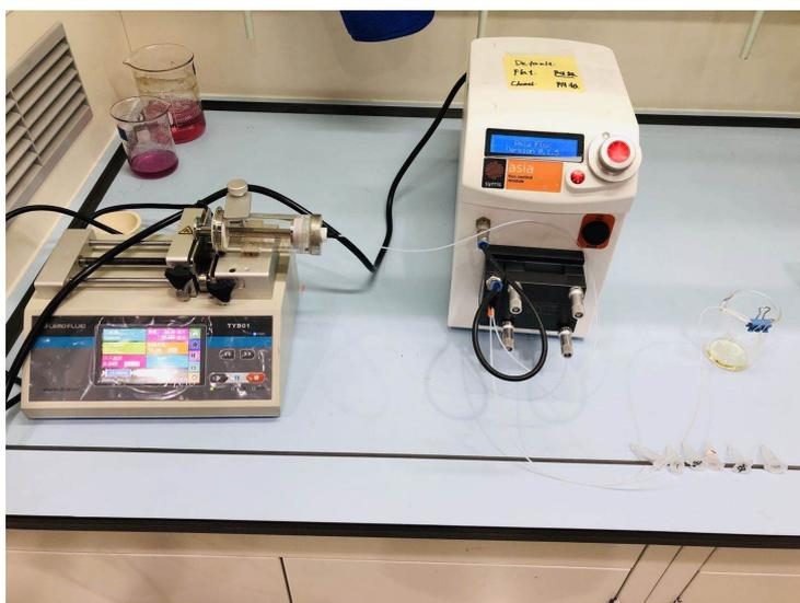
Figure S2 Electrochemistry continuous flow system
