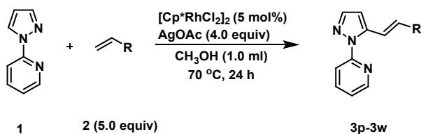
In a 50 mL sealed tube, the mixture of **1** (0.20 mmol), **2** (1.0 mmol), AgOAc (133.5 mg, 0.8 mmol),  $[\text{Cp}^*\text{RhCl}_2]_2$  (6.2 mg, 0.01 mmol), were dissolved in anhydrous MeOH (1.0 mL). The reaction mixture was heated to 70 °C for 24 h. When the reaction was finished, the mixture was cooled to room temperature and the solvents were removed under reduced pressure. The residue was purified by column chromatography on silica gel (EtOAc/Petroleum ether) to give the products **3p-3w**.
