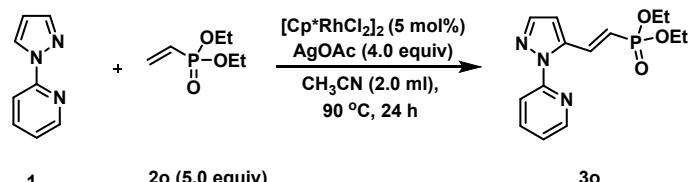
In a 50 mL sealed tube, the mixture of **1** (0.20 mmol), **2o** (1.0 mmol), AgOAc (133.5 mg, 0.8 mmol), [Cp<sup>\*</sup>RhCl<sub>2</sub>]<sub>2</sub> (6.2 mg, 0.01 mmol), were dissolved in anhydrous MeCN (2.0 mL). The reaction mixture was heated to 90 °C for 24 h. When the reaction was finished, the
