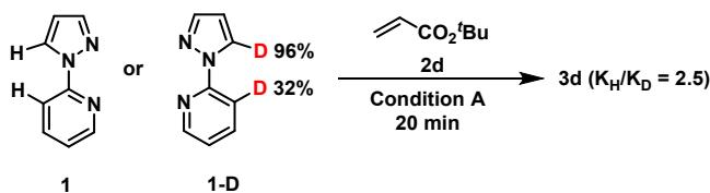
In a 50 mL sealed tube, the mixture of **1** or **1-D** (0.20 mmol), **2d** (1.0 mmol), AgOAc (133.5 mg, 0.8 mmol),  $[\text{Cp}^*\text{RhCl}_2]_2$  (6.2 mg, 0.01 mmol), were dissolved in anhydrous CH<sub>3</sub>CN (2.0 mL). The reaction mixture was heated to 90 °C for 20 min. The solvent was removed in vacuum and <sup>1</sup>H NMR was taken using 0.20 mmol 1,3,5-trimethoxybenzene as the internal standard.
