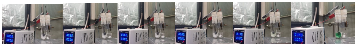
Figure S16. Intensification of colour in the anodic chamber as a function of increasing constant potential.
