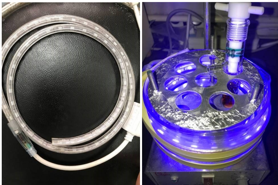
Figure S1. 8 W LEDs strip and reaction setup
