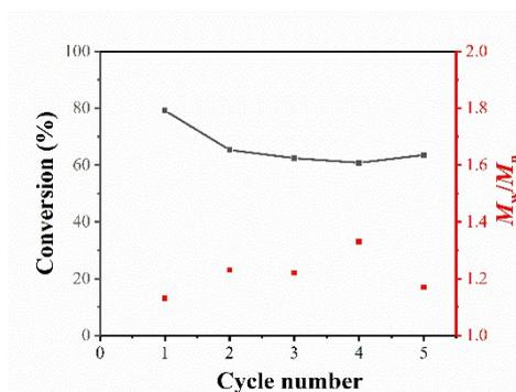
**Figure S8.** The average polymerization yields and polydispersity index (PDI) of PMMA after each PET-RAFT polymerization.
