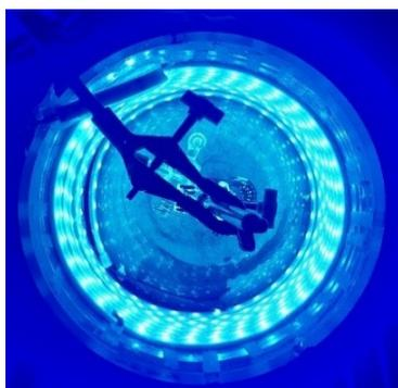
**Figure S4.** Representative photograph composed of reaction vial surrounded by the blue LEDs (A small fan was used to continuously blow air into the reaction system to fully dissipate the heat to maintain the reaction temperature at room temperature.).
