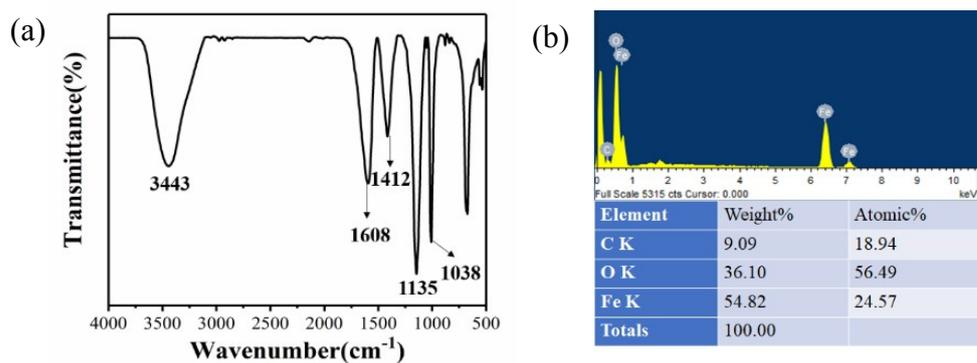
**Figure S3.** FTIR spectra and the EDS analysis of superparamagnetic  $\gamma$ -Fe<sub>2</sub>O<sub>3</sub>@CDs nanoparticles.
