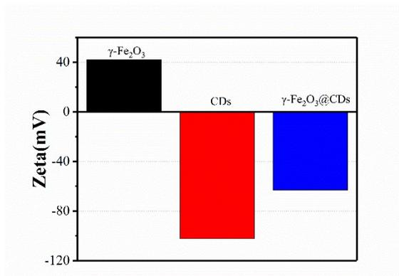
**Figure S2.**  $\zeta$  Potential of  $\gamma$ -Fe<sub>2</sub>O<sub>3</sub>, CDs and  $\gamma$ -Fe<sub>2</sub>O<sub>3</sub>@CDs nanoparticles, respectively.
