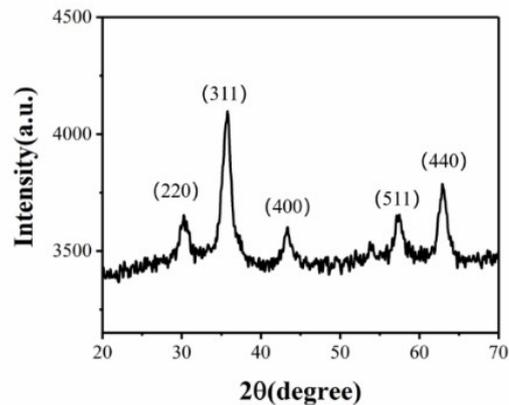
**Figure S1.** The XRD patterns of superparamagnetic  $\gamma$ -Fe<sub>2</sub>O<sub>3</sub> nanoparticles.
