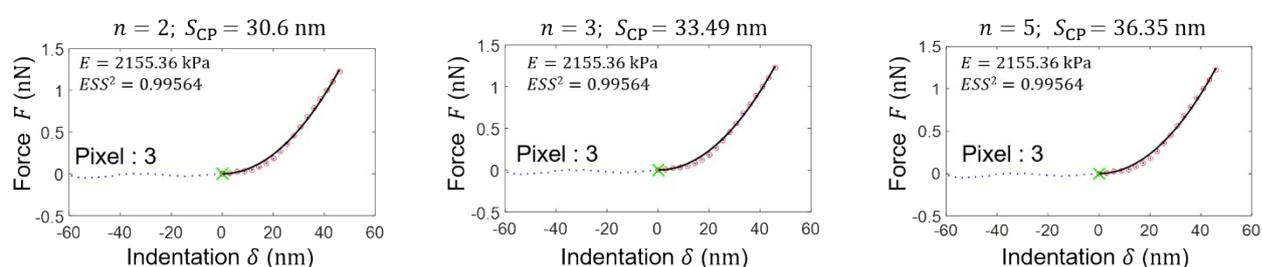
Fig. S1 Illustration of the impact of  $\sigma$  (indicated) on Young modulus derived here from Sneddon model with becc correction (given in force *versus* indentation representation). The quantity  $F_c$  corresponds to the value of the force defined by  $F_c = F + n\sigma$  with here  $n = 2, 3$  and  $5$  from the left to the right panel.
