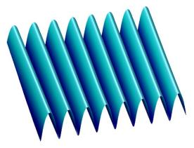
**Figure S1**. Imprinted PDMS wrinkles using the wrinkled PDMS surface as the template.
