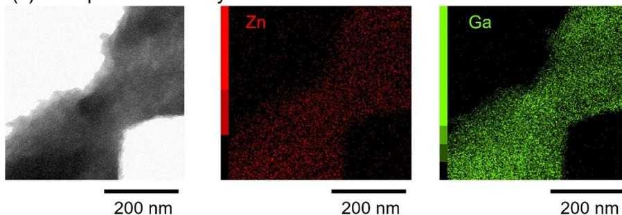
**Figure S1 (a) FE-TEM image of precursory wet gel obtained from an aqueous solution of  $\text{Zn}(\text{NO}_3)_2 \cdot 6\text{H}_2\text{O}$  and  $\text{Ga}(\text{NO}_3)_3 \cdot n\text{H}_2\text{O}$  under a highly supersaturated condition induced by epoxide-mediated alkalization. Enlarged views and EDS mappings of Zn and Ga of (b) Layered Double hydroxide and (c) Amorphous Metal Hydroxide as shown in Fig. S1(a).**
