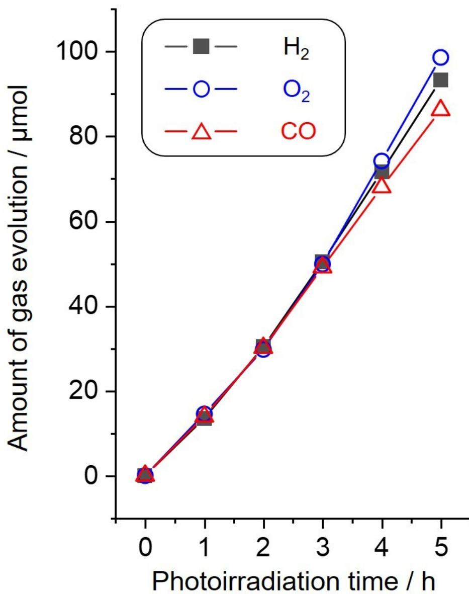
**Figure S7** Time course of gas evolutions for photocatalytic conversion of CO<sub>2</sub> with H<sub>2</sub>O over bare AMH-derived ZnGa<sub>2</sub>O<sub>4</sub>-700.
