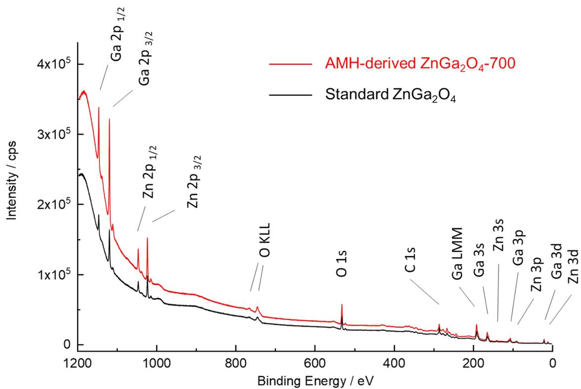
**Figure S5 Wide scan XPS spectra of AMH-derived ZnGa<sub>2</sub>O<sub>4</sub>-700 (red line) and standard ZnGa<sub>2</sub>O<sub>4</sub> (black line).**
