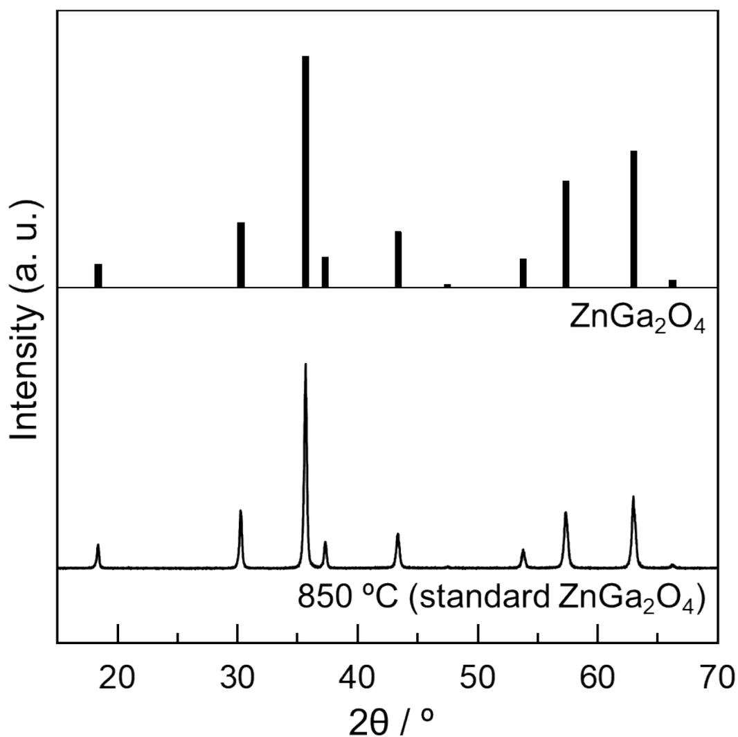
**Figure S4** PXR D patterns of ZnGa<sub>2</sub>O<sub>4</sub> prepared from a mixture of ZnO and Ga<sub>2</sub>O<sub>3</sub> powders by calcination at 850 °C. ZnGa<sub>2</sub>O<sub>4</sub> obtained as a single phase was named as “standard ZnGa<sub>2</sub>O<sub>4</sub>”. Crystallite size and BET specific surface area of standard ZnGa<sub>2</sub>O<sub>4</sub> are 29 nm and 1.3 m<sup>2</sup> g<sup>-1</sup>, respectively.
