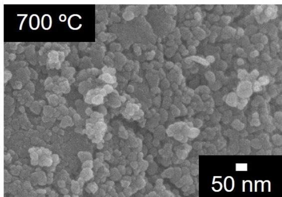
**Figure S3 SEM images of AMH-derived  $\text{ZnGa}_2\text{O}_4$  catalysts.**
