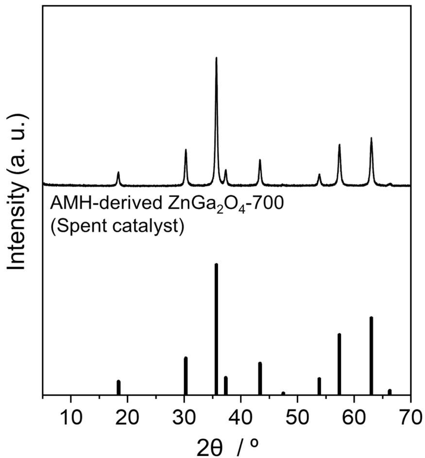
**Figure S8** XRD pattern of AMH-derived ZnGa<sub>2</sub>O<sub>4</sub>-700 after the photocatalytic CO<sub>2</sub> reduction in water.
