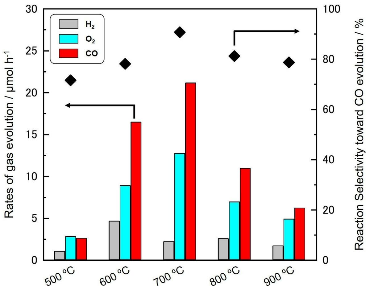
**Figure S6** Rates of H<sub>2</sub> (grey), O<sub>2</sub> (sky blue), and CO (red) evolution and reaction selectivity toward CO evolution (◆) over Ag-loaded AMH-derived ZnGa<sub>2</sub>O<sub>4</sub> prepared by calcination at various temperatures for 12 h; the loading amount of Ag co-catalyst: 1.0wt%.
